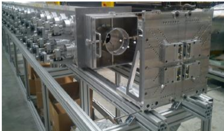
Figure 9. Aluminium full scale RFQ model to validate tuning procedures
