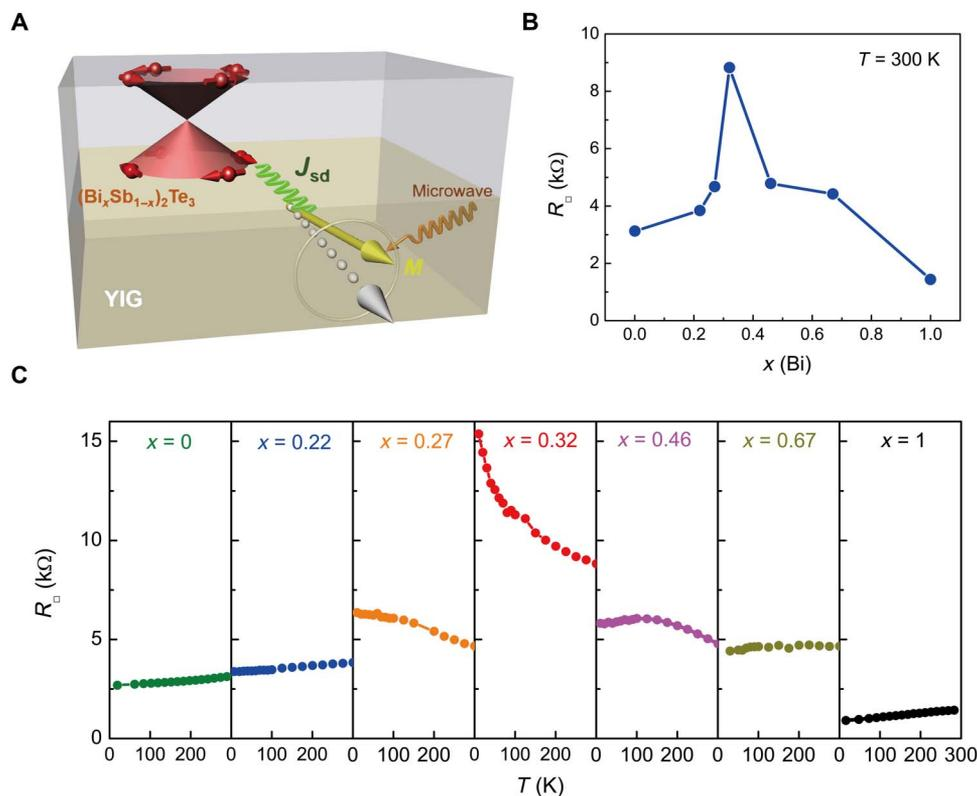
**Fig. 1. FMR measurement principle and TI properties.** (A) Schematic drawing of magnetization dynamics in YIG interfaced with TI in which the spin of the surface state electron is locked to momentum. (B) Room temperature sheet resistance of  $(\text{Bi}_x\text{Sb}_{1-x})_2\text{Te}_3$  with different Bi concentrations. (C) Temperature dependence of the sheet resistance of seven YIG (10 nm)/ $(\text{Bi}_x\text{Sb}_{1-x})_2\text{Te}_3$  (five QLs) heterostructures.
