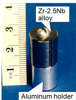
**Figure 2.** Construction of Zr-2.5Nb sample for texture measurements [16].
