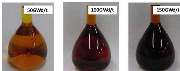
Fig. 3. Appearance of non-radioactive simulated waste under different burn-up conditions.
