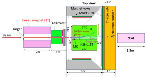
Fig. 6. The top view of the hypernuclear spectrometer.
