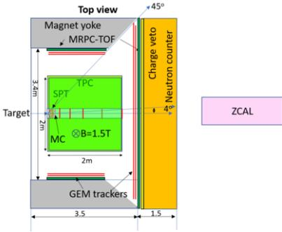
Fig. 1. The top view of the hadron spectrometer.
