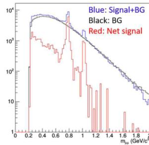
Fig. 8. The fully simulated and reconstructed dimuon spectrum.
