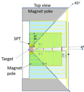
Fig. 5. The top view of the dimuon spectrometer.
