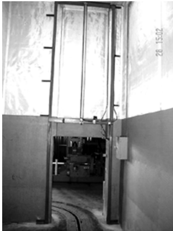
Fig. 3 Pneumatic shutter doors (access control for product and workers)
