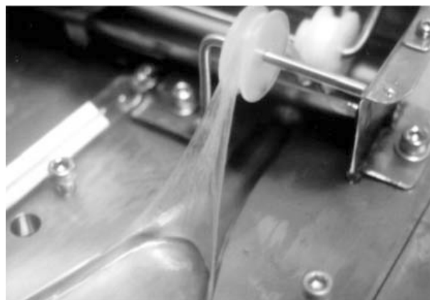
Fig. 2 The wind up of BC fiber bundle directly from medium surface
