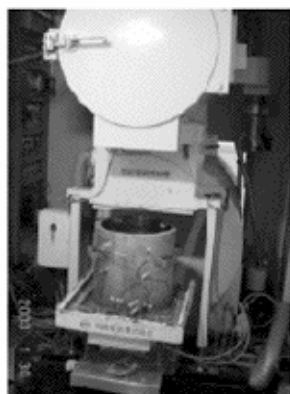
Liquid irradiation system using low energy EB (250keV, 10mA)
