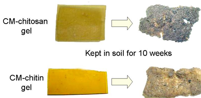
Fig. 5 Soil burial tests of CMChit and CMChTs hydrogels, 1mm thick, before and after keeping in soil for 10 weeks.
