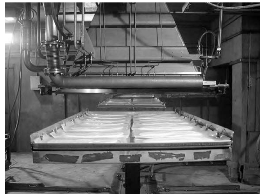
Fig. 4 Electron beam processing of sago hydrogel facial mask.
