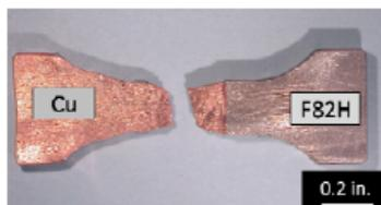
Fig. 7: Tensile sample HIP'ed at 650 ° C, showing fracture at interface (left). Tensile sample HIP'ed at 850 ° C, showing ductile failure in copper (right).
