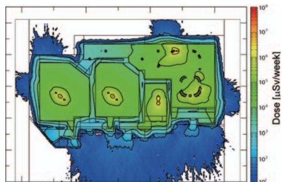
Fig. 5 Example of neutron-dose distribution calculated by PHITS for a typical proton therapy facility.
