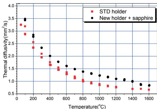
Fig. 10 Comparison of data between STD holder and new holder (Cape-Lehman model)
