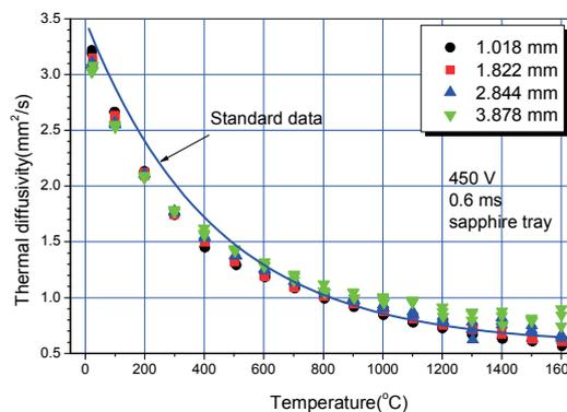
Fig. 13 The thickness effect ( $UO_2$  disk samples)
