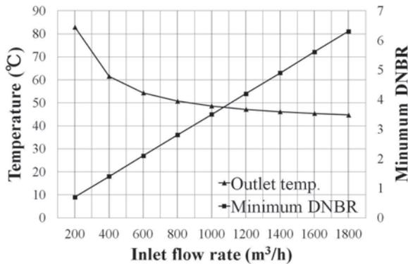
Fig.6. Change of minimum DNBR and reactor outlet temperature as a function of inlet flow rate.
