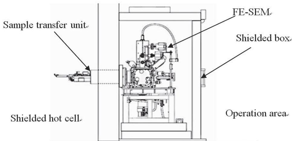
**Figure 1** Schematic diagram of the modified FE-SEM.
