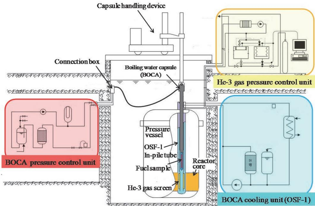
Fig.1 Schematic configuration of fuel transient test facility
