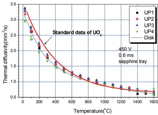
Fig. 15 The thermal diffusivity of UO<sub>2</sub> crack samples
