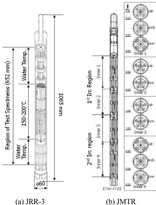
Fig.4 Configuration of irradiation capsule in JRR-3 and JMTR.
