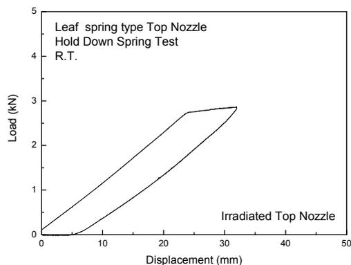
Fig. 12. Typical test results of a hold down spring test for the leaf spring type top nozzle
