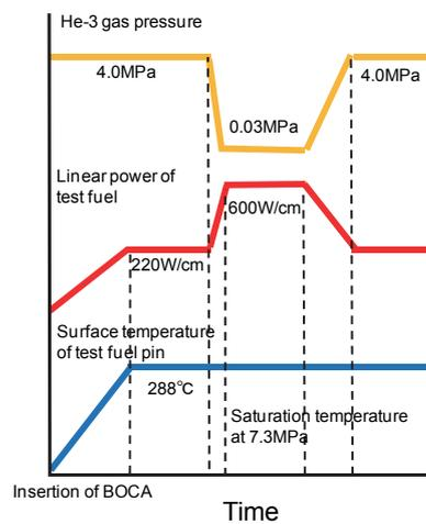
Fig.3 Example of power ramping test of JMTR
