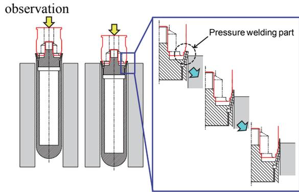
Fig.4 Process of pressure welding of the rabbit
