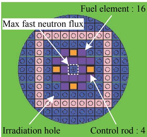
Fig.2. Calculation model by MCNP (standard core)
