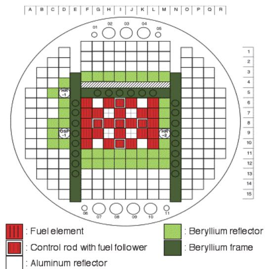
Fig. 1 Core arrangement of JMTR.
