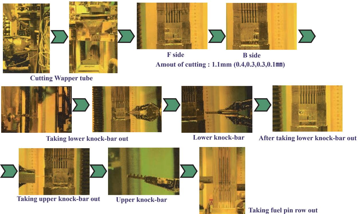
Figure 8 disassembling procedure of the first row
