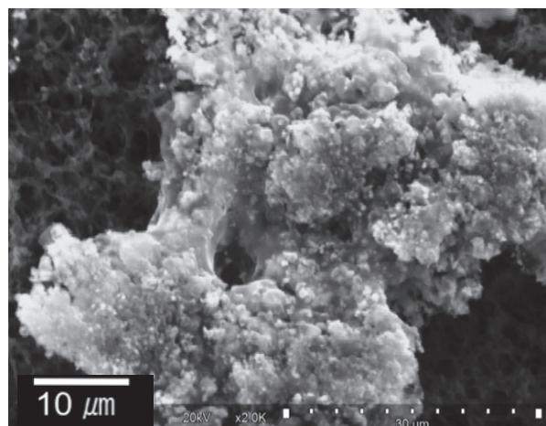
Fig.1. SEM of a crud flake.
