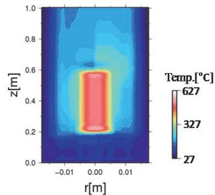
Fig.7 Calculation results under BWR conditions on the liner power of 600 W/cm.
