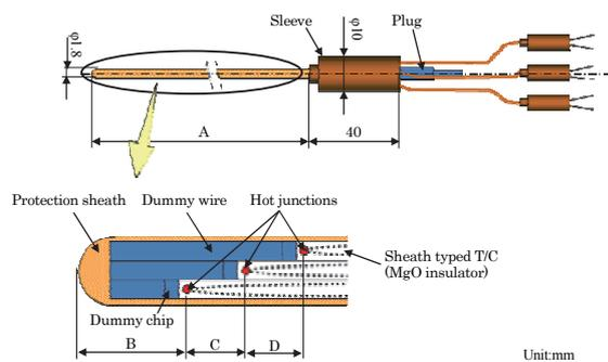
Fig.1 Structure of multi-paired thermocouple.
