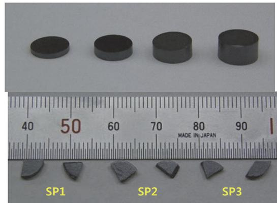
Fig. 4 UO<sub>2</sub> samples with different thickness
