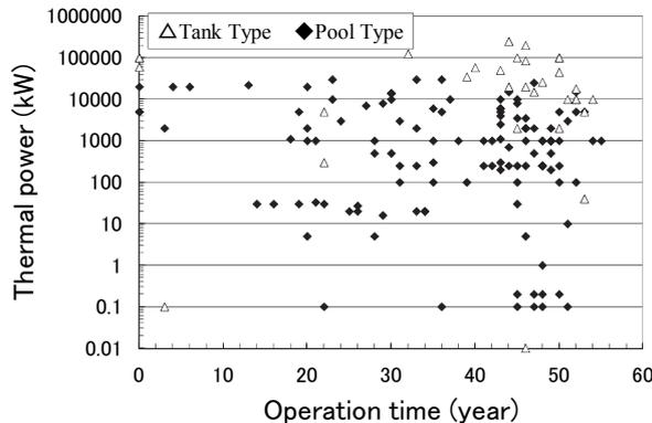
Fig.1. Relation between reactor type (tank type and swimming pool type) and thermal power in world test research reactor.
