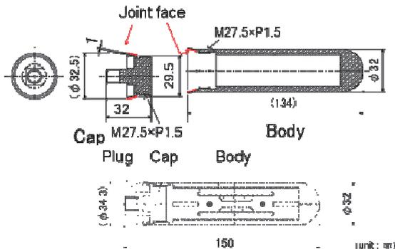
Fig.3 Structure of pressure welding type hydraulic rabbit
