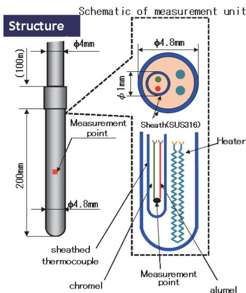
Fig.6 Structure of water level sensor.
