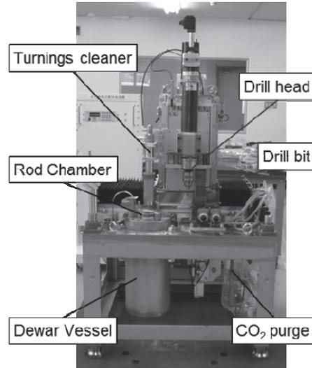
Fig. 6 Improved center boring device
