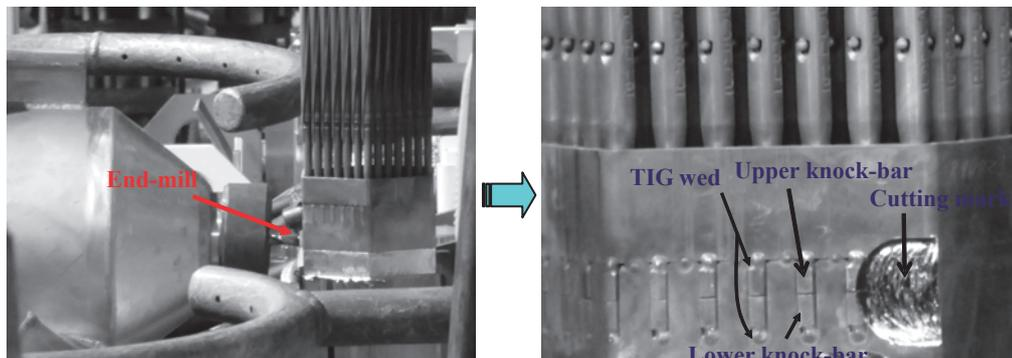
Figure 6 Cutting knock-bar weld
