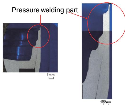
Fig.5 Metallographic observation of the rabbit
