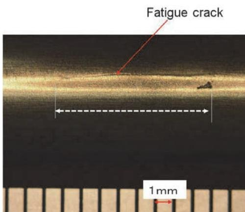
Fig.3 Photograph of fatigue crack Appearance.
