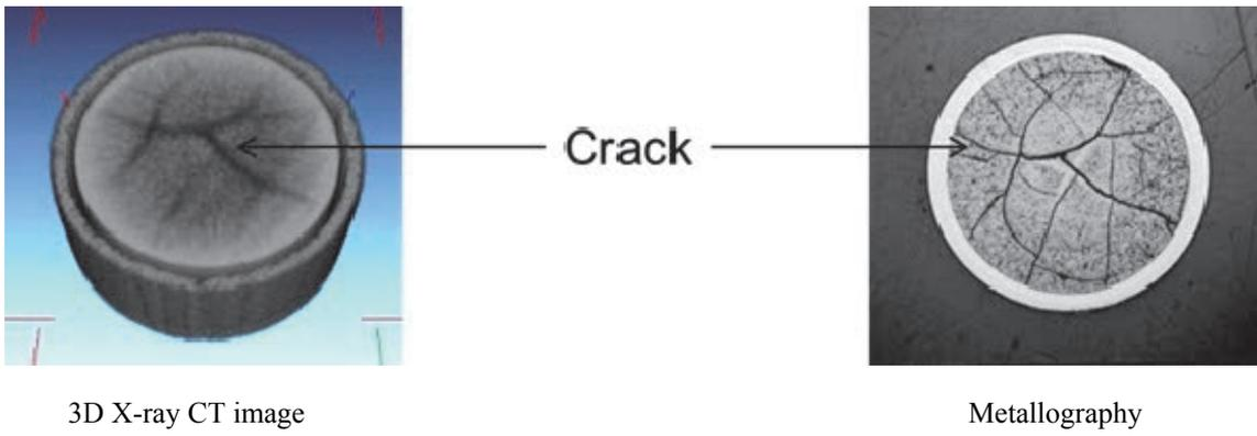
(c) Crack of the pellet surface
