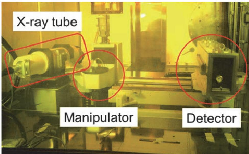
Fig.3 The X-ray scanner system in hot cell.
