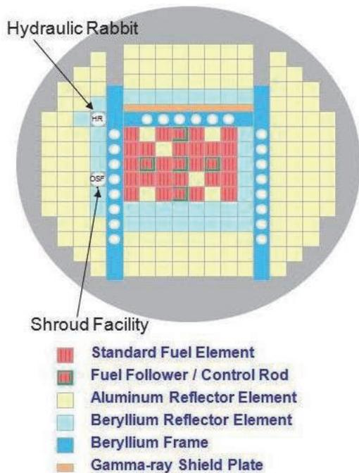
Fig.2 Cross Section of the Core.
