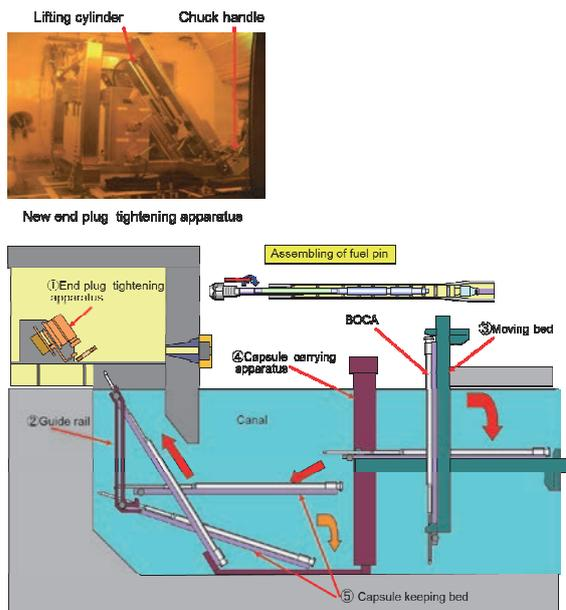
Fig.2 Schematics of the new capsule assembling apparatus.
