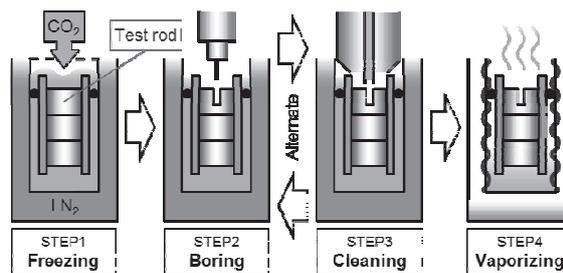
Fig. 2 Processing steps of center boring device
