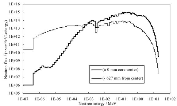
Fig. 2. Neutron spectra at the U samples irradiation position
