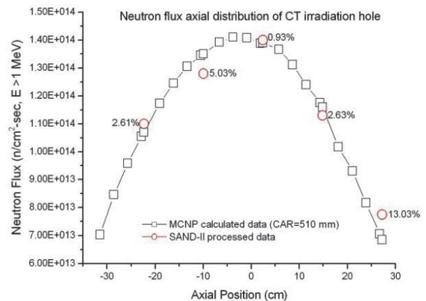
Fig. 7. The comparison fast neutron flux between the calculated and measured value of 10M-01K capsule
