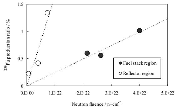
Fig. 6. <sup>239</sup>Pu production ratio as a function of neutron fluence
