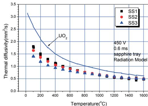
Fig. 14 The thermal diffusivity of SIMFUEL
