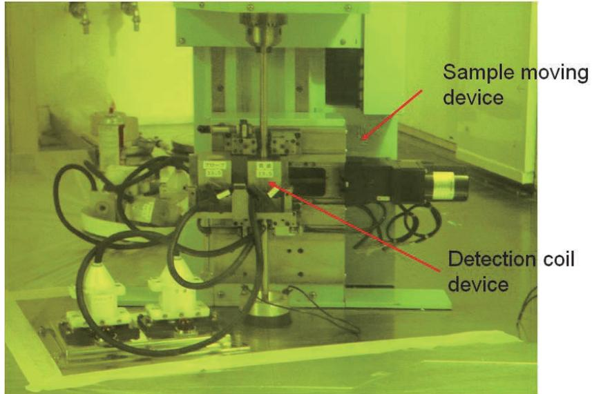
Fig.1 In cell device of eddy current test equipment.
