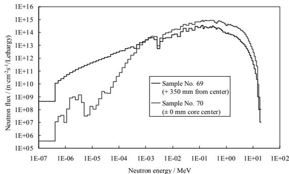
Fig. 1. Neutron spectra at the Am samples irradiation position
