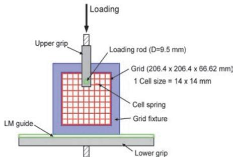
Fig.1. Conceptual drawing of a cell spring test
