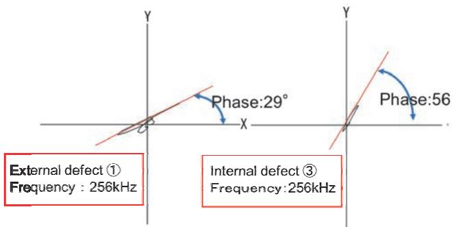
Fig. 7 Pattern of standard defect.
