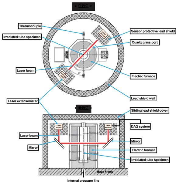
Figure 2. Measurement concept of diametral creep strain of irradiated cladding tube
