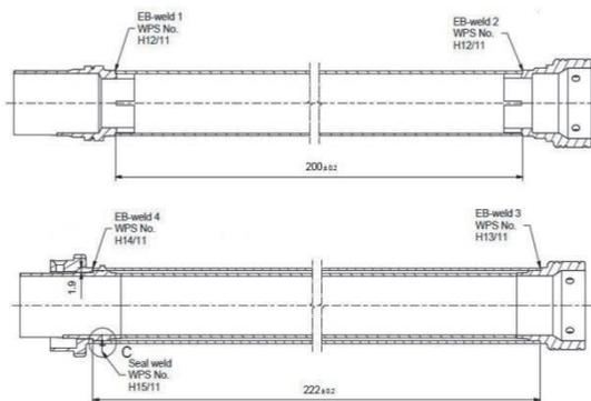
Fig 2. Critical weld points of an insulated test channel welded for WPS documents.
