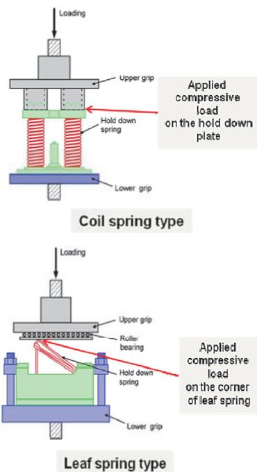
Fig.5. Conceptual drawing of a hold down spring test
