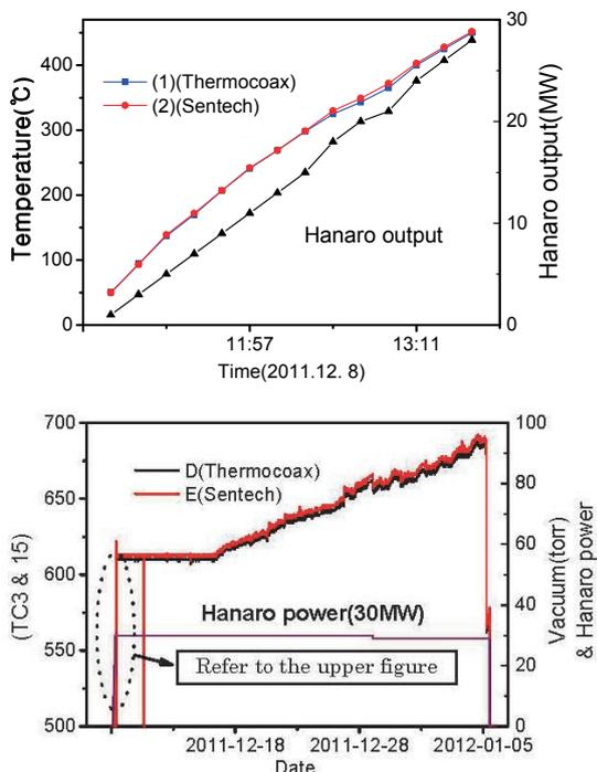
Fig.5 Result of the Thermocoax and Sentech thermocouple in HANARO test.
