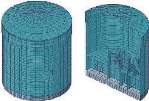
Fig.4. 3D FEM model of reactor building
