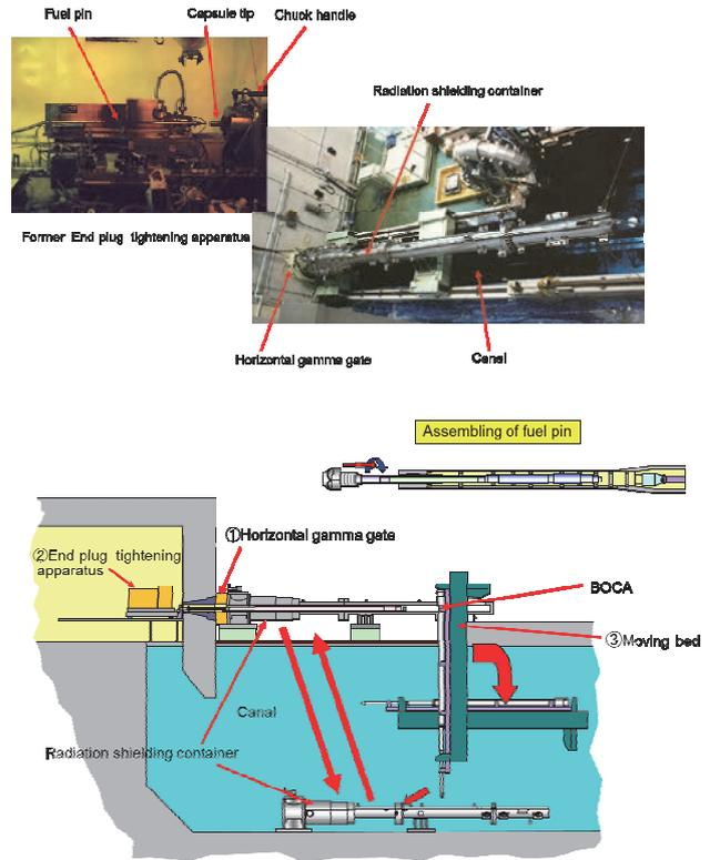
Fig.1 Schematics of the former capsule assembling apparatus.
