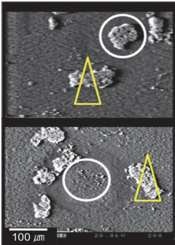
Fig.2. BSE of crud before and after burning.
