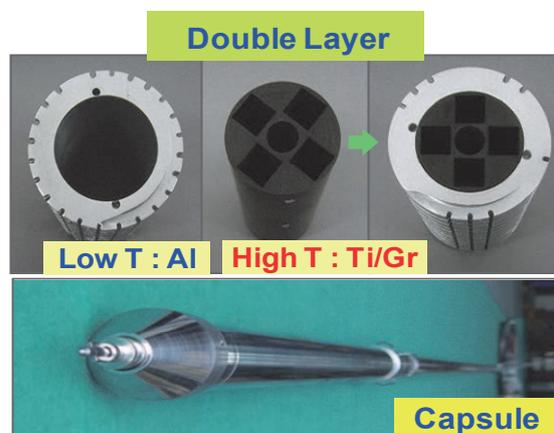
Fig.4 Double layered thermal media and high temperature irradiation capsule.
