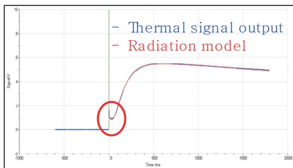
Fig. 11 The radiation model behavior
