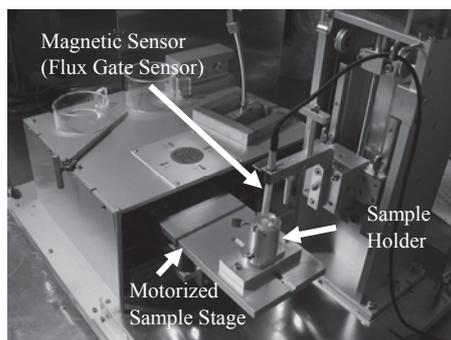
Fig.2. Remote-controlled apparatus for measurement of magnetic flux density.
