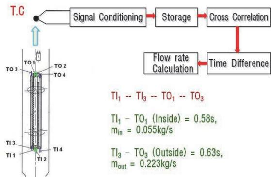
Fig 12. The noise analysis process performed during the ATL test
