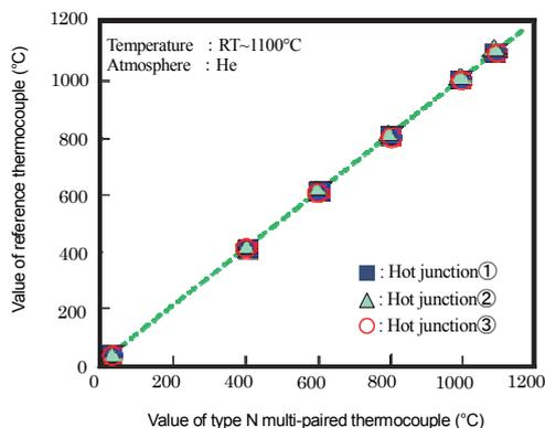
Fig.3 Result of Demonstration test with type-N multi-paired thermocouple [3].
