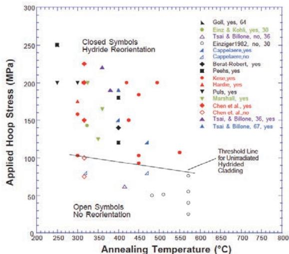
Figure 3. NRC Evaluation of hydride reorientation, Einziger et al., 2005.
