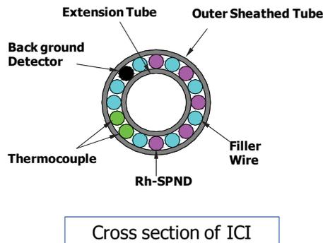
Fig.10 In-Core-Instrument containing several localized SPNDs.
