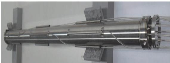
Fig 8. SPND mounted on the insulated test channel assembly
