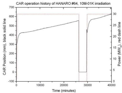
Fig. 5. The CAR operation history of 64<sup>th</sup> operation cycle of HANARO
