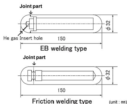
Fig.2 Structures of EB welding type hydraulic rabbit and friction welding type rabbit in JMTR
