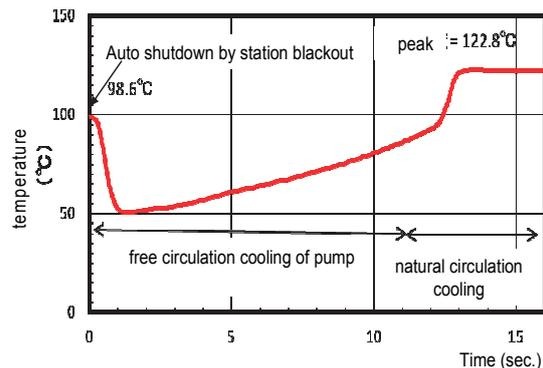
Fig.2. The maximum fuel surface temperature after the auto shutdown by station blackout
