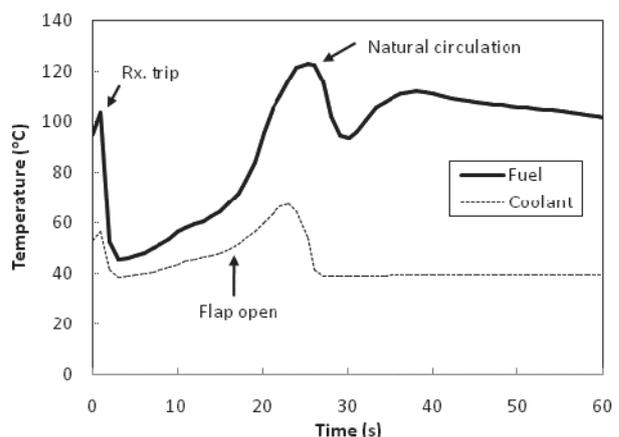
Fig.1. Typical temperature behaviors at LOFA
