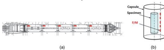
Fig. 3. The schematic diagrams of installed F/M in a capsule
