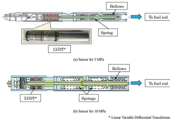
Fig.6 Structure of rod inner pressure gauges.
