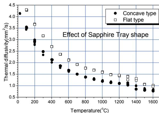
Fig. 8 Effect of sapphire tray shape
