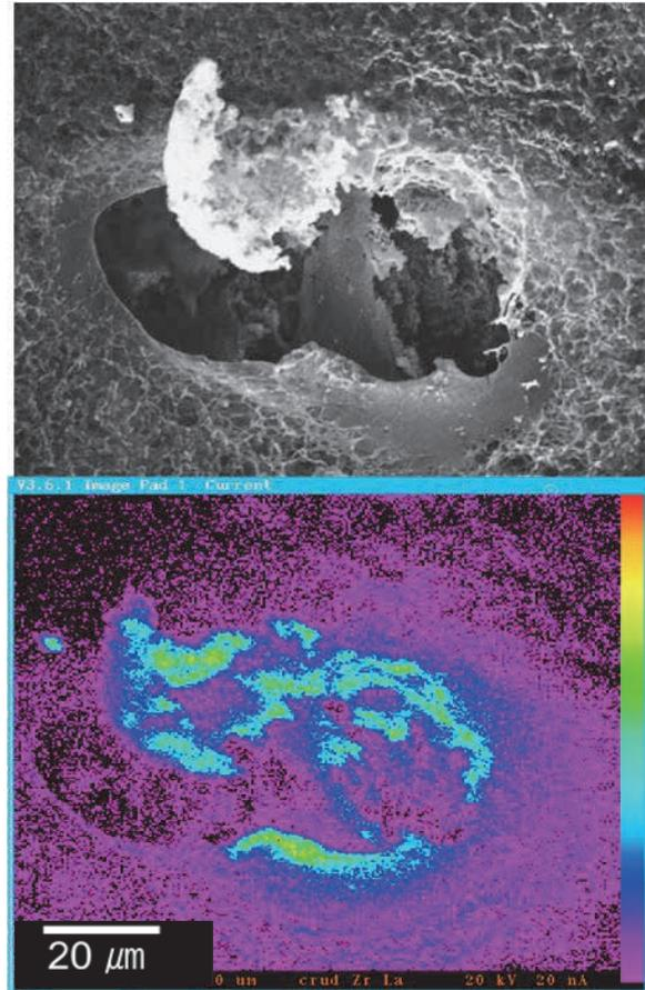
Fig.4. BSE and X-ray map of crud flake after burning.
