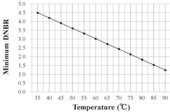
Fig.5. Change of minimum DNBR as a function of core inlet temperature.
