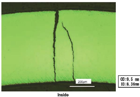
Fig. 9 Fatigue crack of Metallography.
