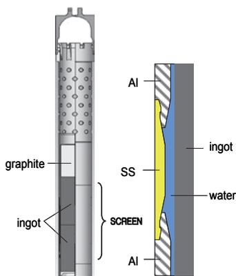
Fig. 3 Irradiation rigs and neutron screen
