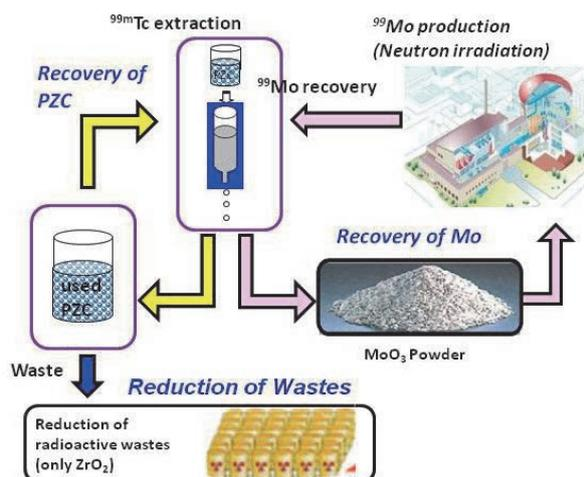
Fig.2 Concept of Mo recycling (in case of PZC).
