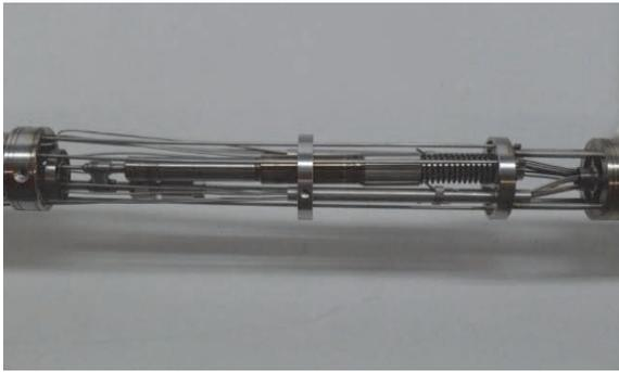
Fig 7. LVDT mounted between DCF rod and cable tube
