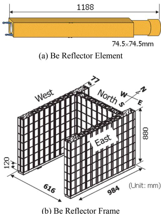
Fig. 2 Configuration of Beryllium reflectors in JMTR.
