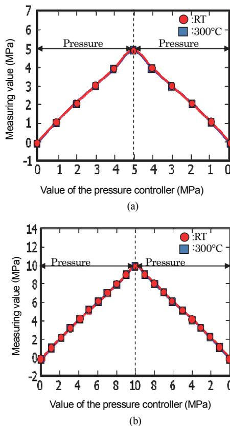
Fig.7 Results of performance test with rod inner pressure gauge:(a) 5 MPa, (b) 10 MPa.
