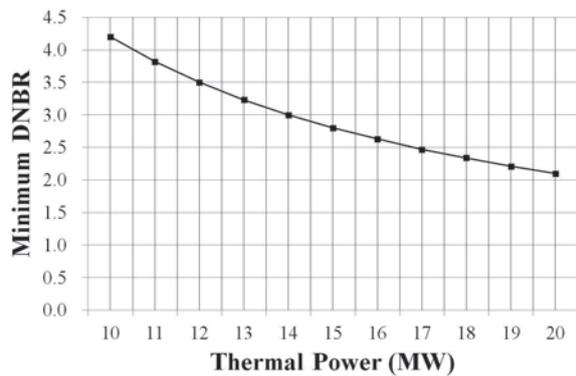
Fig.7. Change of minimum DNBR as a function of thermal power.
