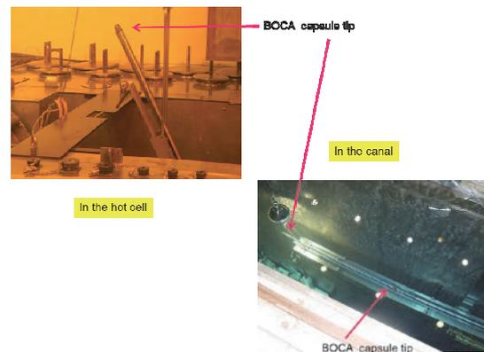
Fig. 3 BOCA capsule during mock-up test
