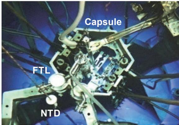
Fig.1 Reactor core of HANARO.
