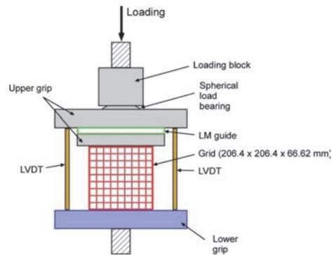
Fig.3. Conceptual drawing of a static buckling test
