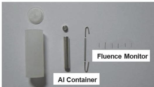
Fig. 2. F/Ms and containers used in this study
