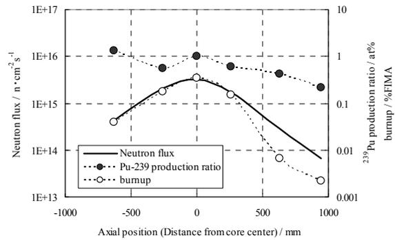
Fig. 5. Axial distribution of the <sup>239</sup>Pu production ratios, the burnups in the irradiated U samples and neutron flux in the subassembly SVIR-1
