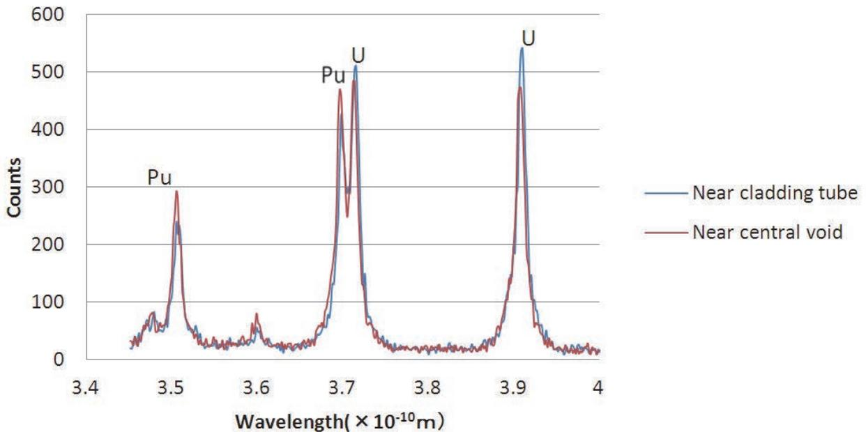
**Figure 3** Elemental analysis results of the fuel sample by WDX
