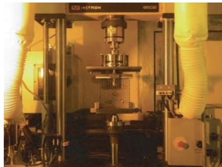
Fig.4. Test fixture of a static buckling test
