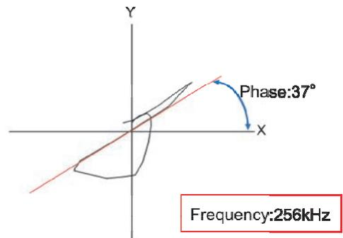
Fig. 8 Fatigue crack of X-Y pattern.
