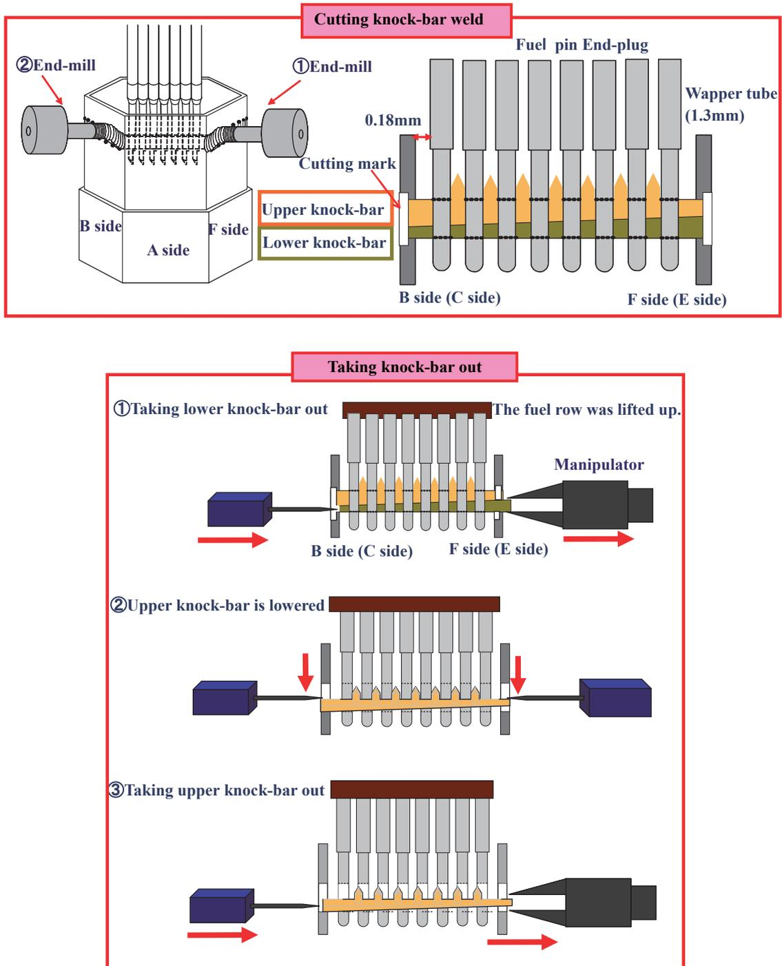
Figure 3 Caption correction work procedure
