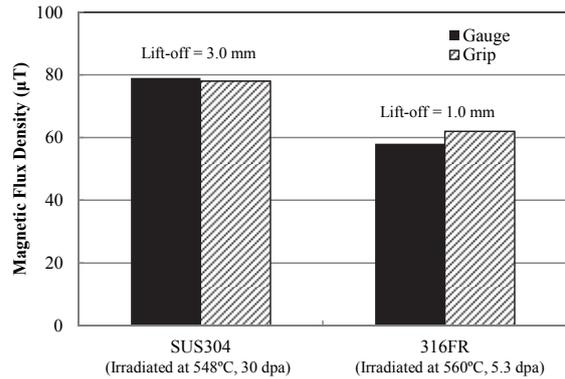
Fig.5. Comparing magnetic flux density between two sample shapes.
