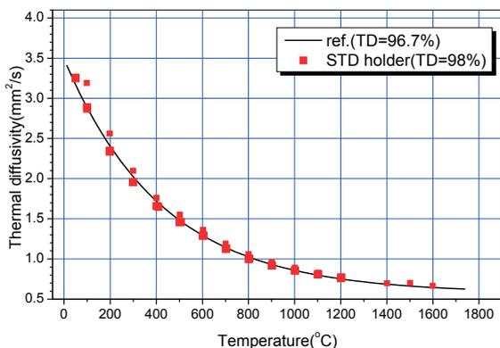
Fig. 6 Comparison of thermal diffusivity between vacuum state and flowing gas state.
