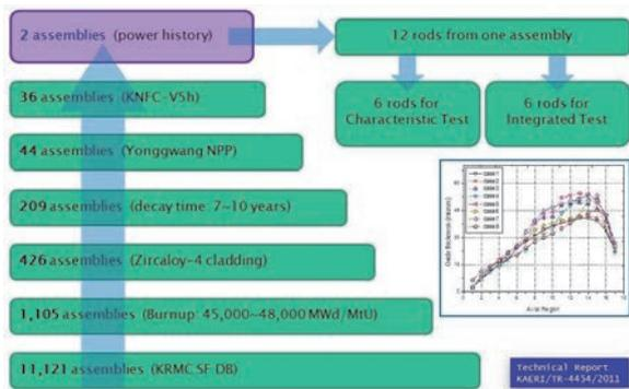
Fig.1. Selection of target spent fuel rods.
