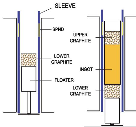
Fig. 5 Irradiation hole before and after loading a rig
