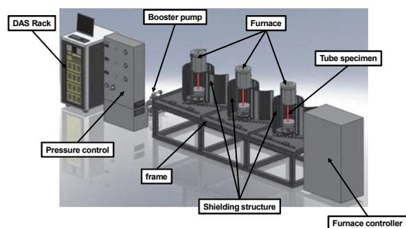
Figure 1. Multi-channel irradiated clad tube creep tester
