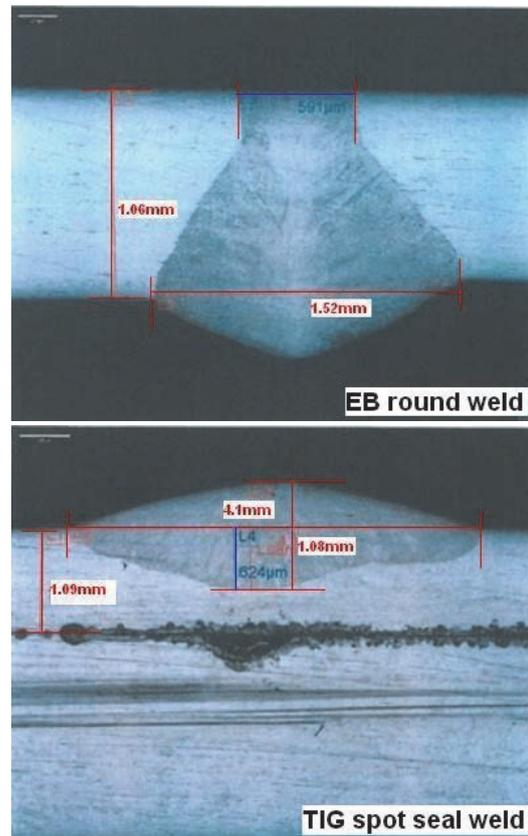
Fig 3. The microstructures of samples welded in the qualification test.
