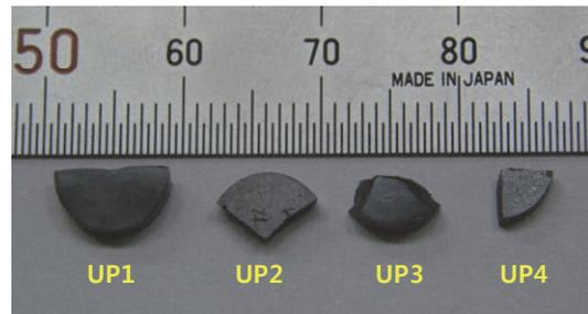
Fig. 2 Crack samples of UO<sub>2</sub>
