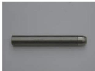
Fig.7. Dummy cladding for a cell spring test
