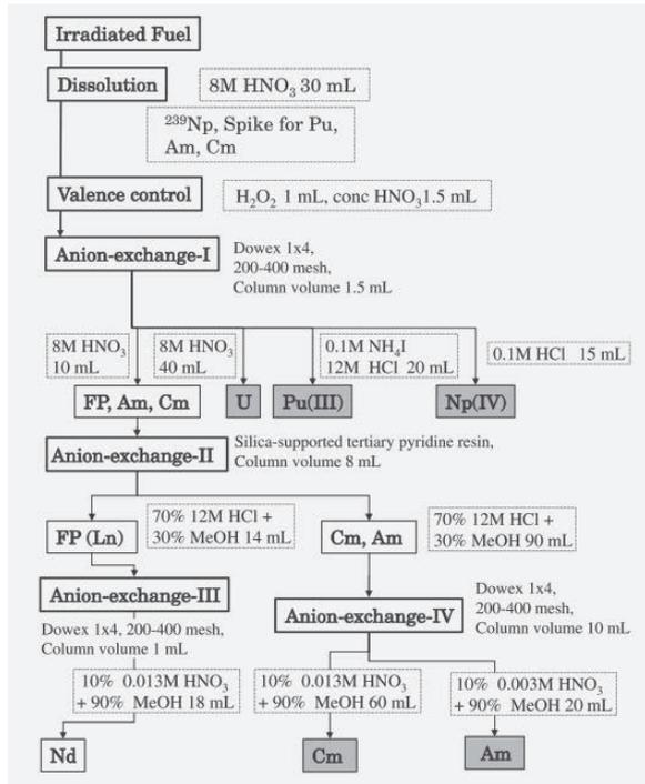
Fig. 3. Schematic flow sheets of chemical analysis
