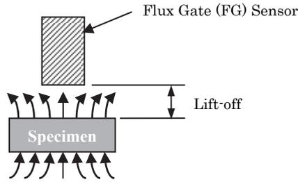
Fig.3. Schematic view of measuring magnetic flux density.
