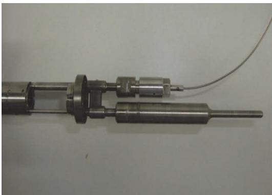
Fig 5. TC mounted on the top of DCF rod.
