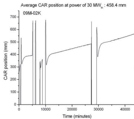
Fig. 4. The CAR operation history of 63<sup>rd</sup> operation cycle of HANARO
