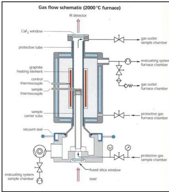
Fig. 1 Diagram of LFA
