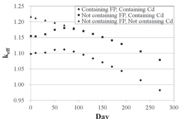
Fig.4. Effective multiplication factor ( $k_{eff}$ ) as a function of operation days, obtained by COREBN
