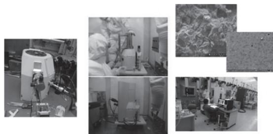
Fig. 11 Installation of SEM in a hot cell
