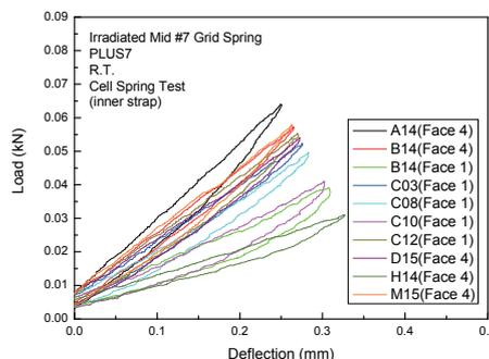
Fig.9. Typical test results of a cell spring test
