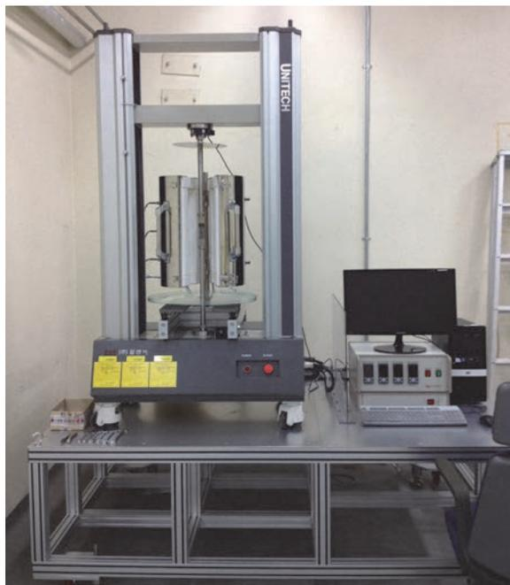
Figure 4. Hydride reorientation tester in PIEF hot Lab.
