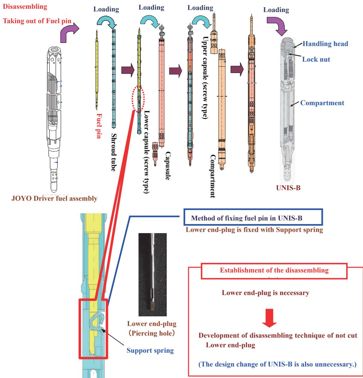
Figure 2 Method for loading UNIS-B
