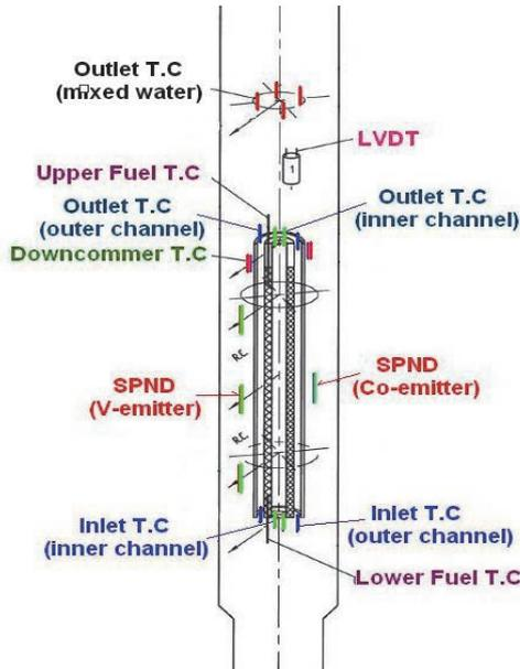
Fig 4. Position of sensors instrumented in the test rig.
