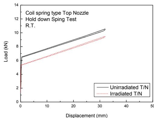
Fig. 11. Typical test results of a hold down spring test for the coil spring type top nozzle
