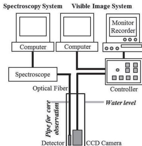
Fig.9 Cherenkov light measurement apparatus.
