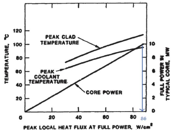
Fig.2. Temperatures and core power with heat flux
