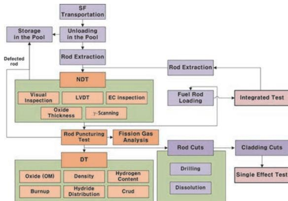
Fig.2. Characteristic test of the spent fuel rod.
