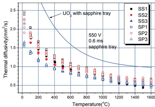
Fig. 16 The thermal diffusivity of SIMFUEL cracked samples
