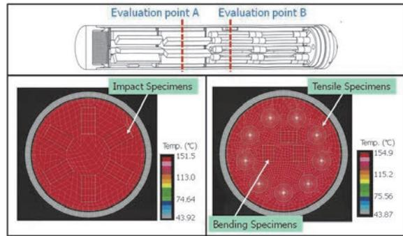
Fig.5 Result of irradiation temperature calculated by NISA.
