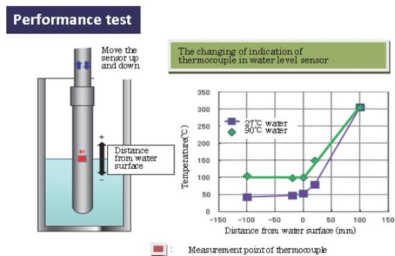
Fig.8 Results of performance tests.
