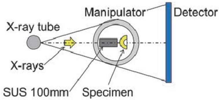
(a) Schematic of transmissivity test
