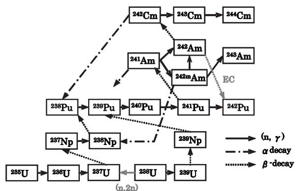
Fig. 4. Main transmutation chains of actinides in fast reactor
