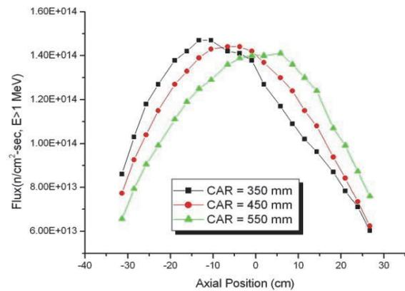
Fig. 1. The calculated axial neutron flux distribution for a 10M-01K capsule irradiated in a CT hole
