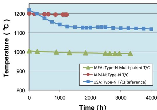
Fig.4 Result of the type-N multi-paired and type-N thermocouple in endurance tests.
