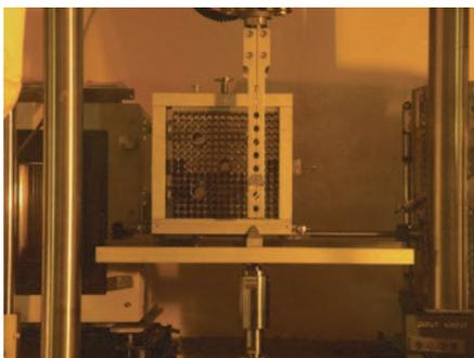
Fig.2. Test fixture of a cell spring test
