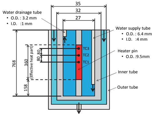
Fig.5 Schematic configuration of analysis model.
