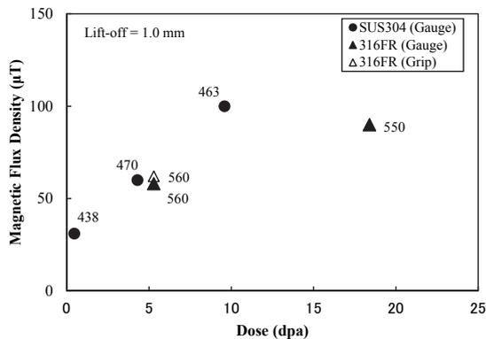
Fig.4. Relationship between irradiation dose and magnetic flux density for SUS304 and 316FR. Values in the plot mean irradiation temperatures (°C).
