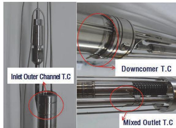
Fig 6. Coolant TCs installed in the test rig.
