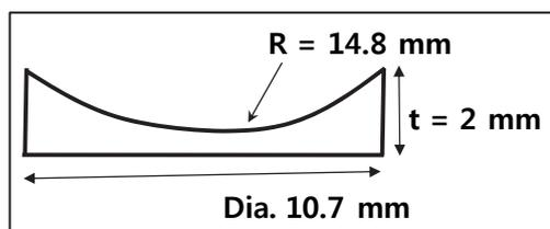
Fig. 7 Geometry of concave sapphire tray
