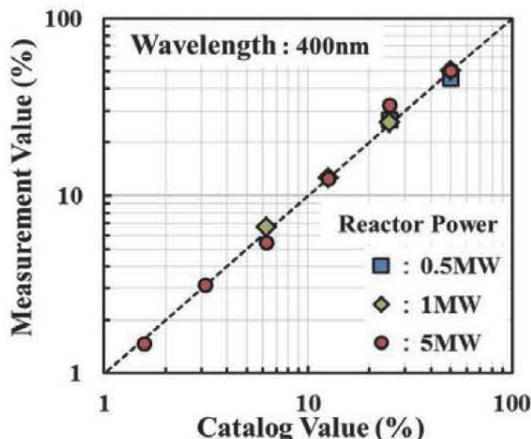
Fig.10 Characteristics of the ratio of transmitted light of the Cherenkov light by dimming filter.
