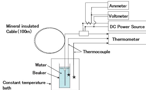
Fig. 7 Test apparatus of performance tests
