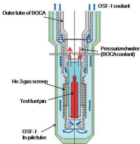
Fig.2 Schematic of the core part of BOCA/OSF-1
