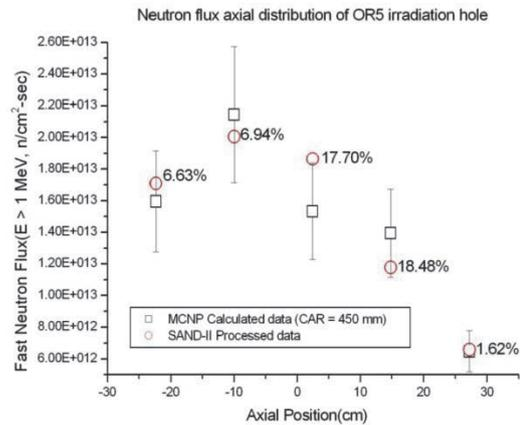
Fig. 6. The comparison fast neutron flux between the calculated and measured value of 09M-02K capsule
