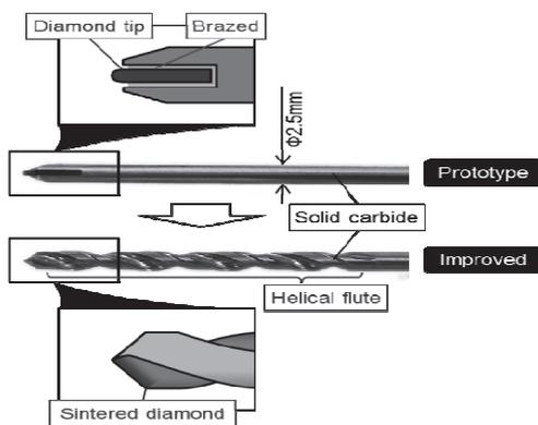
Fig. 3 Comparison of drill bits
