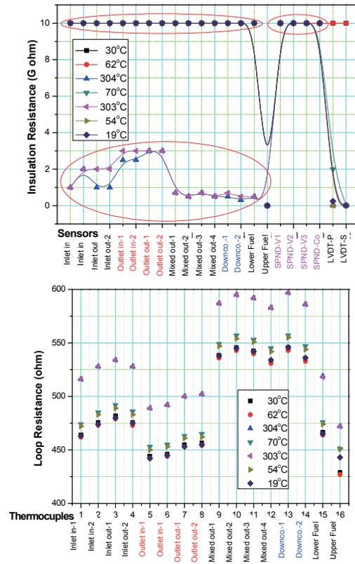
Fig 11. Insulation resistance and loop resistance values measured for signal cables
