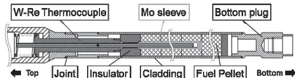
Fig. 1 Fuel rod for Power ramp test
