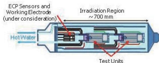
Fig.1 Schematic drawing of the in-pile test.
