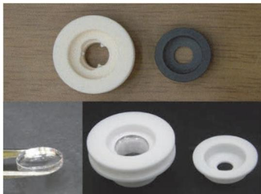
Fig. 5 Standard holder(up) and new holder with sapphire tray(down)
