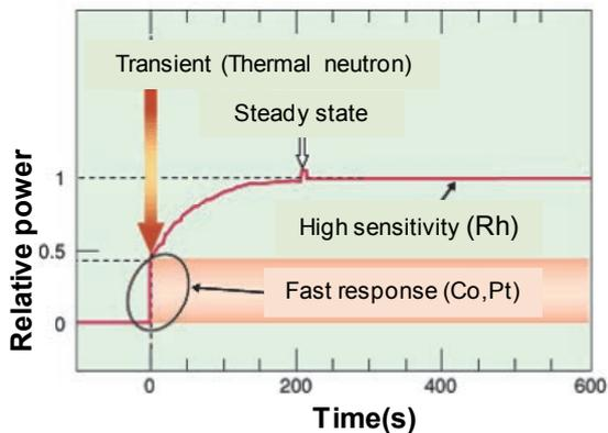
Fig.9 Hybrid SPNDs transient response when the thermal neutron flux was changed.
