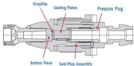
Fig 9. Top seal assembly (Graphite Sealing)
