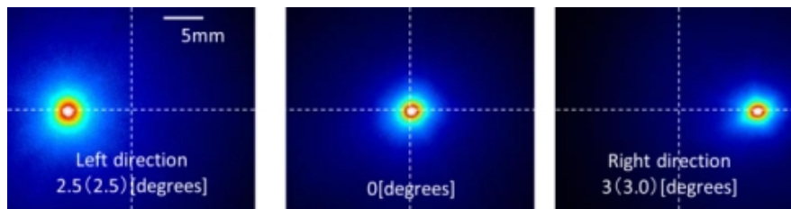
Fig.1: Direction control of electron beam by external magnetic field ( B=0.2\text{ T} ).
