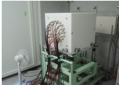
FIG. 7. Flat-efficiency neutron detector developed and used for the ^{209}\text{Bi} and ^9\text{Be} experiments in 2015.
