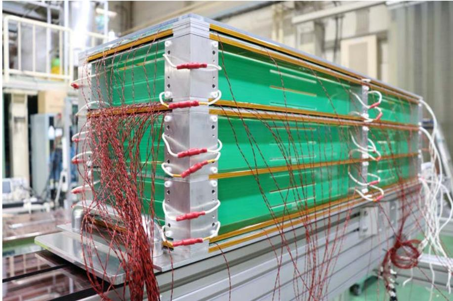
**Fig. 3.** A picture of TPC we have constructed. The TPC consists of 3 drift layers, and the signal region is in the middle layer.
