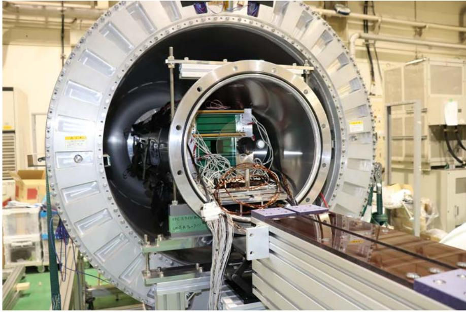
**Fig. 4.** A picture of TPC installed inside the vacuum chamber and solenoidal magnet. The integration test with this setup has carried out at KEK.
