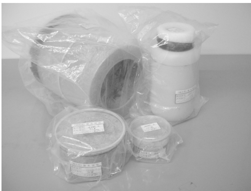
Photo 3-1 Examples of the standard volume sources. These sources are used in efficiency calibrations at the NSRI of JAEA. The filling material is the foamed Portland cement.
