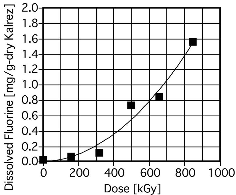
Figure 3.15-3 Quantity of dissolved fluorine vs. dose for Kalrez irradiated at room temperature
