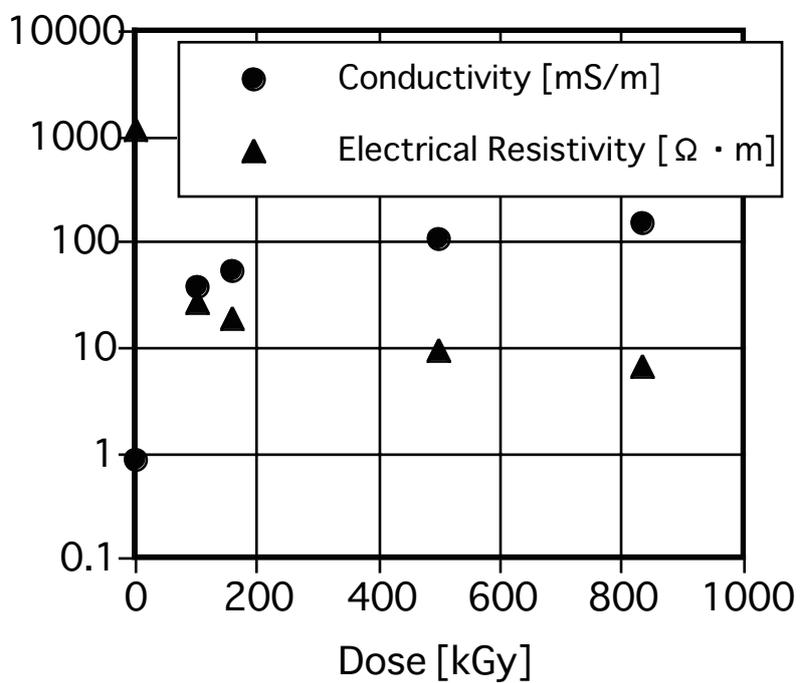
Figure 3.5-2 Conductivity and electrical resistivity of the water after irradiation
