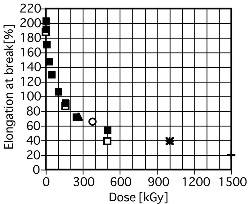
Figure 3.12-2 Elongation at break of AFLAS SF at room temperature
