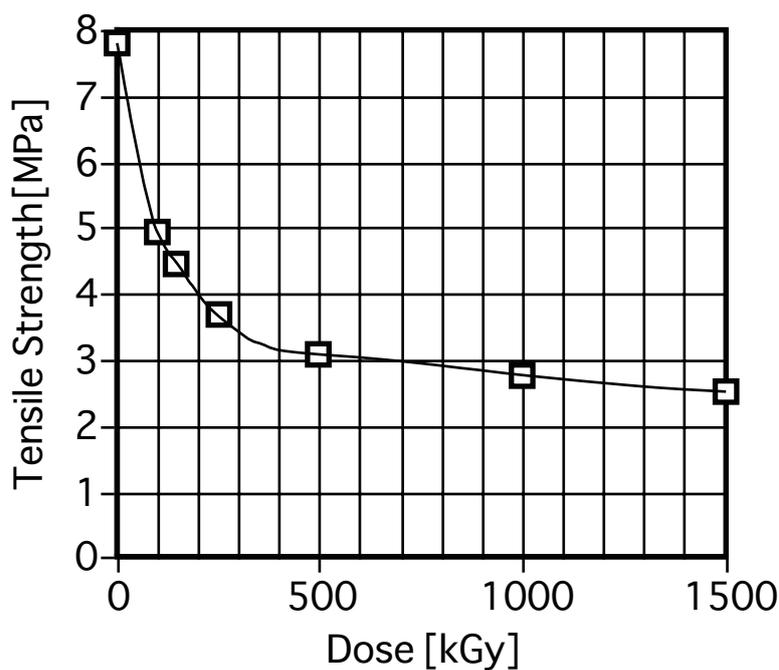
Figure 3.16-1 Tensile strength of EB-irradiated Butyl Rubber at room temperature
