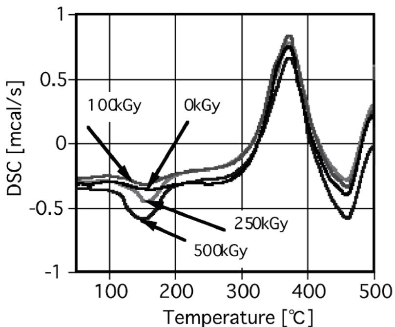
Figure 3.13-3 DSC curves of Neoprene under helium atmosphere
