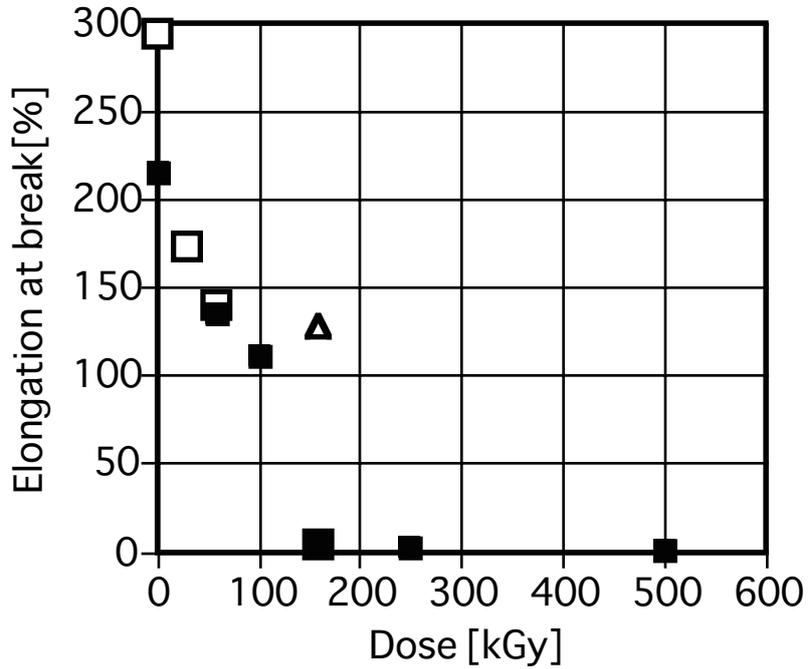
Figure 3.7-2 Elongation at break of  $\gamma$ -irradiated PFA 500LP at room temperature
