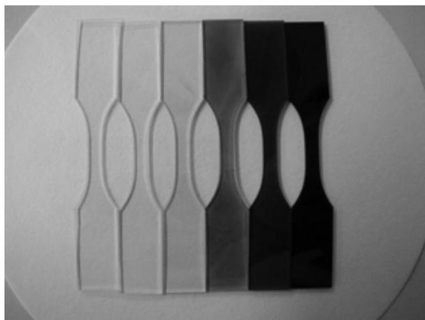
Figure 3.10-3 Coloring of EB-irradiated Polyvinyl Chloride HTGA5749 (0, 100, 160, 250, 500, 1000 kGy, vacuum-packed)
