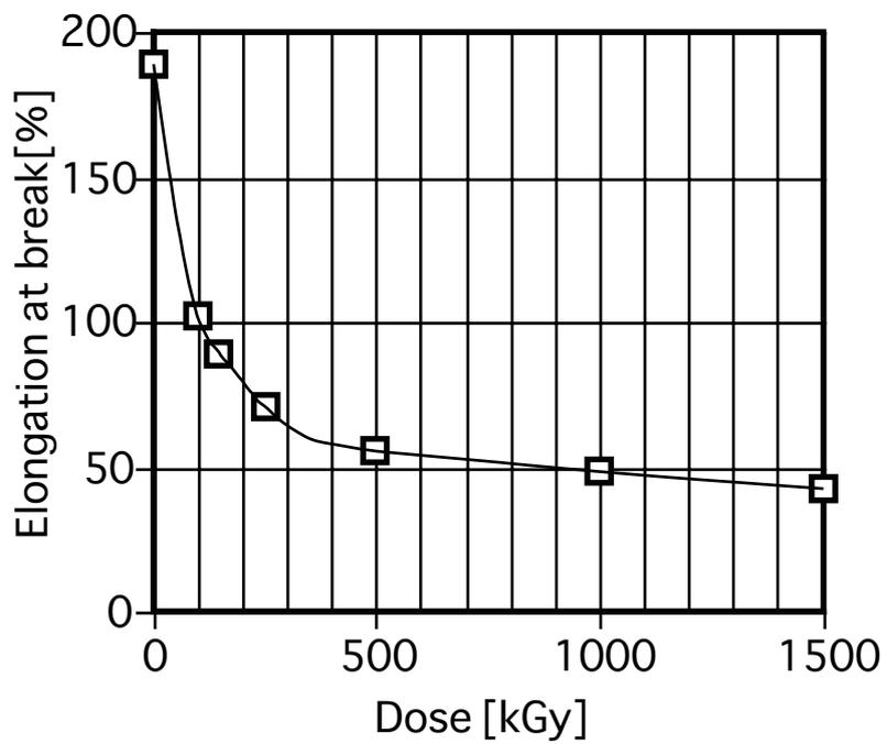
Figure 3.16-2 Elongation at break of EB-irradiated Butyl Rubber at room temperature
