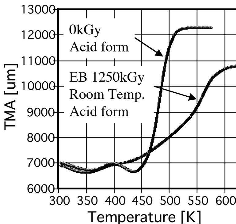
Figures 3.1-12 TMA curves of acid form Nafion N117CS membrane
