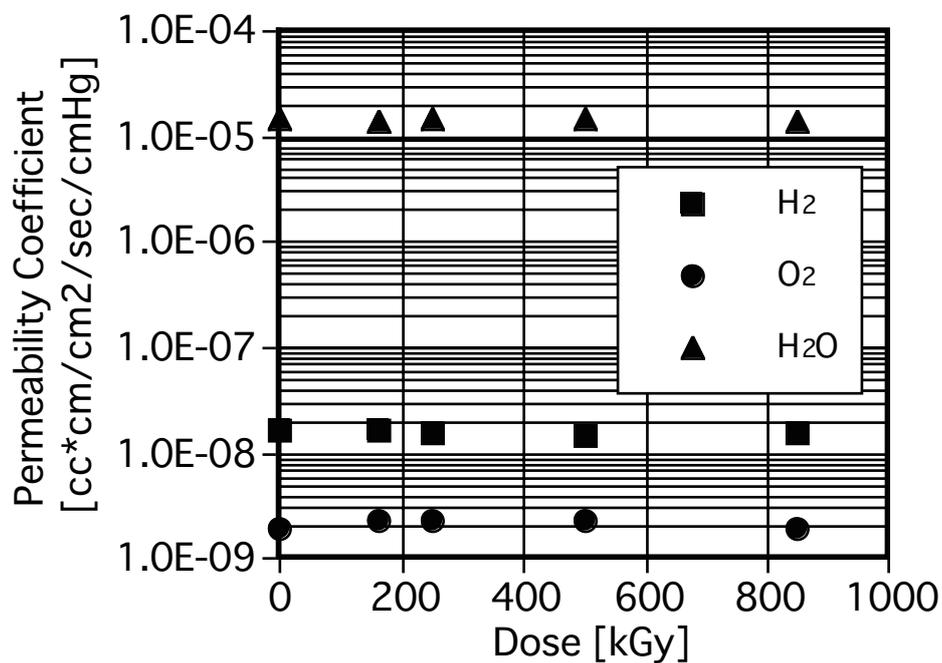
Figure 3.1-4 Permeability coefficient of  $\gamma$ -irradiated Nafion N117CS at room temperature
