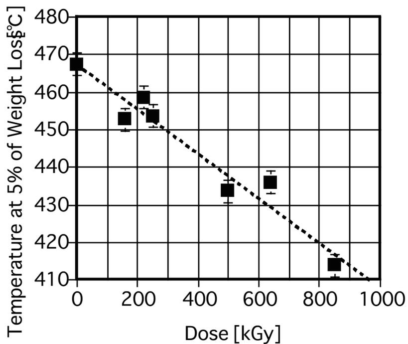
Figure 3.1-7 Temperature at 5% of weight loss of Na cation exchanged Nafion N117CS membrane under helium atmosphere
