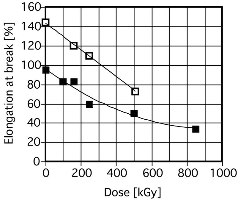
Figure 3.4-2 Elongation at break of  $\gamma$ -irradiated Nafion NE1110 at room temperature
