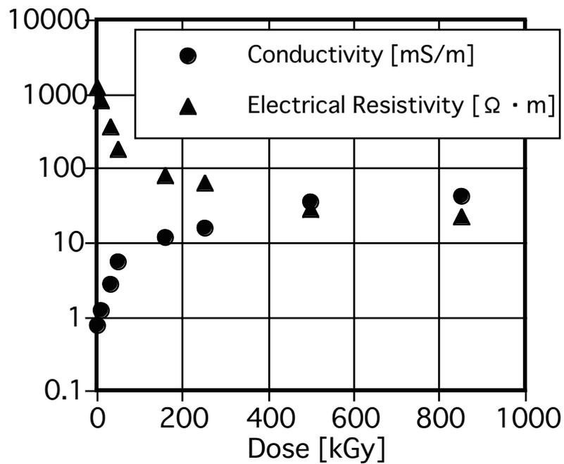
Figure 3.8-3 Conductivity and electrical resistivity of the water after irradiation
