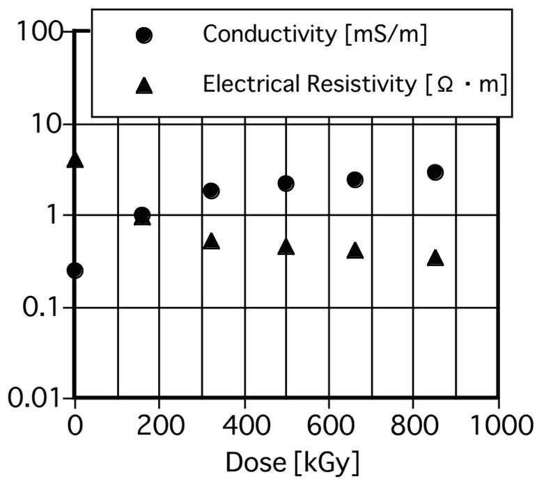
Figure 3.17-3 Conductivity and electrical resistivity of the water after irradiation
