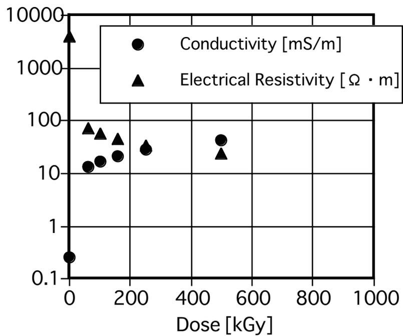
Figure 3.7-4 Conductivity and electrical resistivity of the water after irradiation
