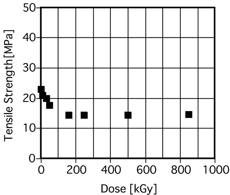
Figure 3.8-1 Tensile strength of  $\gamma$ -irradiated FEP 750A at room temperature
