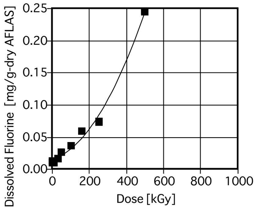
Figure 3.12-3 Quantity of dissolved fluorine vs. dose for AFLAS SF irradiated at room temperature
