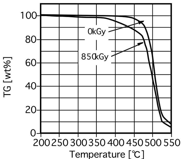
Figure 3.1-5 Weight loss curve vs. temperature of Na cation exchanged Nafion N117CS membrane under helium atmosphere
