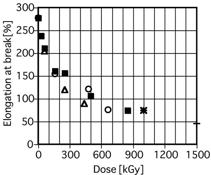
Figure 3.13-1 Elongation at break of Neoprene at room temperature
