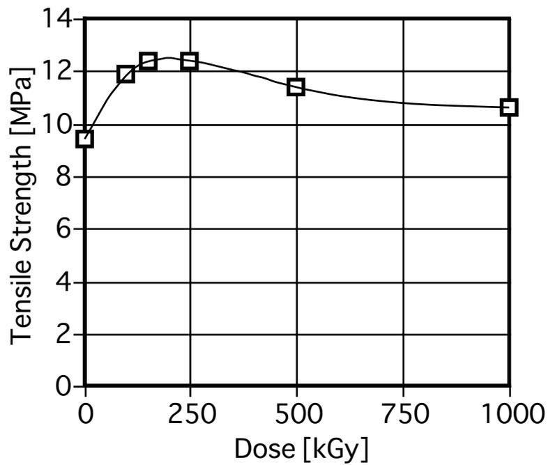
Figure 3.14-1 Tensile strength of EB-irradiated EPDM at room temperature
