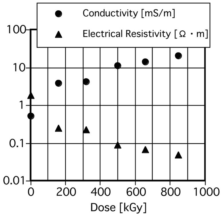
Figure 3.15-4 Conductivity and electrical resistivity of the water after irradiation
