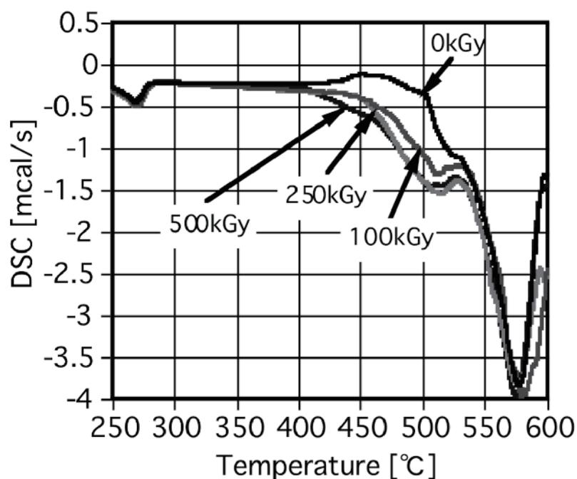
Figure 3.8-4 DSC curves of FEP 750A under helium atmosphere
