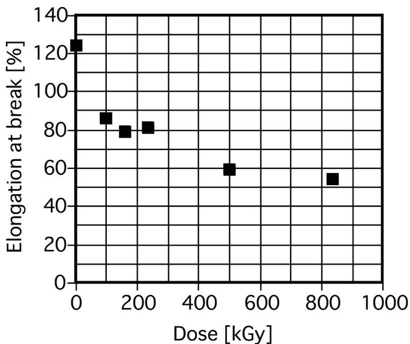
Figure 3.2-1 Elongation at break of  $\gamma$ -irradiated Nafion N112 at room temperature
