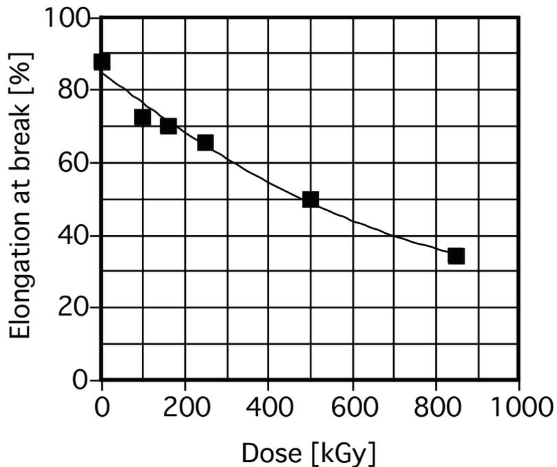
Figure 3.3-1 Elongation at break of  $\gamma$ -irradiated Nafion N115 at room temperature
