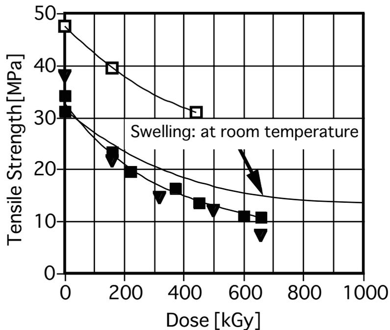
Figure 3.1-3 Tensile strength of  $\gamma$ -irradiated Nafion N117CS at 343K
