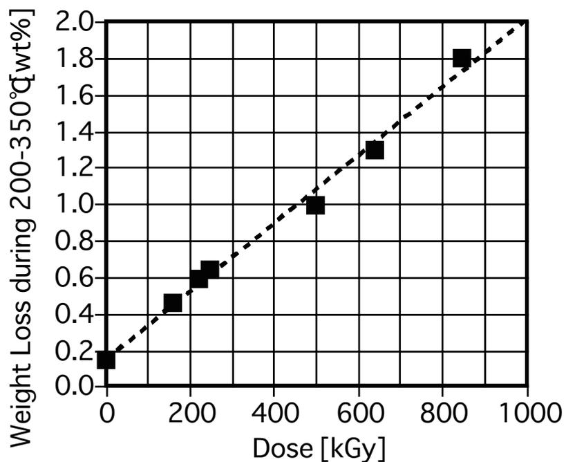
Figure 3.1-6 Weight loss of Na cation exchanged Nafion N117CS membrane between 473-623K under helium atmosphere
