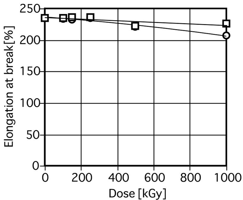
Figure 3.10-2 Elongation at break of EB-irradiated Polyvinyl Chloride HTGA5749 at room temperature
