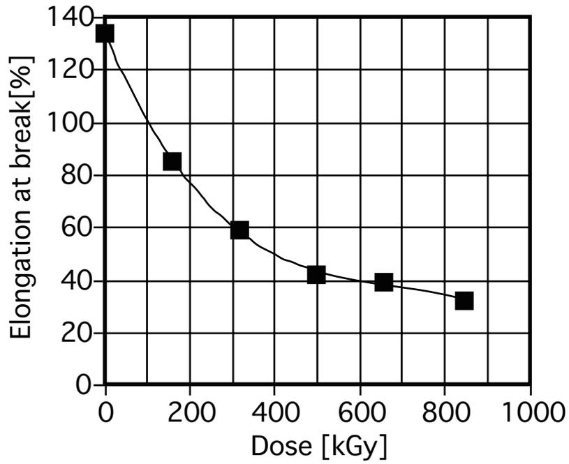
Figure 3.15-2 Elongation at break of  $\gamma$ -irradiated Kalrez at room temperature
