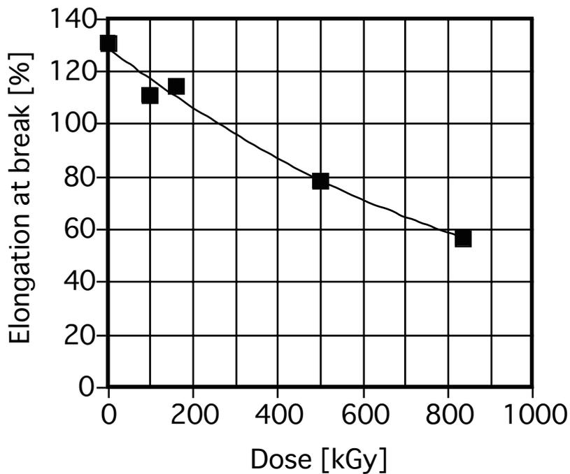
Figure 3.5-1 Elongation at break of  $\gamma$ -irradiated Nafion NE1135 at room temperature
