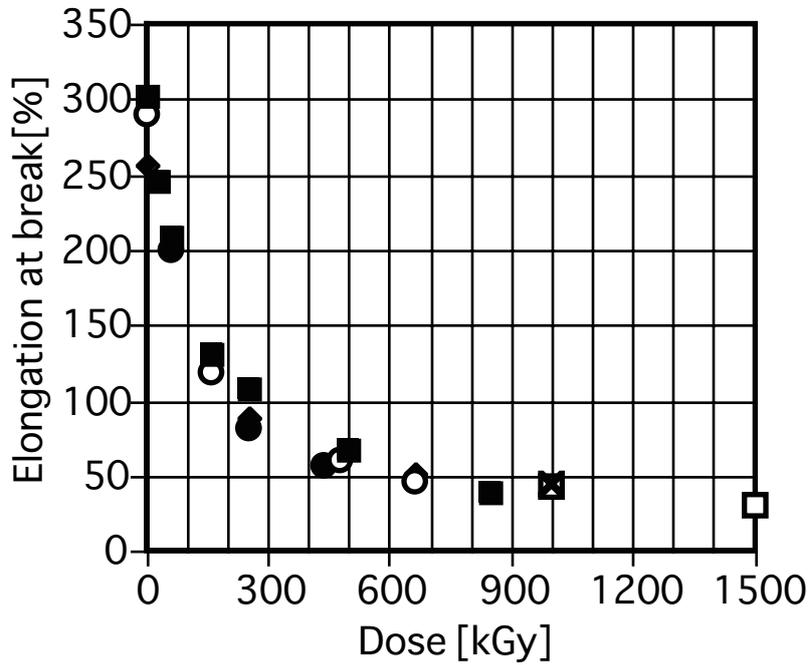
Figure 3.11-1 Elongation at break of VITON
