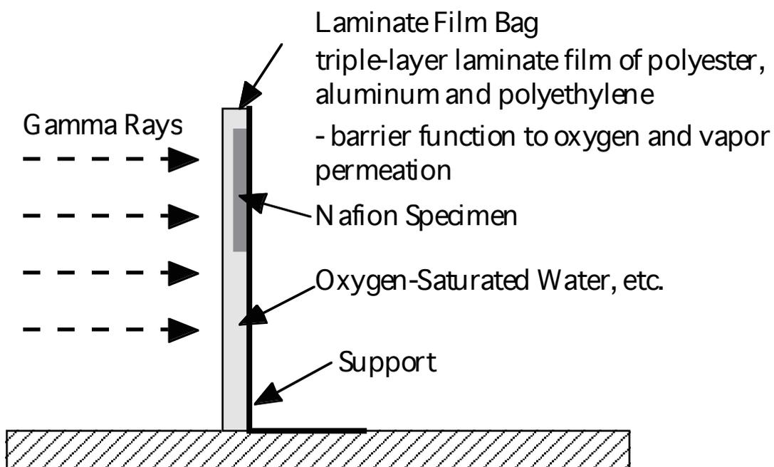
Figure 2 Structure of the TEST STAND for the gamma-rays irradiation
