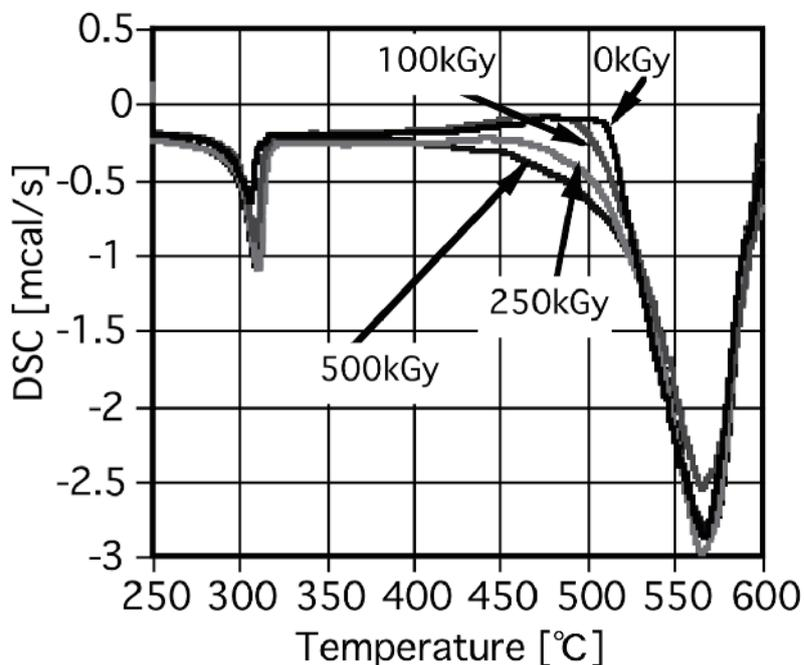
Figure 3.7-5 DSC curves of PFA 500LP under helium atmosphere
