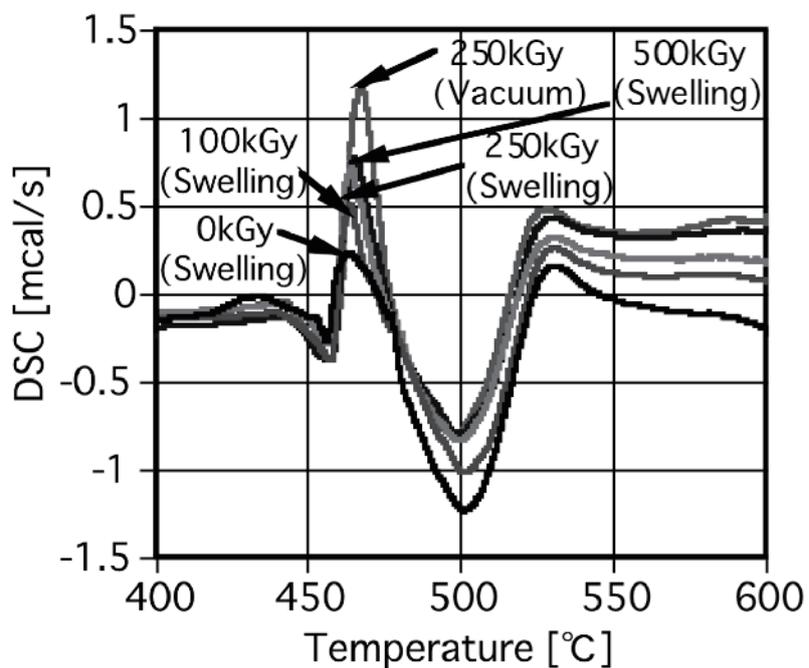
Figure 3.12-4 DSC curves of AFLAS SF under helium atmosphere
