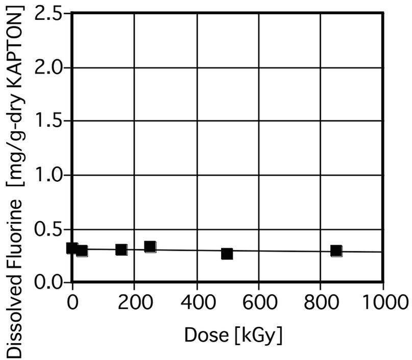
Figure 3.9-2 Quantity of dissolved fluorine vs. dose for Kapton 500H irradiated at room temperature
