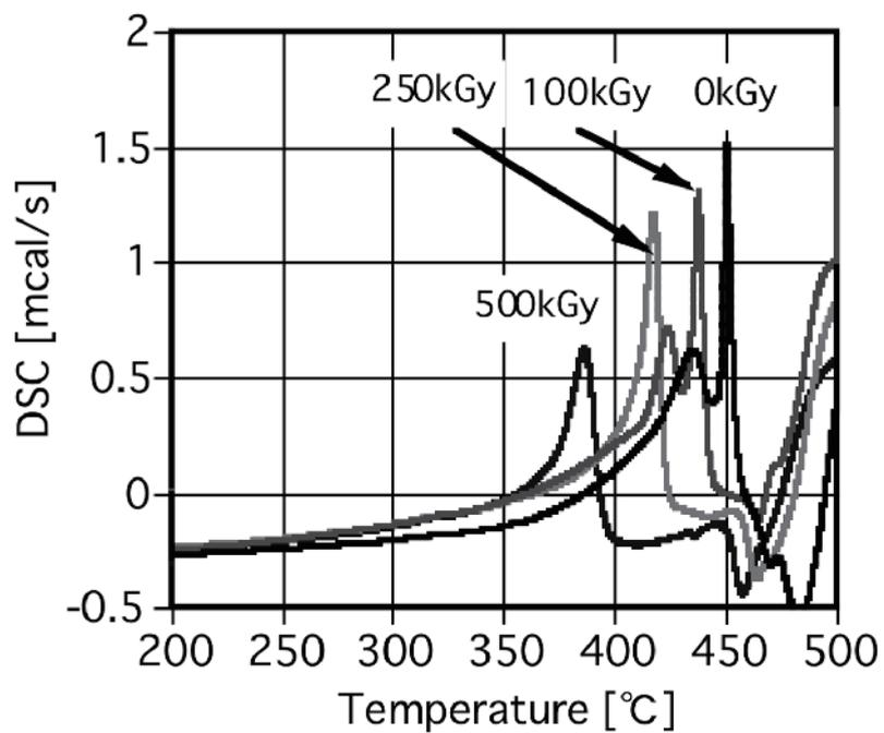
Figure 3.11-3 DSC curves of VITON under helium atmosphere
