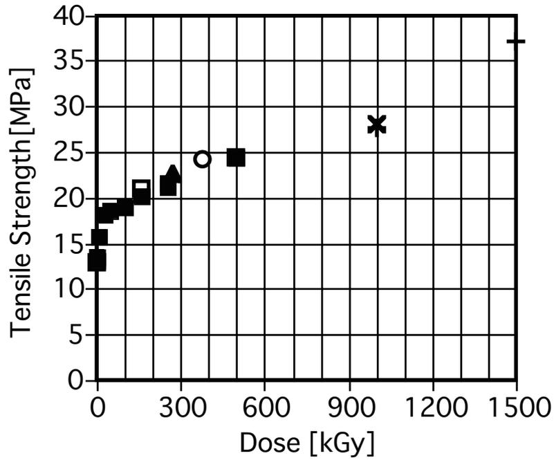
Figure 3.12-1 Tensile strength of AFLAS SF at room temperature
