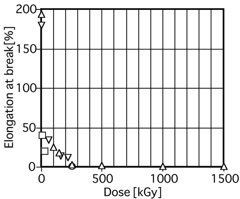
Figure 3.6-2 Elongation at break of  $\gamma$ -irradiated PTFE at room temperature
