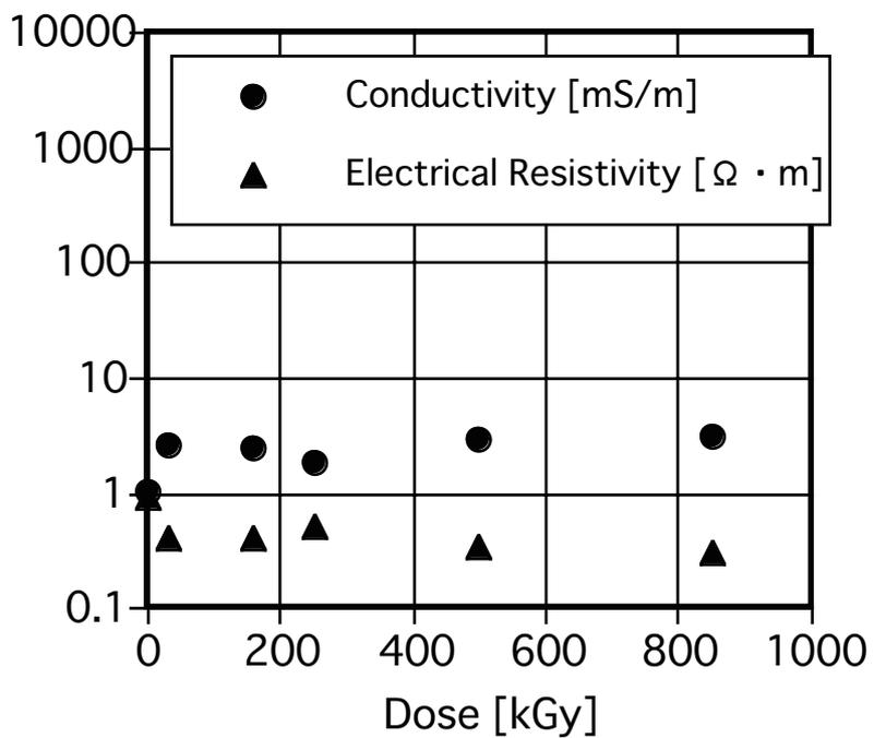
Figure 3.9-3 Conductivity and electrical resistivity of the water after irradiation
