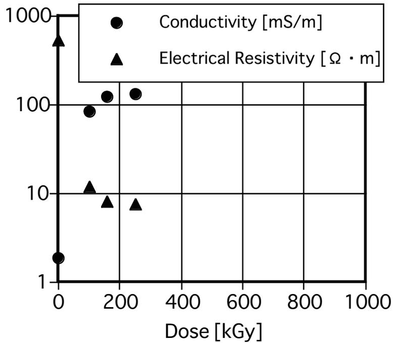
Figure 3.4-3 Conductivity and electrical resistivity of the water after irradiation
