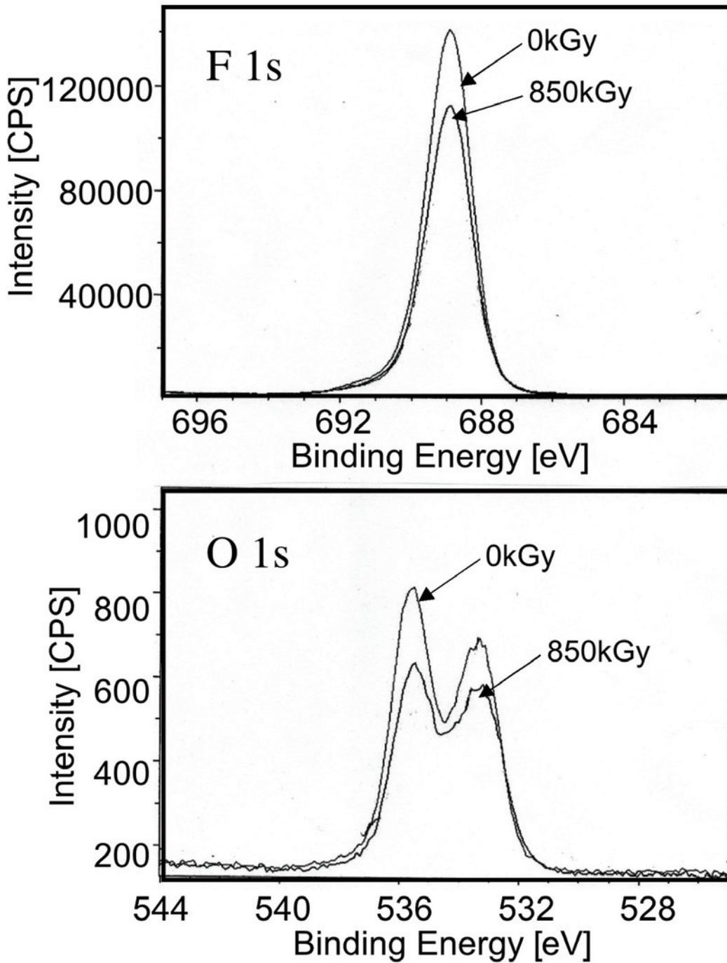
Figures 3.1-11 High resolution spectrums of the F(1s) and O(1s) peaks
