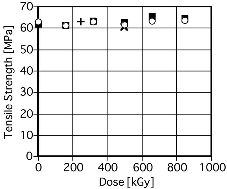
Figure 3.17-1 Tensile strength of Denaturated Polyphenylene Ether at room temperature
