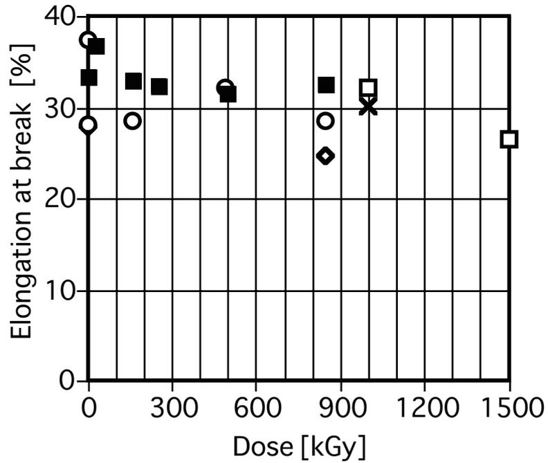
Figure 3.9-1 Elongation at break of Kapton 500H
