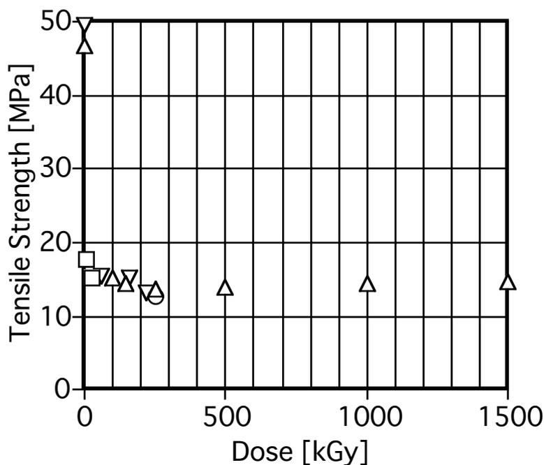
Figure 3.6-1 Tensile strength of  $\gamma$ -irradiated PTFE at room temperature
