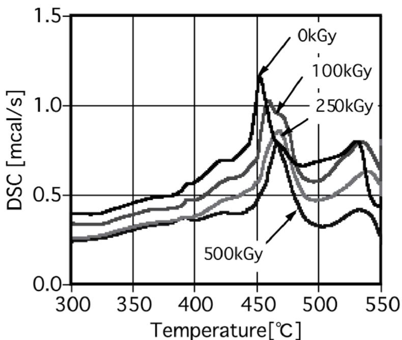
Figure 3.1-8 DSC curves of acid form Nafion N117CS membrane under helium atmosphere
