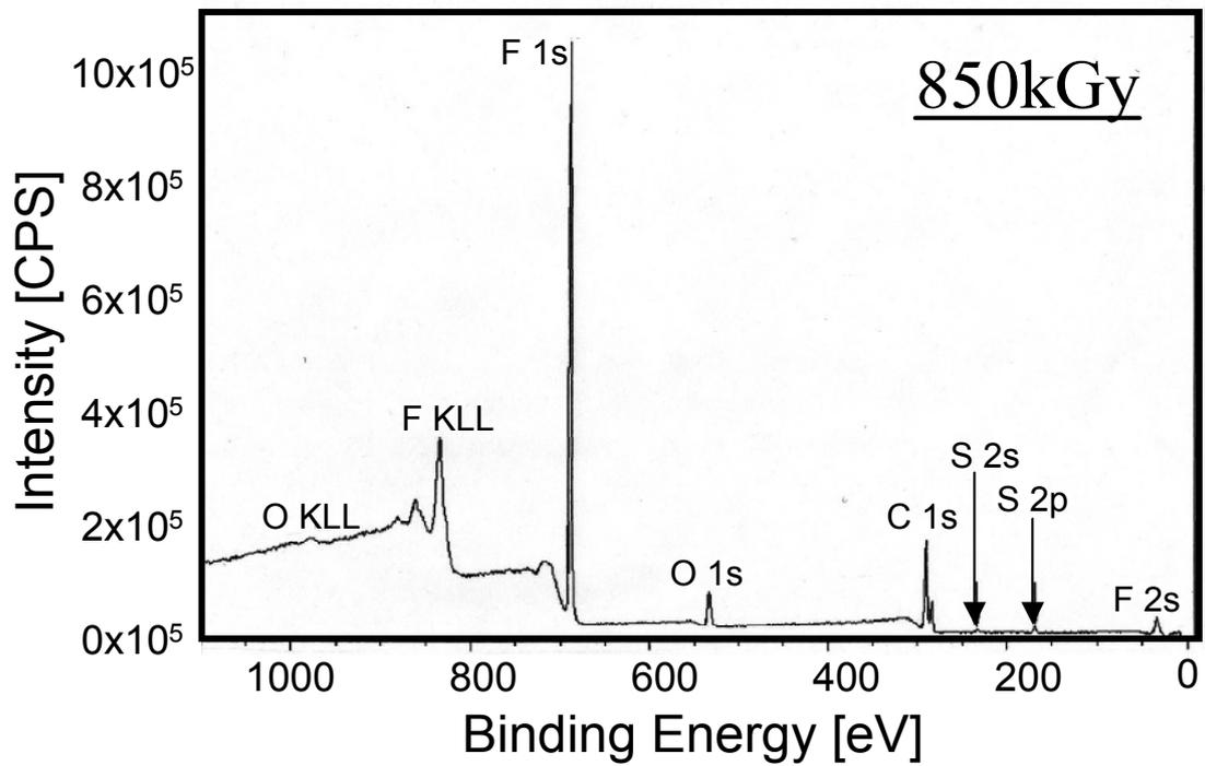
Figures 3.1-9 X-ray photoelectron spectrums of Nafion N117CS membrane
