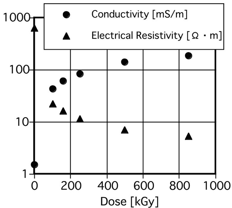
Figure 3.3-2 Conductivity and electrical resistivity of the water after irradiation
