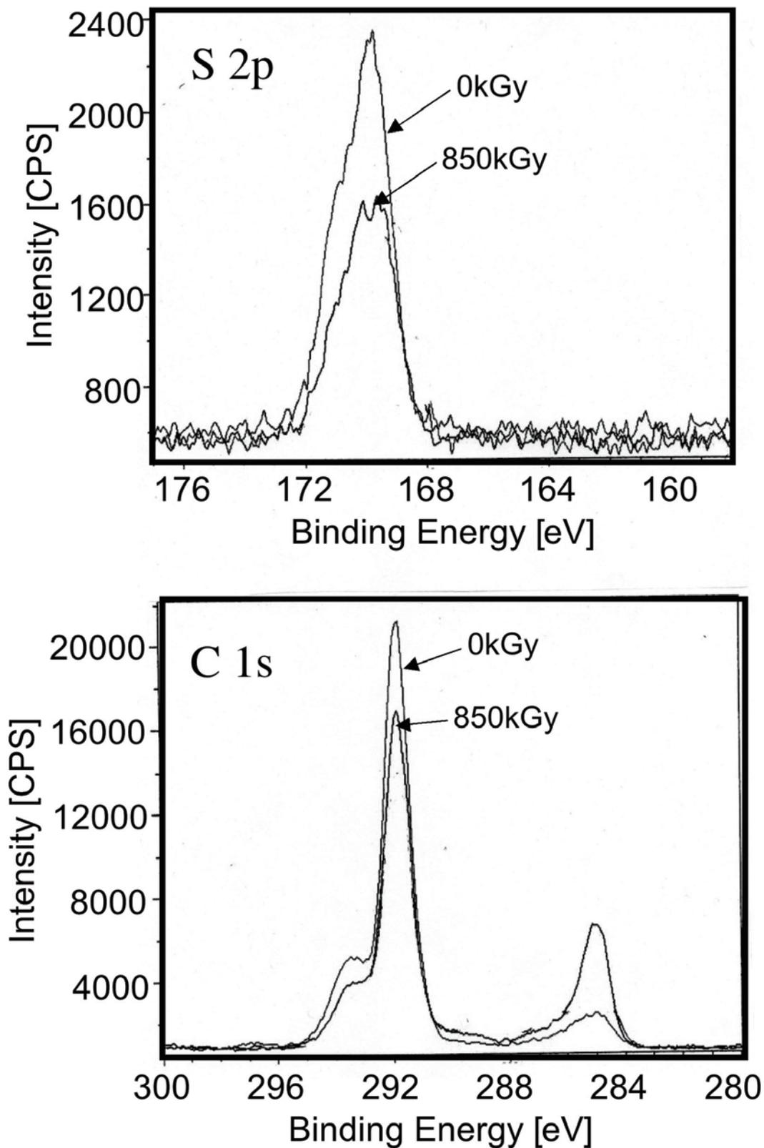
Figures 3.1-10 High resolution spectrums of the S(2p) and C(1s) peaks
