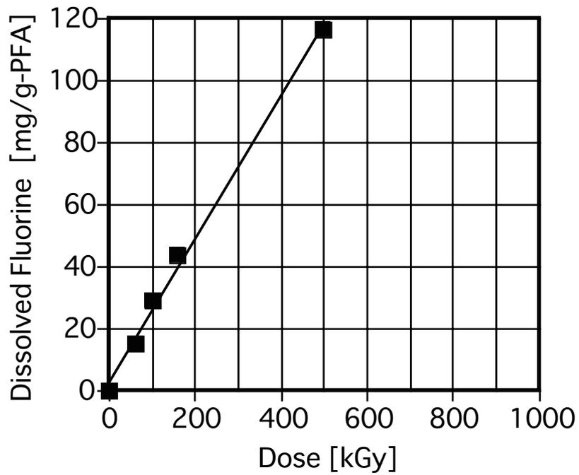
Figure 3.7-3 Quantity of dissolved fluorine vs. dose for PFA 500LP irradiated at room temperature
