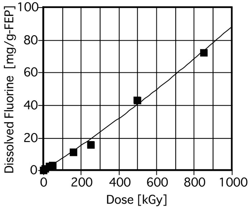
Figure 3.8-2 Quantity of dissolved fluorine vs. dose for FEP 750A irradiated at room temperature
