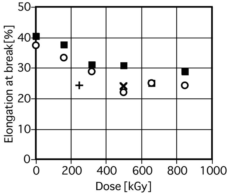
Figure 3.17-2 Elongation at break of Denaturated Polyphenylene Ether at room temperature
