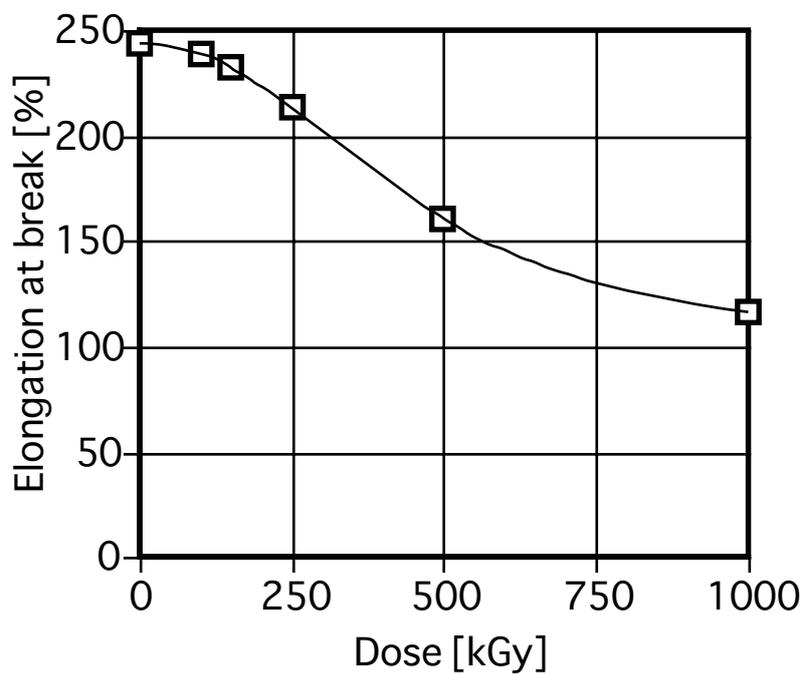
Figure 3.14-2 Elongation at break of EB-irradiated EPDM at room temperature
