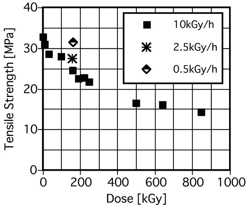
Figure 3.1-2 Effect of dose rate on deterioration in tensile strength
