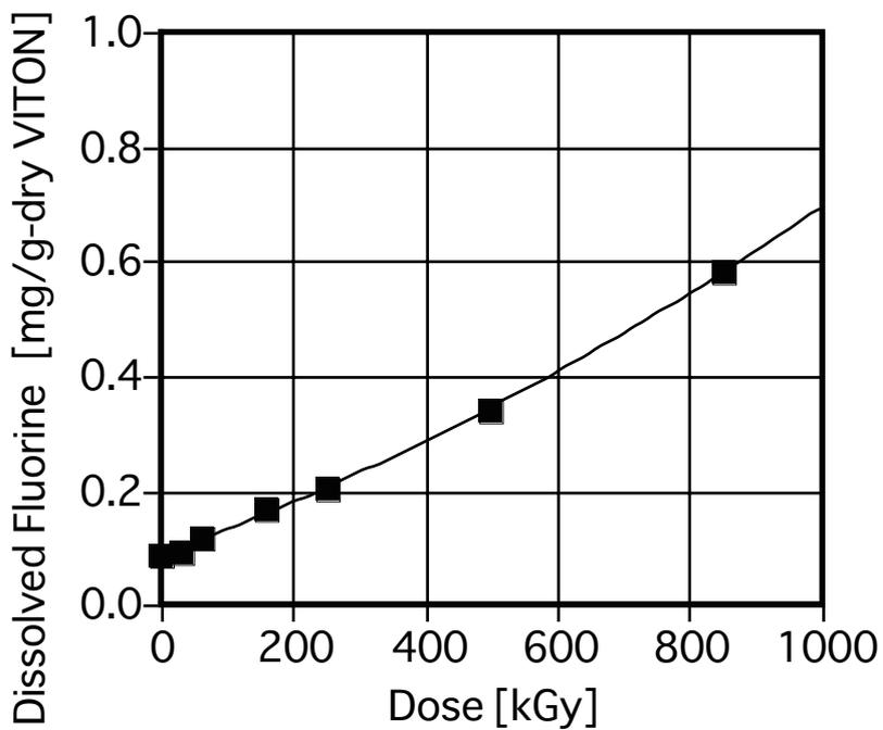
Figure 3.11-2 Quantity of dissolved fluorine vs. dose for VITON irradiated at room temperature
