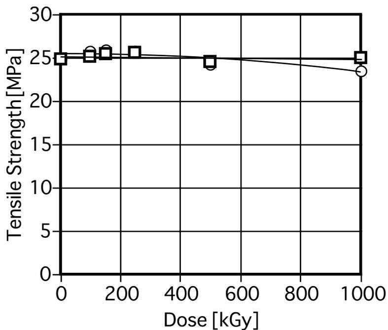
Figure 3.10-1 Tensile strength of EB-irradiated Polyvinyl Chloride HTGA5749 at room temperature
