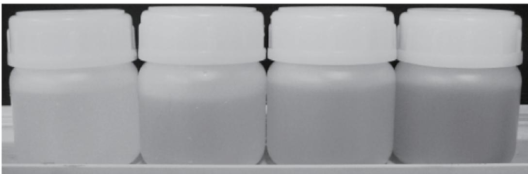
Figure 3.13-2 Coloring of the water after the irradiation of Neoprene with  $\gamma$  - rays
