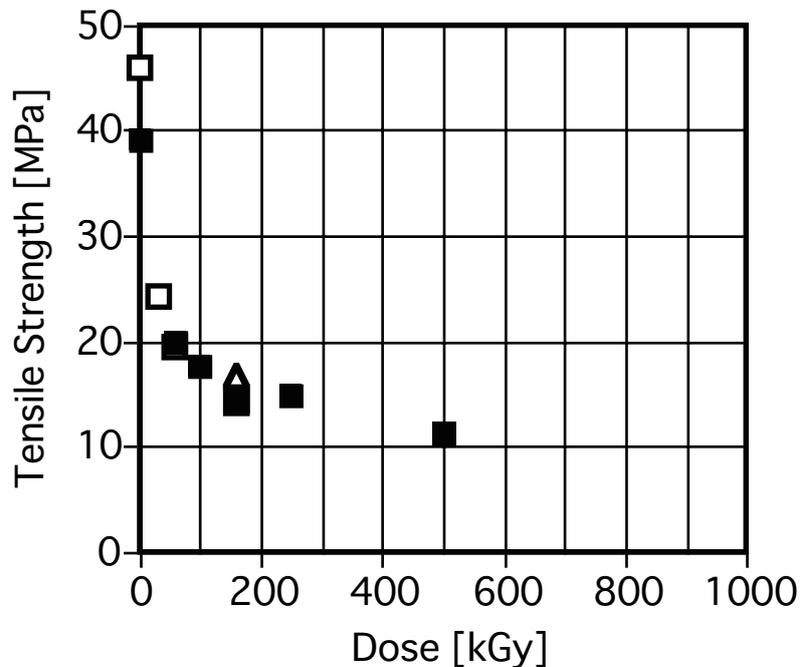
Figure 3.7-1 Tensile strength of  $\gamma$ -irradiated PFA 500LP at room temperature
