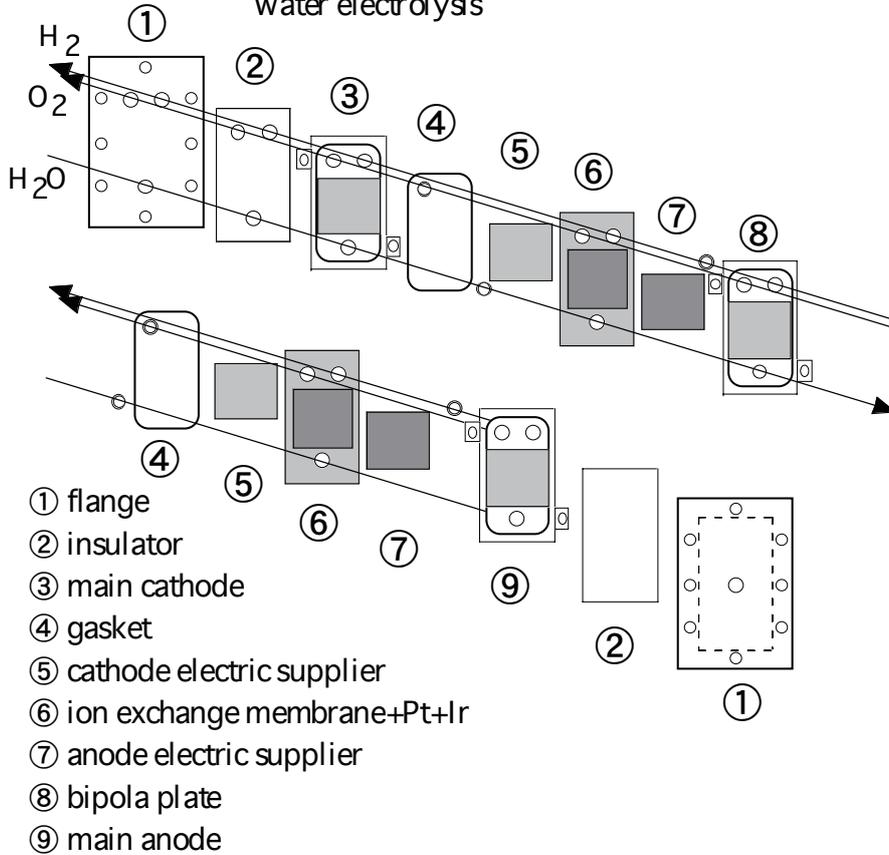
(b) Exploded view of electrolyzer
