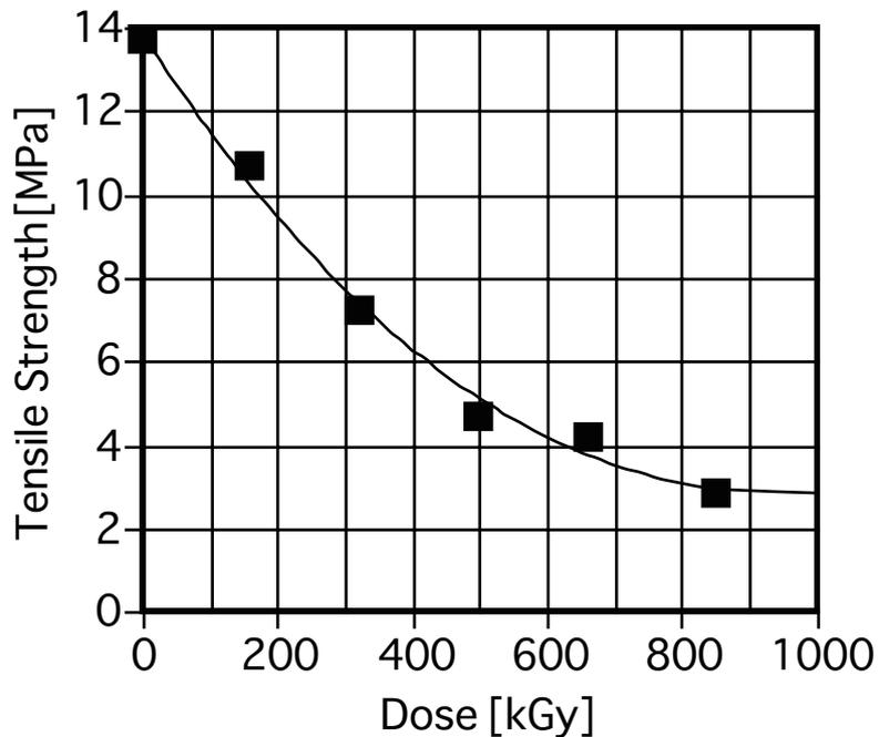
Figure 3.15-1 Tensile strength of  $\gamma$ -irradiated Kalrez at room temperature
