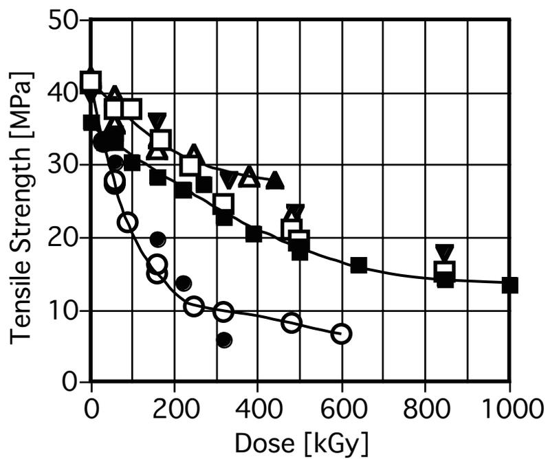
Figure 3.1-1 Tensile strength of  $\gamma$ -irradiated Nafion N117CS at room temperature
