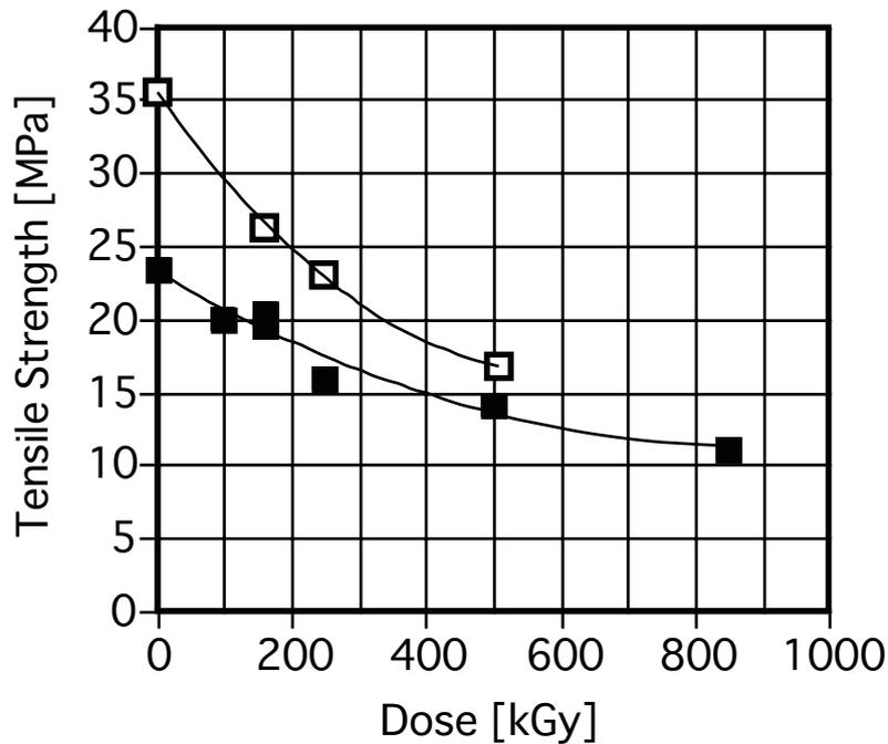
Figure 3.4-1 Tensile strength of  $\gamma$ -irradiated Nafion NE1110 at room temperature
