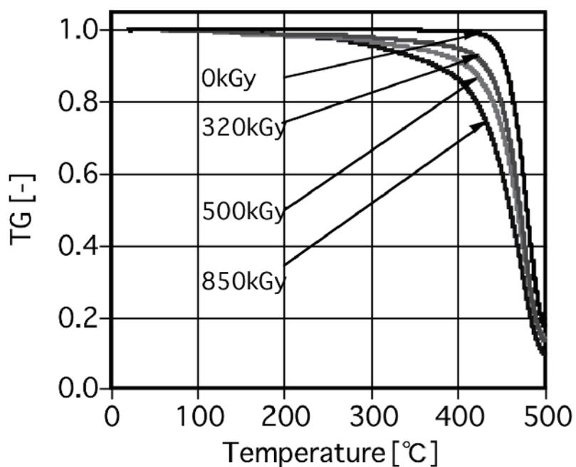
Figure 3.15-5 Weight loss curve vs. temperature of Kalrez under helium atmosphere
