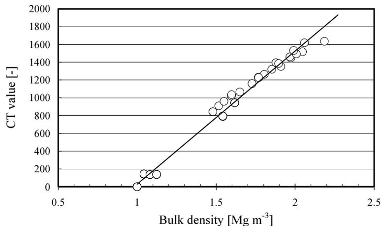
**Figure 3 Relationship between the bulk density and CT value of Kunigel V1 bentonite**
