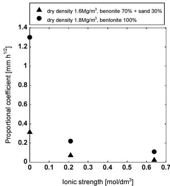
**Figure 9 Relationship between ionic strength and proportional coefficient**
