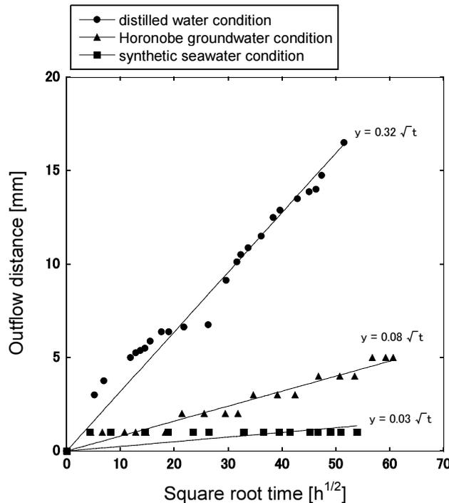
Figure 6 Change of buffer outflow distance with time (dry density of  $1.6 \text{ Mg/m}^3$ )
