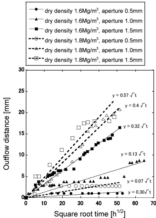
Figure 4 Change of buffer outflow distance with time (sand mixtures ratio 30%)
