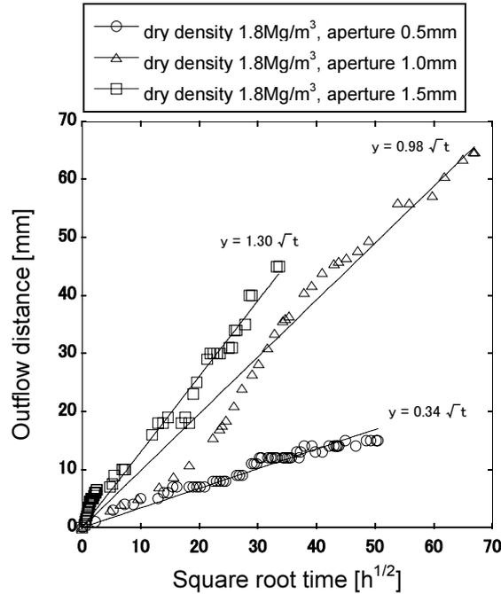
Figure 5 Change of buffer outflow distance with time (sand mixtures ratio 0%)
