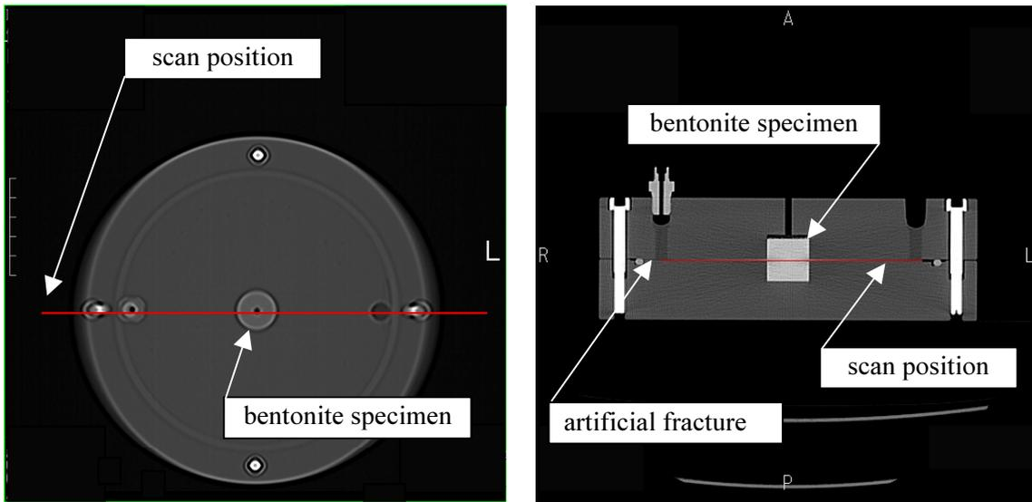
Figure 13 scan position of X-ray CT measurement
