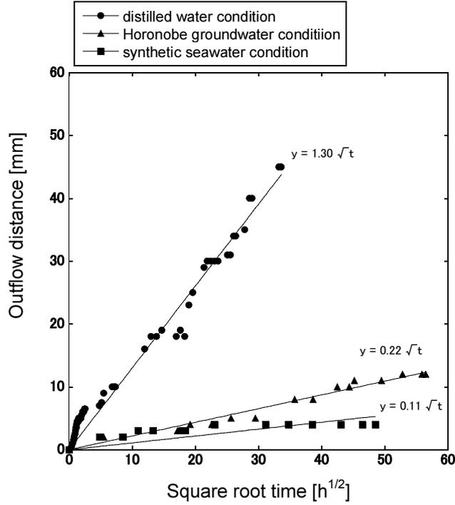
**Figure 7 Change of buffer outflow distance with time (dry density of 1.8 Mg/m<sup>3</sup>)**
