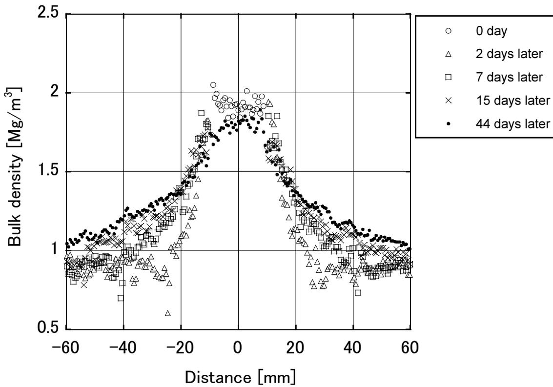
Figure 14 Relationship between outflow distance and density distribution into fracture with time
