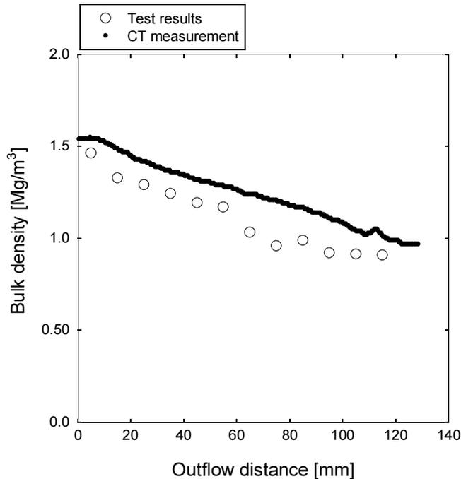
**Figure 12 Comparison of CT measurement and oven-drying method**
