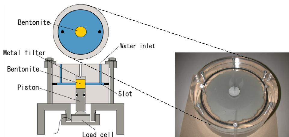
**Figure 1 Test apparatus for buffer extrusion experiment**
