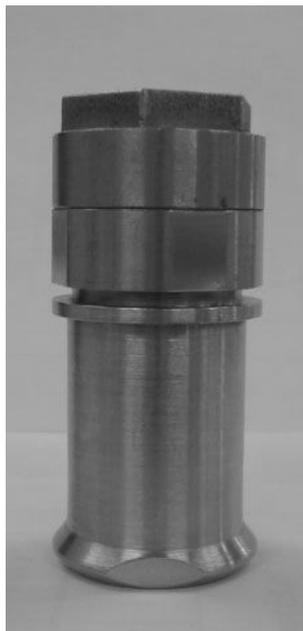
Fig. 3 Source holder, which contains either X1 or X4 capsule.
