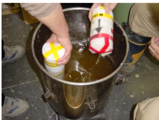
Figure 1: Following sealing in two layers of aluminium-backed plastic and aluminium foil, the core will be sealed in wax until required for squeezing. From Ota et al. 5)
