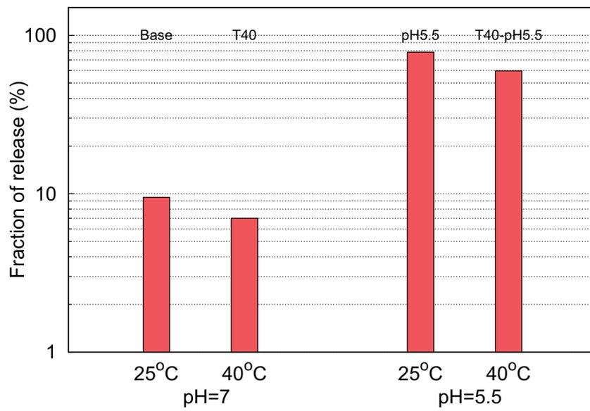
Figure 2.12: Comparison of the final release fractions (total iodine): influence of temperature at pH=7 and 5.5.
