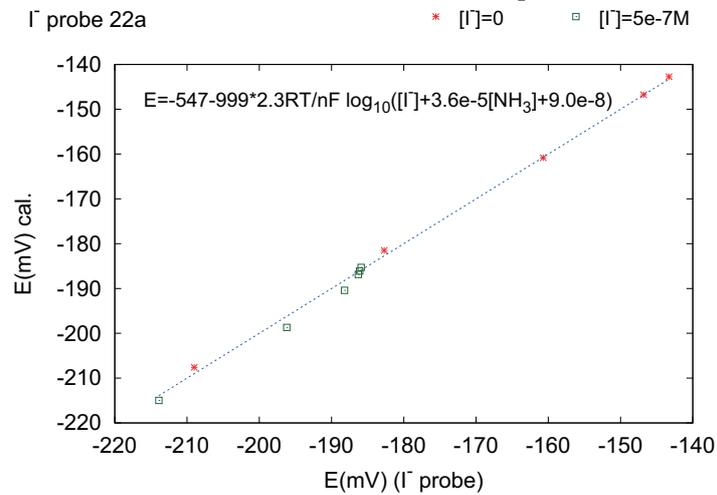
(b) Calibration of the iodide electrode for the compensation of the ammonia influence.
