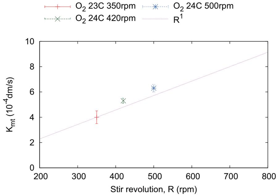
Figure A.5: Dependence of  $K_{mt}$  on the revolution of the stirrer.
