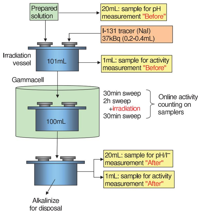
Figure 2.7: Experimental procedure.
