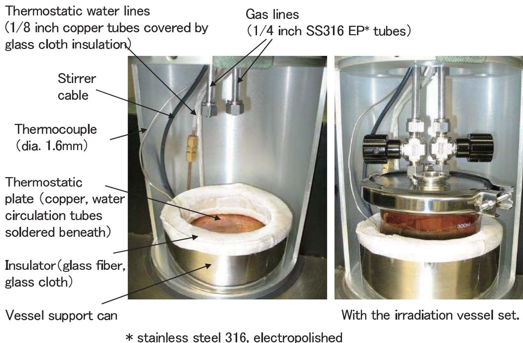
Figure 2.4: Set-up of the irradiation vessel in the irradiator.
