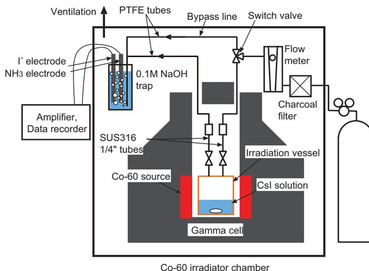
Figure 3.1: Schematic illustration of the experimental system.
