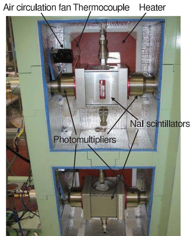
Figure 2.6: On-line counting chamber.
