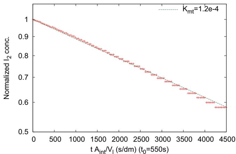
Figure A.4: Evolution of the normalized iodine concentration in the test solution.
