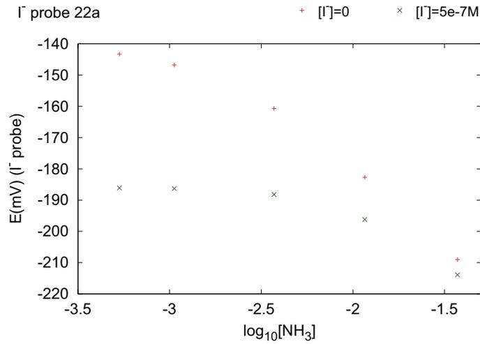
(a) Influence of ammonia on the iodide ion electrode output at low iodide concentrations.
