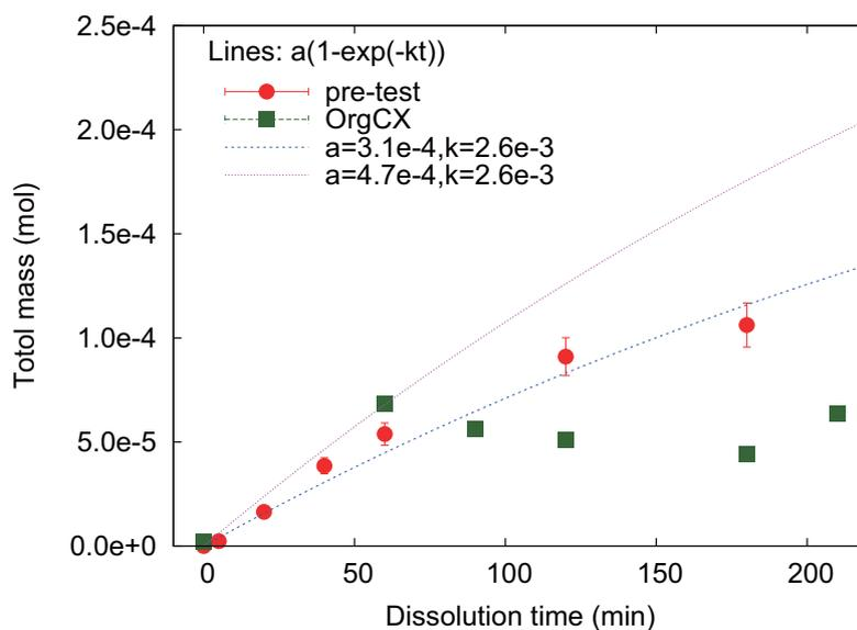
Figure 3.5: Comparison of the xylene mass (mol) evolution in the pre-test (no-irradiation) and the case OrgCX (irradiation 60–180 min: time from the immersion of the PTFE chip).
