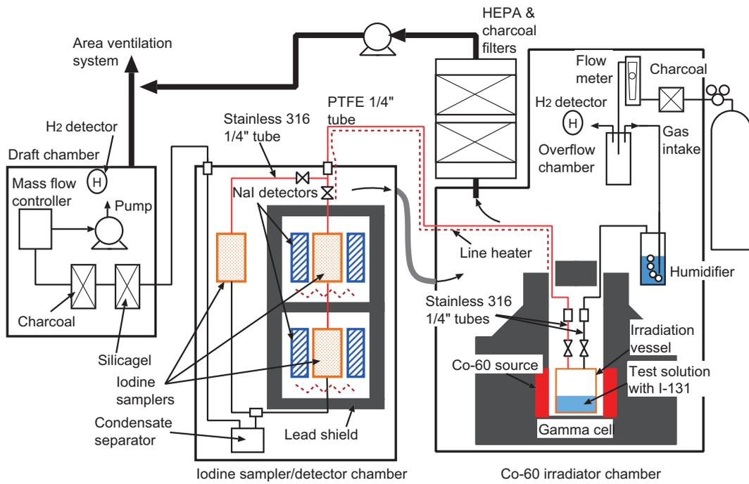
Figure 2.1: Schematic illustration of the experimental system.
