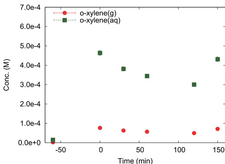
Figure 3.4: Evolution of the o-xylene concentration: OrgCX (irradiation 0–120 min).
