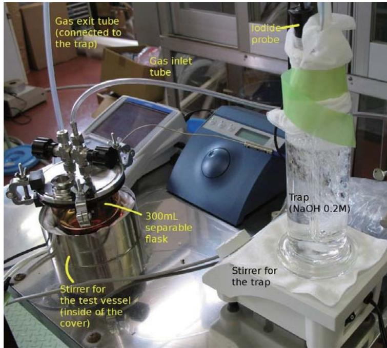
Figure A.2: Measurement of the interface mass transfer coefficient with iodine.
