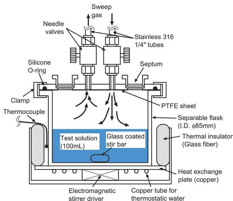
Figure 2.3: Irradiation vessel.
