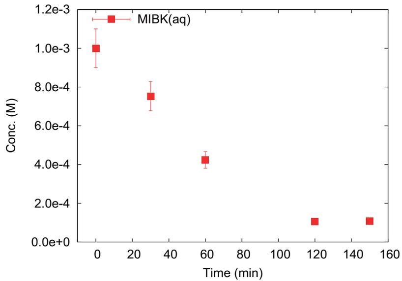
Figure 3.7: Evolution of the MIBK concentration: OrgCM (irradiation 0–120 min).
