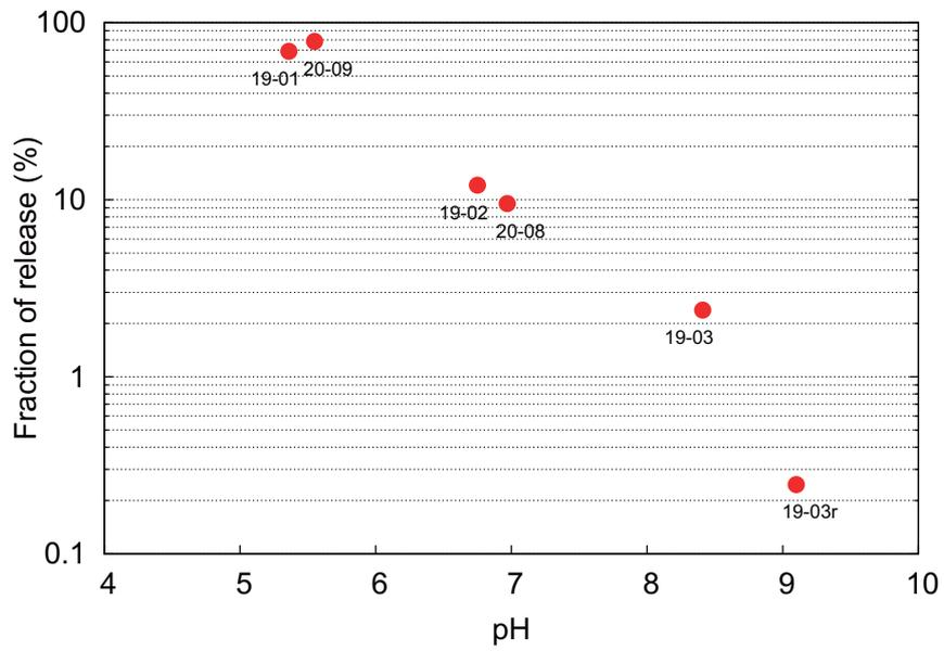
Figure 2.10: Comparison of the final release fractions (total iodine): pH dependence.
