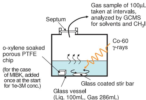
Figure 3.3: Schematic illustration of the xylene-MIBK comparison experiment.
