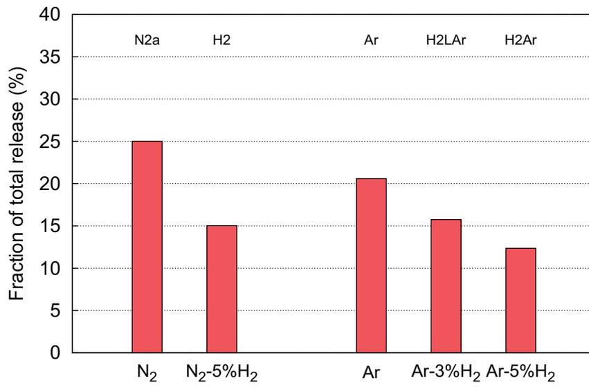
Figure 2.20: Comparison of the final release fractions (total iodine): influence of hydrogen.
