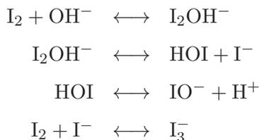
At the pH of the trap solution ( $\sim 13$ ), practically,  $I_2$  produces the same amount of  $I^-$ . Then, monitoring  $I^-$  concentration in the trap is equivalent to monitoring  $I_2$  coming out of the test solution. An ion selective electrode (ISE) for iodide (9653, Thermo) was inserted into the trap to monitor the  $I^-$  concentration there.
