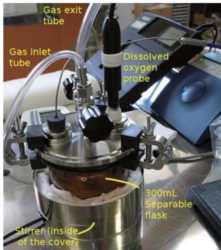
Figure A.1: Measurement of the interface mass transfer coefficient with oxygen.
