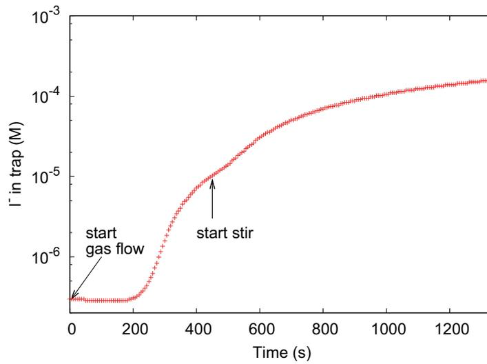
Figure A.3: Evolution of the iodide ion concentration in the trap.
