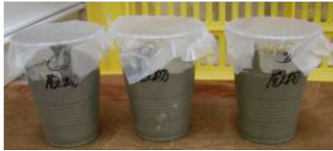
Photo 2-7 Cement composites included sludge from neutralization
