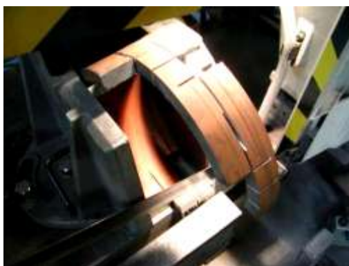
Photo 2-3 Cutting cylindrical carbon steel
