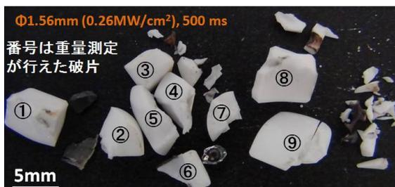
Fig. 32 Appearance of alumina (Laser irradiation time is 500 ms) after crushing test
