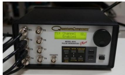
Fig. 15 Digital delay pulse generator
