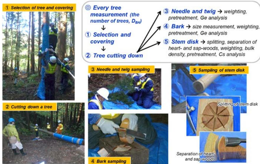
Fig. 2.3-5 Sampling of the tree by cutting down.
