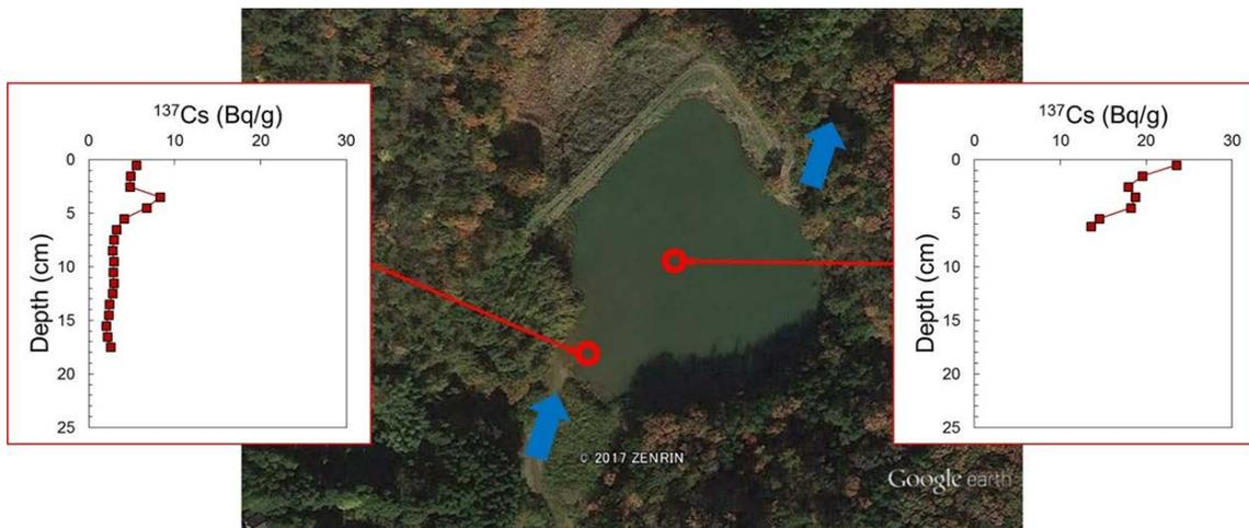
**Fig. 6.5-9** Depth distribution of  $^{137}\text{Cs}$  concentration at the bottom sediment of Shirasago reservoir (left: inflow part, right: center of the lake).
