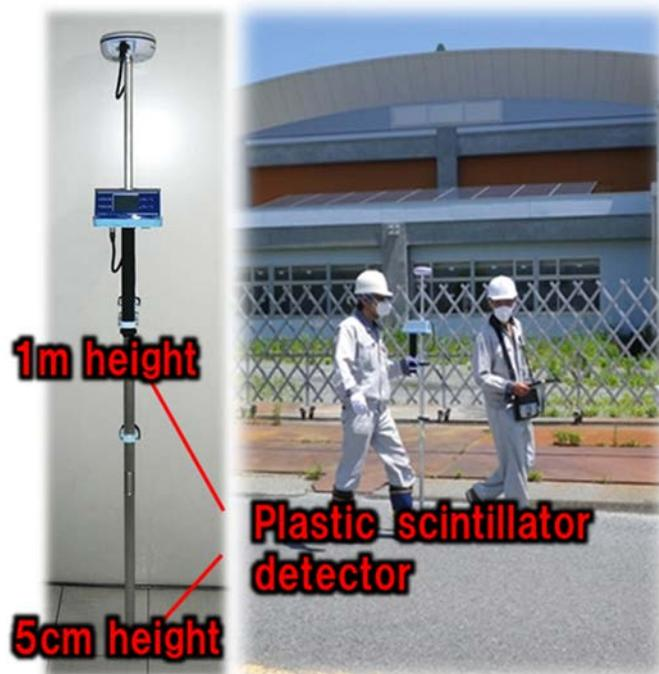
Fig. 2.4-4 Measurement situation using a gamma plotter (GP) (right) and the detector (left).
