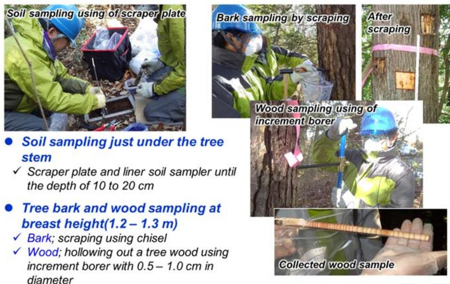
Fig. 2.3-6 Method for sampling of soil and the tree.
