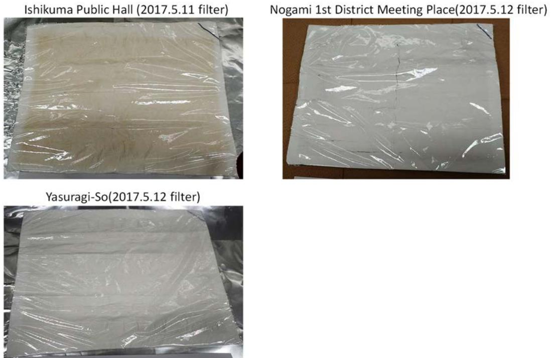
**Fig. 6.2-5 Photographs of filters after sampling the atmospheric suspended dust.**
