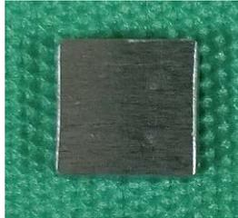
Fig.1 Pure Cr specimen after cut in 2.0 × 10 × 10 mm
