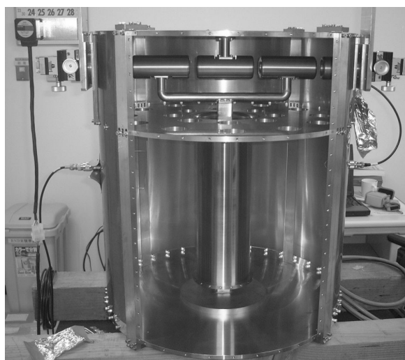
Fig. 3. Cold model of the bunchers to transport RNBs from TRIAC facility to JAEA superconducting booster.
