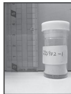
Phot.1 Blast furnace Slag
