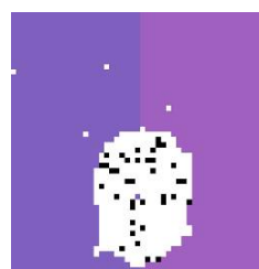
Fig 1. A lenticular bubble on a grain boundary indicated by a vertical line for 10000 Monte-Carlo steps.
