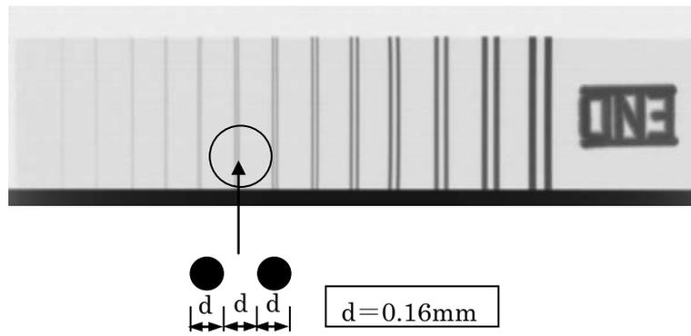
Figure 6 Resolution performance test
