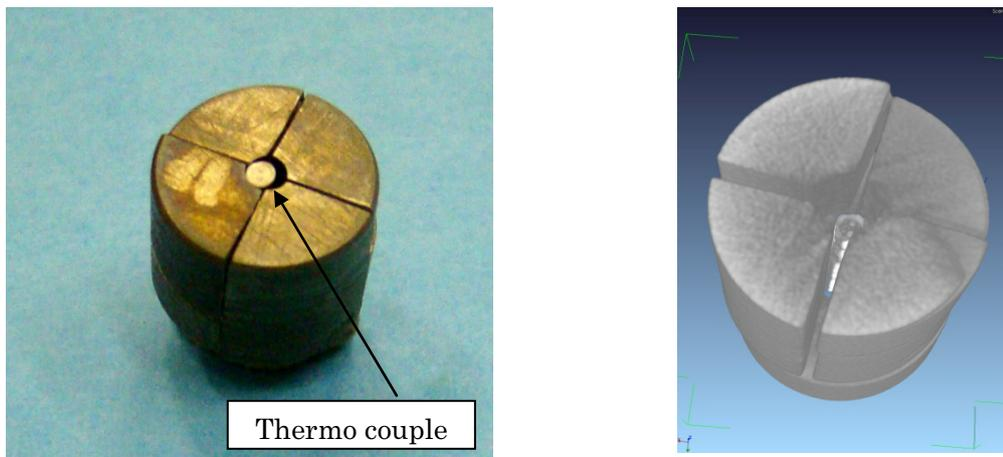
Figure 5 The imitated pellet and a measured 3D graphic
