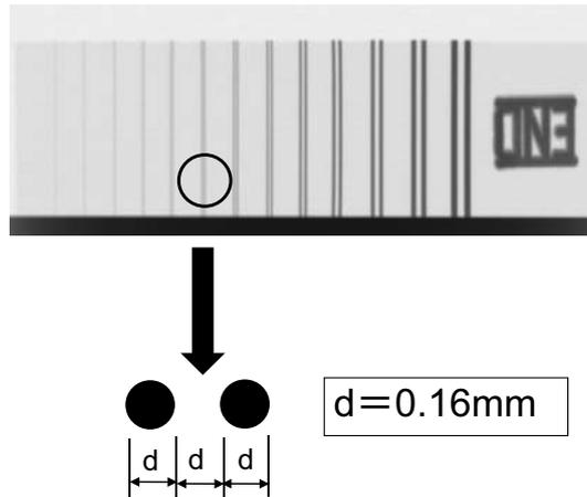
The resolution tests using platinum double wire were performed.
