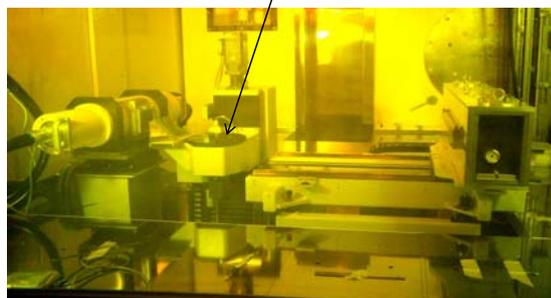
Specimen movement unit has a rotatable specimen table which can move to the vertical direction.
