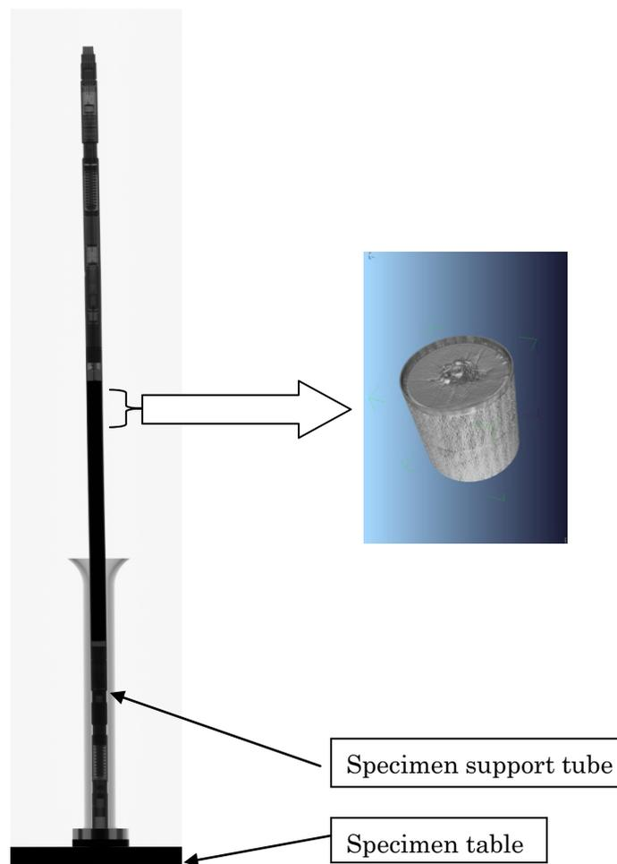
Figure 7 Transmission X-ray graphics of a fuel rod
