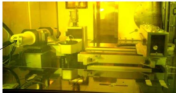
X-ray generator unit consists of high voltage generator unit and x-ray source tube.
