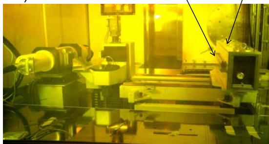
X-ray detector unit is possible to change the distance from X-ray source tube.
