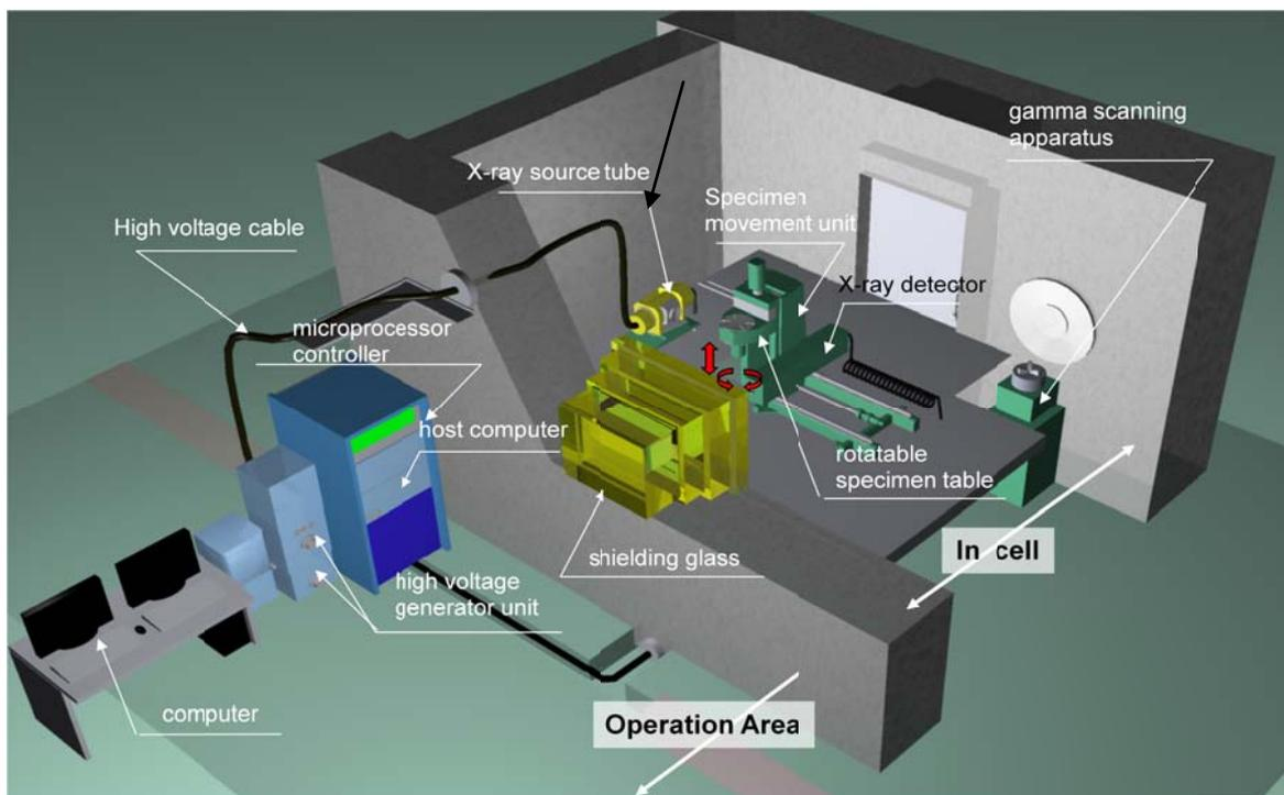
Figure 2 Schematic drawing of the X-ray CT inspection system
