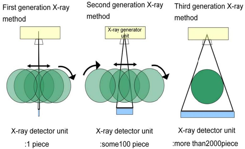
Figure 3 Various scanning methods
