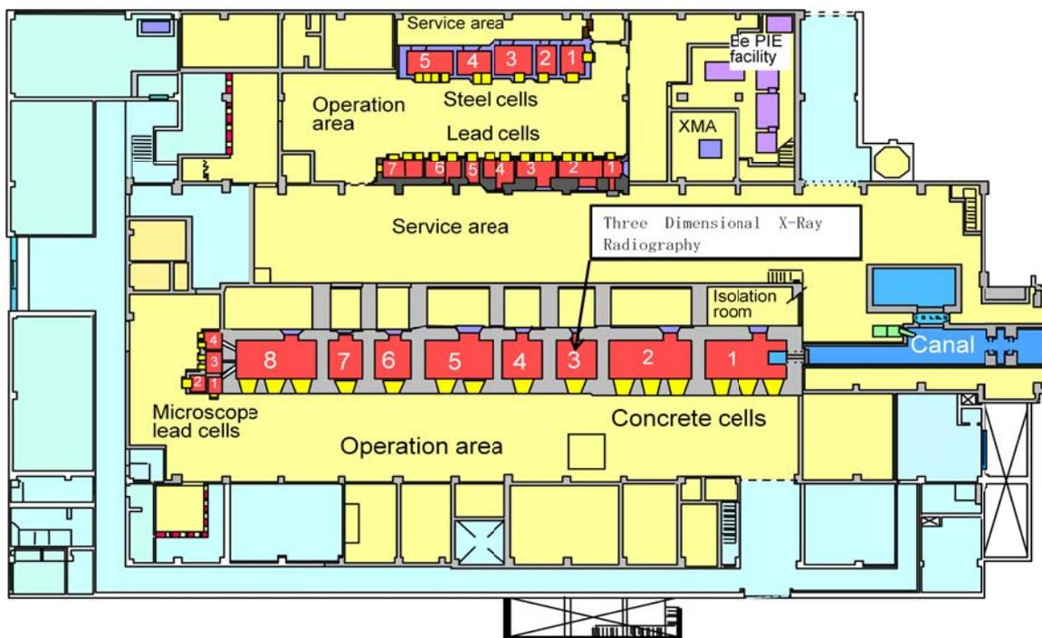
Figure 1 Arrangement of the hot laboratory
