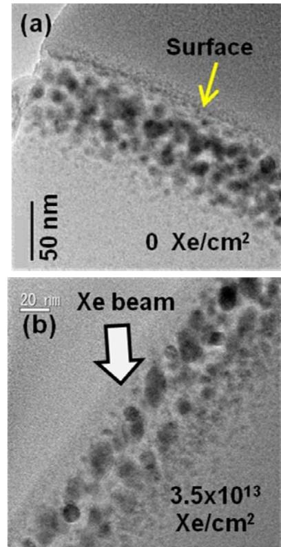
Fig. 2 Cross-sectional TEM images of Zn NPs in silica glass in (a) unirradiated state and after (b) irradiation of 200 MeV  $\text{Xe}^+$  ions to a fluence of  $3.5 \times 10^{13} \text{ Xe}/\text{cm}^2$ . As indicated by an arrow in (b), the sample was irradiated with an incident angle of 45 deg from the surface normal.
