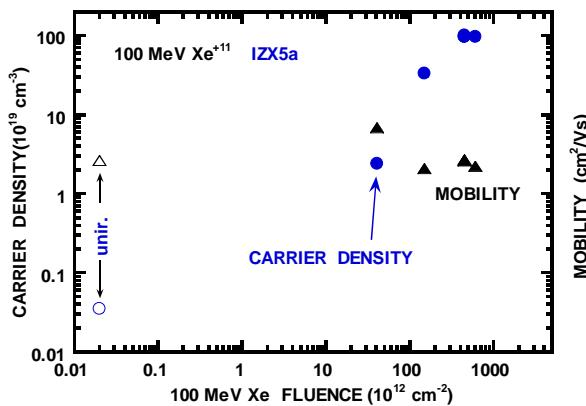
Fig. 2 Carrier density ( $\bullet$ ) and mobility ( $\blacktriangle$ ) of IZO films vs 100 MeV  $\text{Xe}^{+11}$  ion fluence. Open symbols ( $\circ$ ,  $\triangle$ ) indicate carrier density and mobility of unirradiated film.
