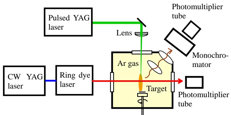
Fig. 1 Setup of the laser-ablation laser spectroscopy.
