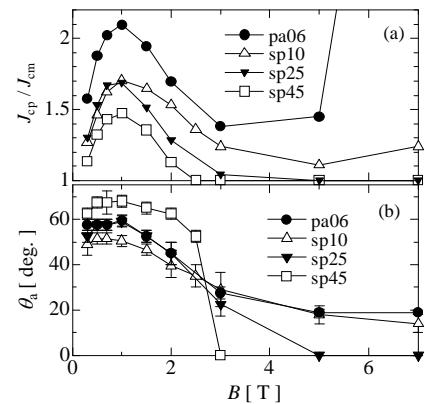
Fig. 2 Magnetic field dependence of (a)  $J_{cp}/J_{cm}$  and (b)  $\theta_a$  at 77.3 K.
