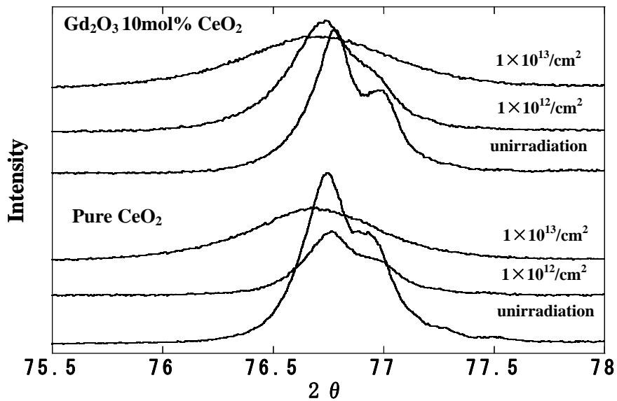
Fig. 1 XRD spectra around (331) of undoped  $\text{CeO}_2$  and those doped with 10 mol%  $\text{Gd}_2\text{O}_3$  for various ion-fluences.
