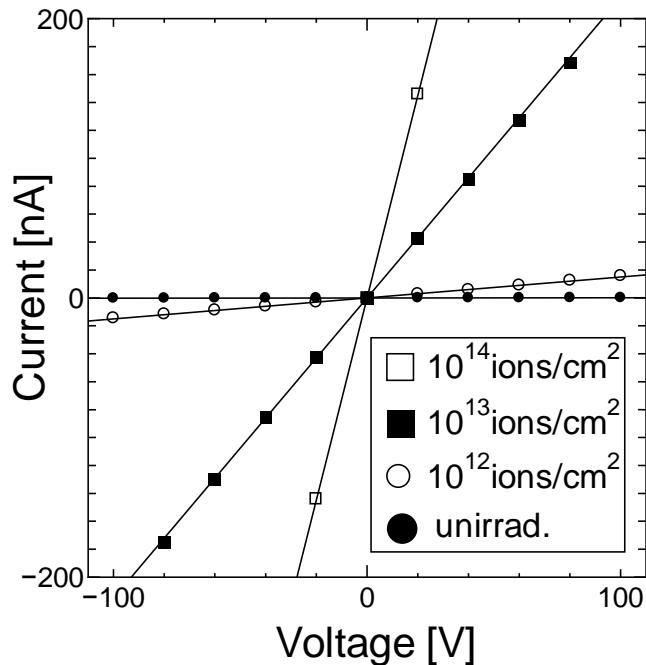
Fig. 1 Current-Voltage characteristics observed for a CeO<sub>2</sub> thin film before and after the irradiation with 120MeV Xe ions. The solid lines are the results of linear fitting of the data in the voltage range from -100V to 100V.
