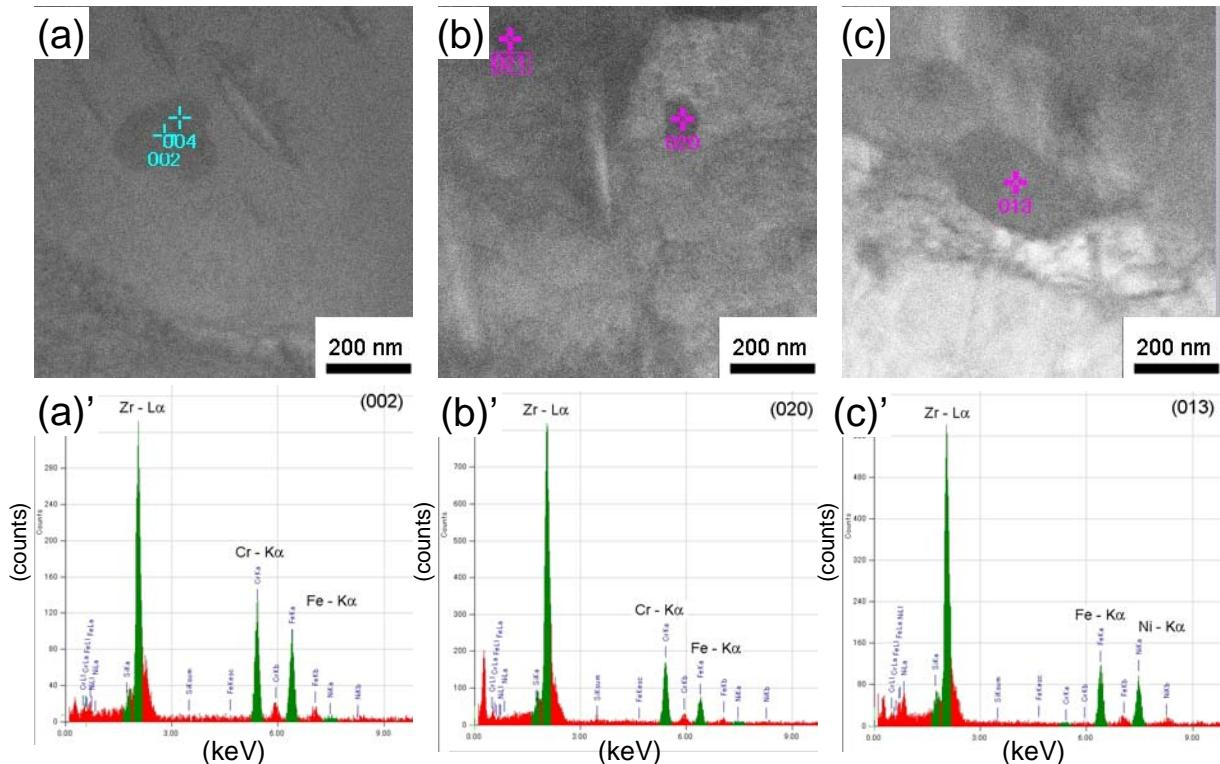
Fig.1 Typical microstructure of Zircaloy-2 irradiated with 210 MeV Xe ions to a fluence of  $5 \times 10^{15}$  ions/cm<sup>2</sup> at room temperature, and (a)' to (c)' indicates the EDS spectrum at the position of “002”, “020” and “013” in (a) to (c), respectively. The precipitate of (a) and (b) is the metal precipitates of (Fe, Cr) base and (c) is the precipitate of (Fe, Ni) base.
