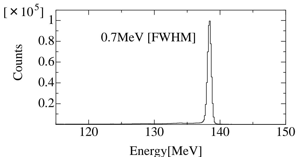
Fig. 2 Energy spectrum of the  $^{16}\text{O} + ^{197}\text{Au}$  elastic scattering. This spectrum was obtained by the sum of energies of a  $\Delta E$  detector and the second annular lane (from the inside) of the  $E$  detector.
