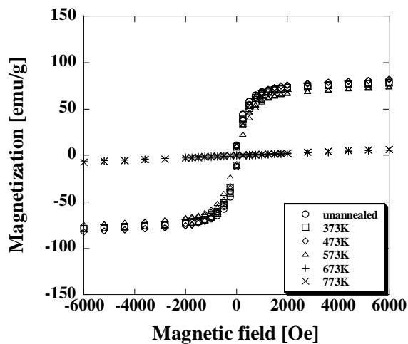
Fig. 2 Irradiation induced magnetic moment at 20K as a function of applied magnetic field for Fe-50at.%Rh irradiated with 200MeV Au to the ion-fluence of  $5 \times 10^{13}/\text{cm}^2$ .
