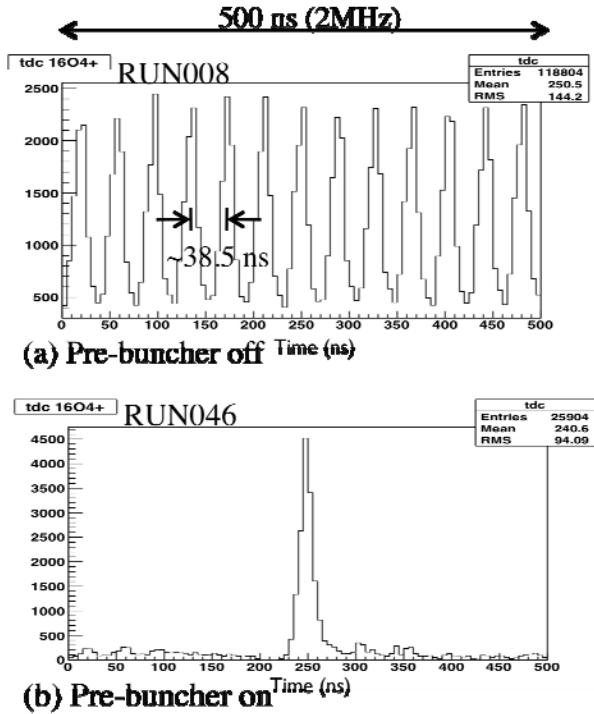
Fig. 1 Beam bunch structure with pre-buncher off (a) and pre-buncher on (b).
