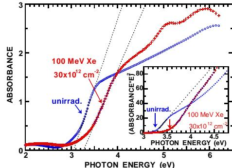
Fig. 2 Optical absorption spectra of unirradiated IZO film and the film irradiated with 100 MeV  $\text{Xe}^{+11}$  at  $3 \times 10^{13} \text{ cm}^{-2}$ . Dotted lines indicate the absorption-edge slope. The inset shows the square of absorbance times photon energy ( $E$ ) vs  $E$ , illustrating the band gap ( $E_g$ ) indicated by vertical lines ( $E_g = 3.239$  and  $3.546 \text{ eV}$  before and after the ion impact).
