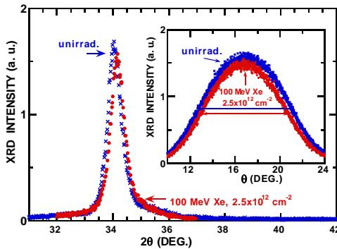
Fig. 1 XRD patterns and rocking curves (inset) before and after 100 MeV  $\text{Xe}^{+11}$  ion impact at  $2.5 \times 10^{12} \text{ cm}^{-2}$ . The peak at  $\sim 34^\circ$  corresponds to ZnO (002) diffraction peak (i.e., c-axis orientation),  $\sim 31^\circ$  and  $32.6^\circ$  ( $\text{In}_2\text{O}_3$ ), and  $33^\circ$  (In) were not observed. In the inset, horizontal lines indicate the full-width at half-maximum (8.45 and 7.83 ° before and after the ion impact).
