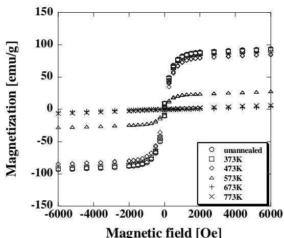
Fig. 1 Irradiation induced magnetic moment at 20K as a function of applied magnetic field for Fe-50at.%Rh irradiated with 200MeV Au to the ion-fluence of  $1 \times 10^{13}/\text{cm}^2$ .
