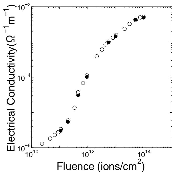
Fig. 2 Fluence dependence of electrical conductivity for a CeO<sub>2</sub> thin film irradiated with 120MeV Xe ions. The solid circles are the values measured based on linear fitting of current-voltage relations. The open circles are the values measured based on the current value at applied voltage of 100V.
