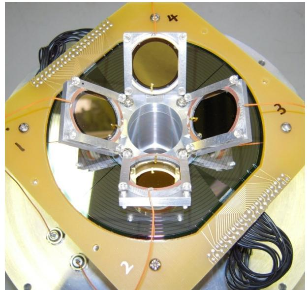
Fig. 1 Si  $\Delta E-E$  telescope consisting of an annular-type  $E$  detector and four  $\Delta E$  detectors.
