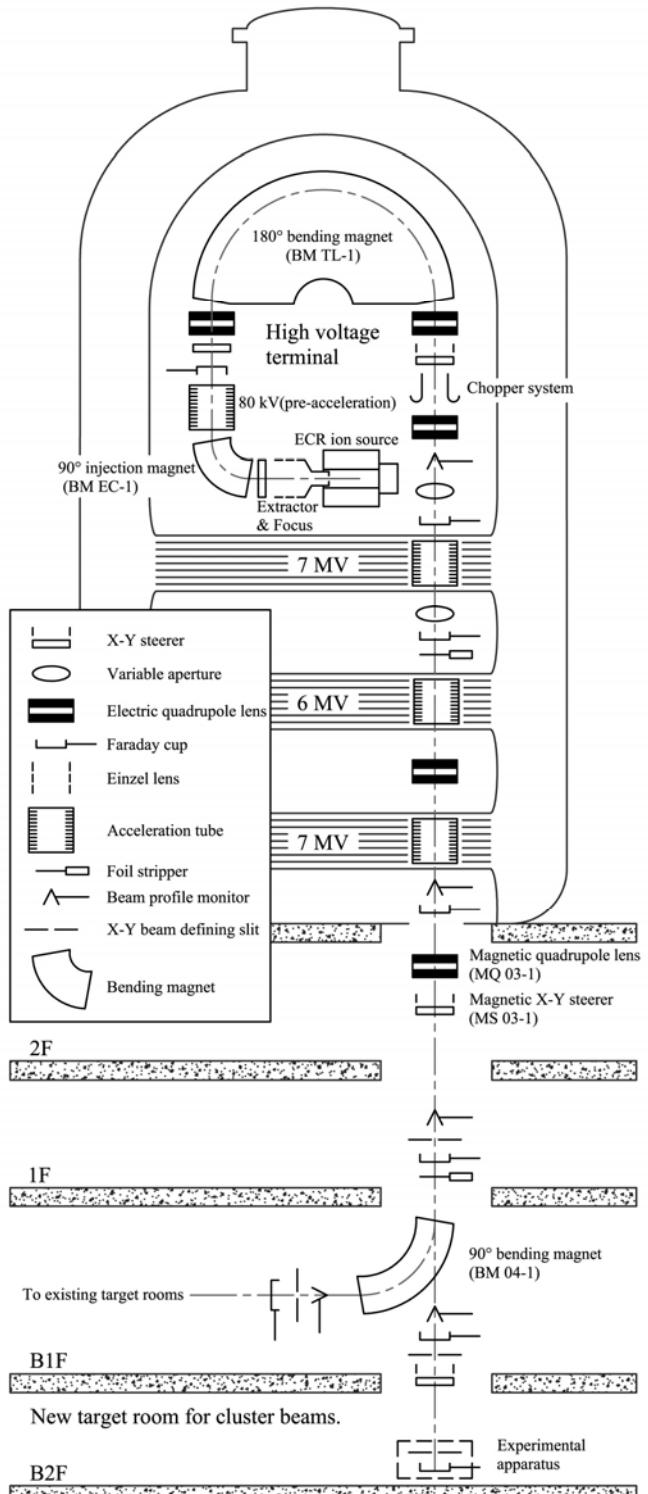
Fig. 1 Schematic diagram of the accelerator
