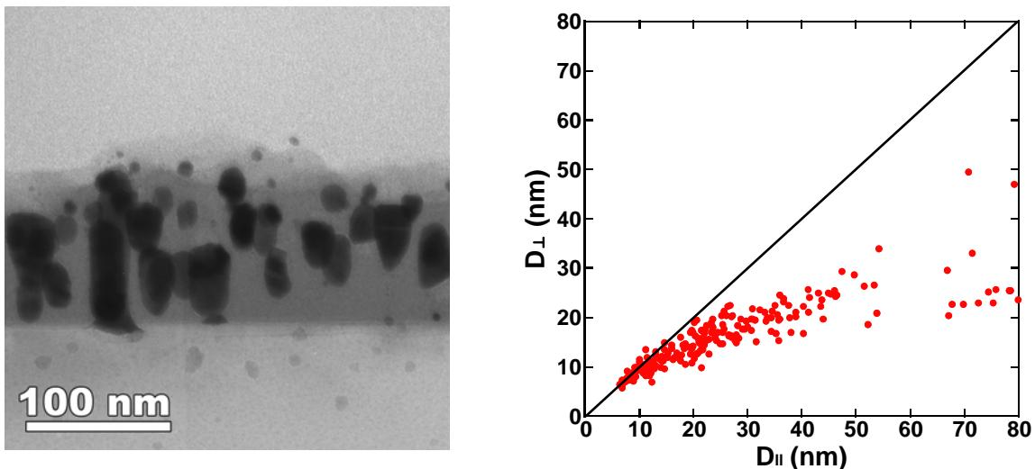
Fig. 2 Bright-field cross section view of the thin film specimen irradiated at ambient temperature with 210 MeV Xe ions to a fluence of  $1 \times 10^{18}$  ions/m<sup>2</sup> (a). The direction of ion irradiation was perpendicular to the film thickness direction. Size distribution of Au nanoparticles as functions of diameters measured parallel and perpendicular to the direction to film thickness or ion beam direction (b).
