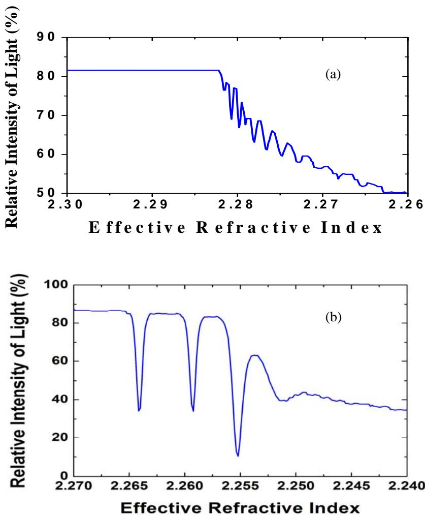
Fig. 1 Prism-coupling results for (a) GLSO glass (b) Nd:MgO:LiNbO<sub>3</sub>
