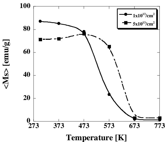
Fig. 3 Average values of saturation magnetization,  $\langle M_s \rangle$ , for the region expect around the ion range, as a annealing temperaturte.
