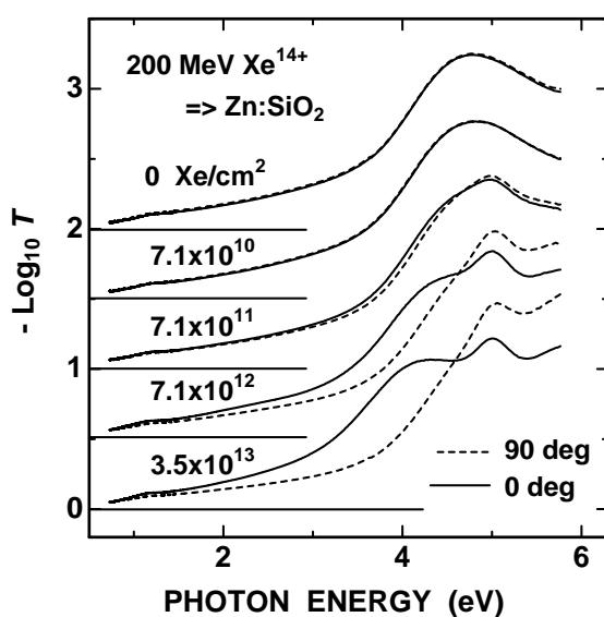
Fig. 1 Optical density spectra of Zn NPs in silica glass in unirradiated state and after irradiation of 200 MeV  $\text{Xe}^{14+}$  ions to four different fluences. Linearly polarized light with the polarization of 0 and 90 deg was used. The spectra are vertically shifted with each other for clarity and the horizontal lines indicate the base lines.
