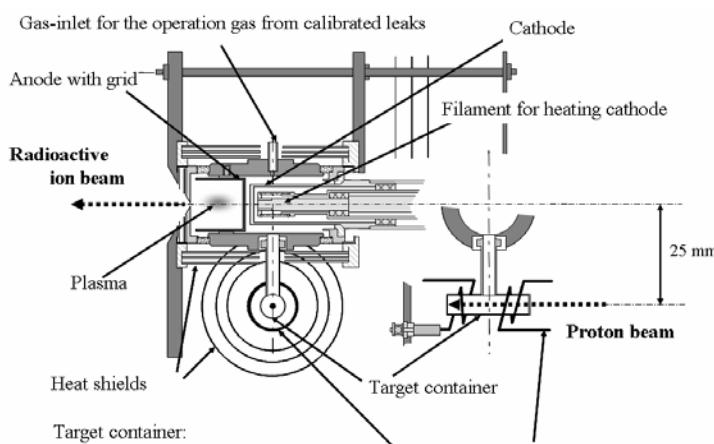
Fig. 1 Schematic view of the new ion source system.
