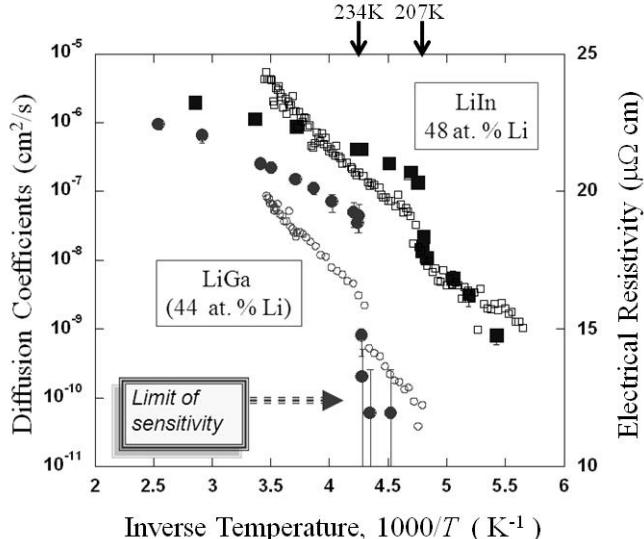
Fig. 1 Temperature-dependence of diffusion coefficients (closed square) and electrical resistivity (open square) for LiIn with 48 at.% Li, and that of diffusion coefficients (closed circle) and electrical resistivity (open circle) for LiGa with 44 at.% Li.
