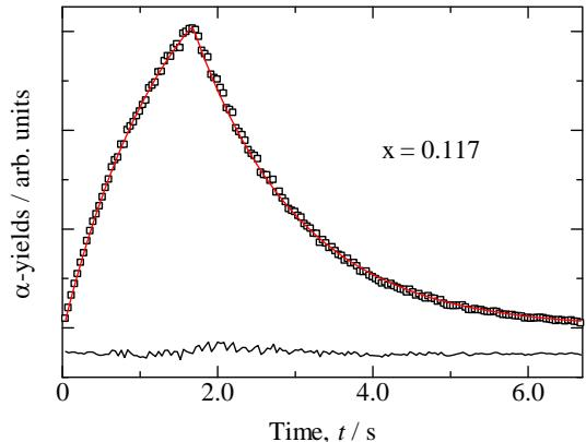
Fig. 2 Time spectrum of the  $\alpha$ -yields for  $\text{La}_{2/3-x}\text{Li}_{3x}\text{TiO}_3$  ( $x = 0.117$ ) measured at 100°C. Rectangles: measured data as Fig. 1, red solid line: calculated and bottom solid line: difference.
