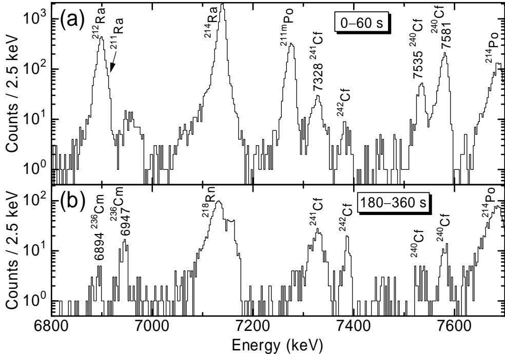
Fig. 1 (a)  $\alpha$ -particle spectrum measured at the first detector station. (b) Sum of  $\alpha$ -particle spectra measured at the 4th, 5th, and 6th detector stations. Ra isotopes and  $^{211\text{m}}\text{Po}$  are produced in the reactions with Pb impurity included in the target.
