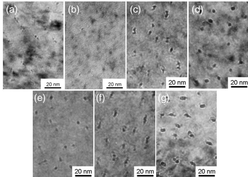
Fig. 1 TEM image of  $\text{UO}_2$  irradiated with (a) 100 MeV  $\text{Xe}^{+25}$ , (b) 100 MeV  $\text{Zr}^{+10}$ , (c) 210 MeV  $\text{Xe}^{+16}$ , (d) 210 MeV  $\text{Xe}^{+29}$ , (e) 150 MeV  $\text{Xe}^{+27}$ , (f) 150 MeV  $\text{Au}^{+27}$ , and (g) 310 MeV  $\text{Au}^{+27+}$  ions to a fluence of  $5 \times 10^{11} \text{ ions/cm}^2$  at room temperature.
