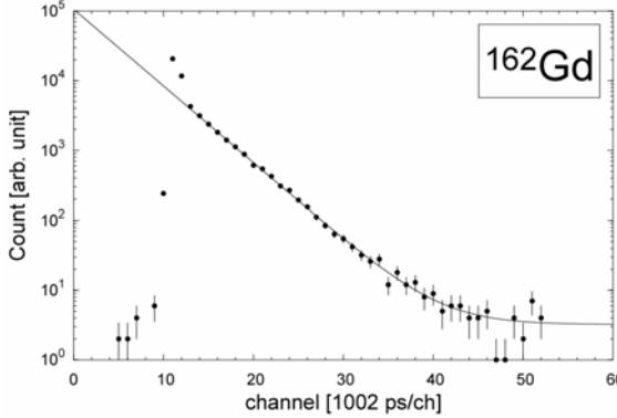
Fig. 2 Time spectrum of  $^{162}\text{Gd}$ . The result of the fitting analysis is shown by a solid curve.
