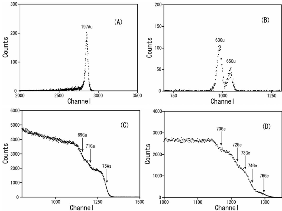
Fig. 3 HIRBS spectra from Au foil (A), Cu foil (B), GaAs crystal (C) and Ge crystal (D).
