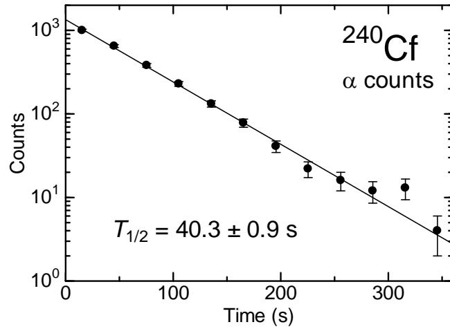
Fig. 2 Decay curve of  $\alpha$  particles of  $^{240}\text{Cf}$ .
