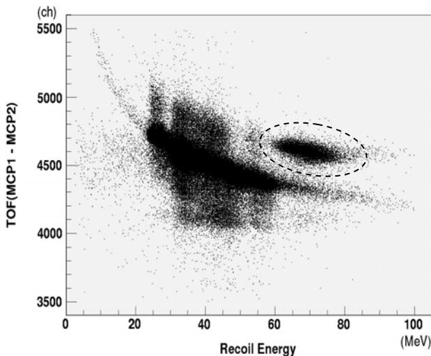
Fig. 1 Two dimensional spectrum of the energy versus TOF obtained from the  $^{82}\text{Kr} + ^{130}\text{Te}$  reaction. The unit of X and Y axis are MeV and ch, respectively. The region of dashed line is the part of ER's.
