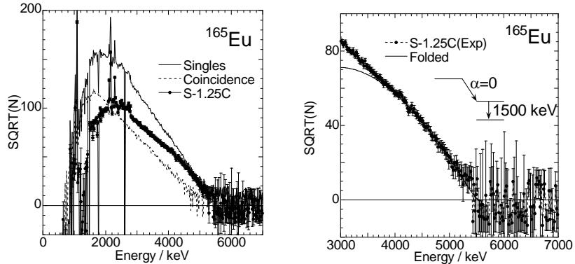
Fig. 1 Typical spectra (Singles, Coincidence with BGO and total absorption (S-1.25C))(left) and the analyzing results by folding methods (right) for  $^{165}\text{Eu}$ .
