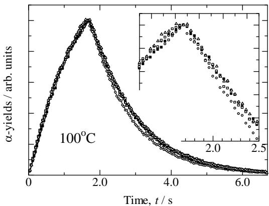
Fig. 1 Time spectra of the  $\alpha$ -particle yields for  $\text{La}_{2/3-x}\text{Li}_{3x}\text{TiO}_3$  measured at 100°C. ○:  $x = 0.067$ , □:  $x = 0.117$ , ■:  $x = 0.117$  (quenched), and △:  $x = 0.167$ .
