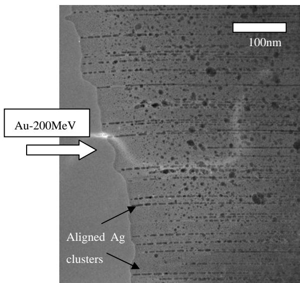
Fig. 1 A photo of cross-section TEM of Au-irradiated Ag-LTA zeolite. Ag clusters are aligned along ion tracks.
