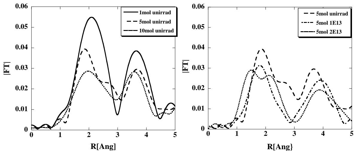
Fig. 2 Dependence of FT spectrum on the amount of  $\text{Gd}_2\text{O}_3$  for unirradiated specimens.
