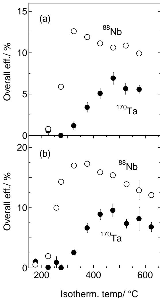
Fig. 1 Overall efficiencies observed for <sup>88</sup>Nb (○) and <sup>170</sup>Ta (●) with 200 ml min N<sub>2</sub> saturated SOCl<sub>2</sub> vapor with (a) 5% and (b) 2% of oxygen concentration as reactive gas are shown as a function of the isothermal column temprature.
