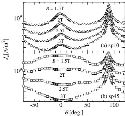
Fig. 1 Angular dependence of  $J_c$  at 77.3 K and 1 T for (a) sp10 and (b) sp45.
