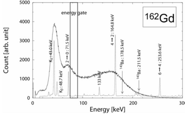
Fig. 1 Energy spectra for  $^{162}\text{Gd}$ .  $\gamma$ -ray spectrum measured with the Ge detector (dashed line), and  $\gamma$ -ray spectrum measured with the  $\text{BaF}_2$  detector (solid line) in coincidence with TAC signals.
