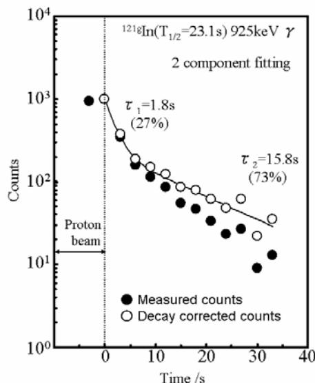
Fig. 2 Release time distributions of  $^{121}\text{In}$  at the target temperature of 1950 °C
