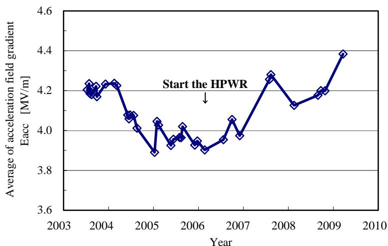
Fig. 1 The average acceleration field gradient  $E_{acc}$  across the superconducting booster changed in the years between 2003 and 2010.
