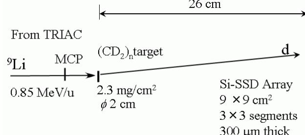
Fig. 2 Experimental setup for  ${}^9\text{Li} + d$  reactions.
