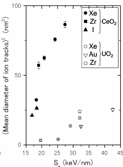
Fig. 3 The square of the mean diameter of ion tracks in  $\text{UO}_2$  and  $\text{CeO}_2$  at room temperature as a function of electronic stopping power ( $S_e$ ).
