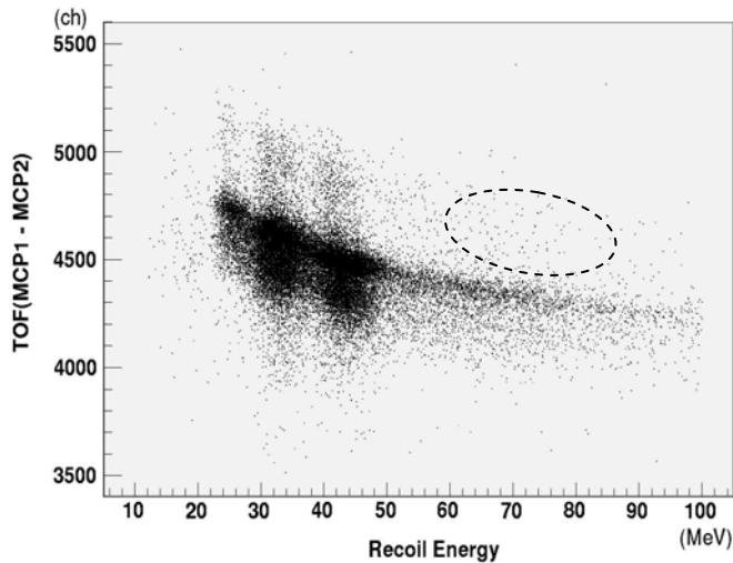
Fig. 2 Two dimensional spectrum of the energy versus TOF obtained from the  $^{82}\text{Kr} + ^{138}\text{Ba}$  reaction. The unit of X and Y axis are MeV and ch, respectively. The dashed line shows the expected area of ER's.
