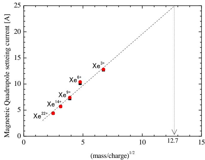
Fig. 2 The relation between a mass to charge ratio of Xe ions and magnetizing current of MQ 03-1.
