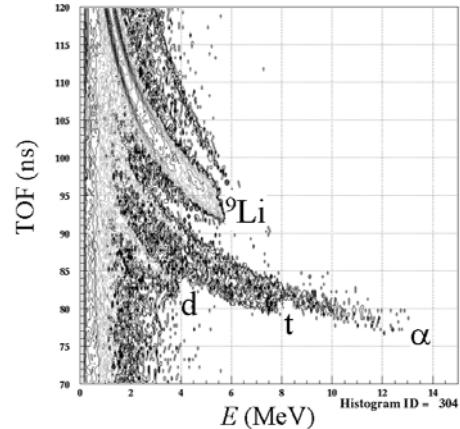
Fig. 3  $E$ -TOF spectrum for recoil particles.
