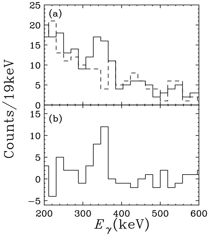
Fig. 1 (a)  $\gamma$  ray energy spectra coincident with SSD (solid line) and accidentally coincident with SSD (dashed line). (b)  $\gamma$  ray energy spectrum obtained by subtracting the accidental  $\gamma$  rays.
