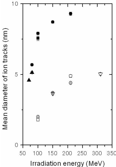
Fig. 2 Mean diameter of ion tracks in  $\text{UO}_2$  and  $\text{CeO}_2$  at room temperature as a function of irradiation energy (MeV).
