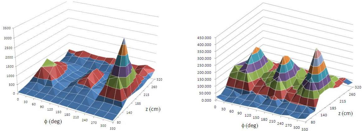
Fig. 2 (Left) Distribution of residual activities of  $^{111}\text{In}$  in the plasma chamber as a function of azimuthal angle ( $\phi$ ) and longitudinal position ( $z$ ). Residual activities of  $^{140}\text{Xe}$  (Right). See the text for details.
