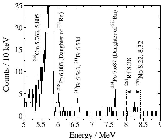
Fig. 1  $\alpha$ -spectrum accumulated from the 283 cycles of the Rf experiments with 0.15 M  $\text{H}_2\text{SO}_4/\text{HNO}_3$ .
