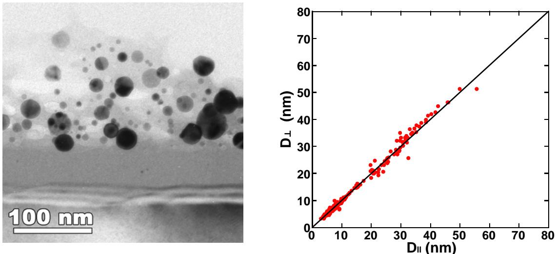
Fig. 1 Bright-field cross section view of thin film specimen before ion irradiation (a), illustrating Au nanoparticles in SiO<sub>2</sub> matrix. Size distribution of Au nanoparticles as functions of diameters measured parallel and perpendicular to the direction to film thickness (b).
