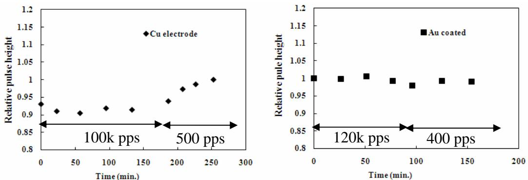
Fig. 1 Pulse-height shifts under the  $^{12}\text{C}$  beam injection rate from 400 pps to  $10^5$  pps using THGEM #3 (left panel) and THGEM #4 (right panel). The horizontal axis indicates time from the beginning of the beam injection.
