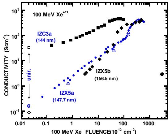
Fig. 1 Conductivity of IZO films vs 100 MeV  $\text{Xe}^{+11}$  ion fluence for three samples with thickness given in the parenthesis. Open symbols ( $\circ$ ,  $\diamond$ ,  $\square$ ) indicate the conductivity of unirradiated films. Open triangles ( $\triangle$ ) mean conductivity decrease during the ion beam break for Hall measurements in air (sample-IZX5a).
