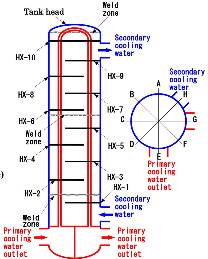
Figure 4 Thickness measured parts of the main body
