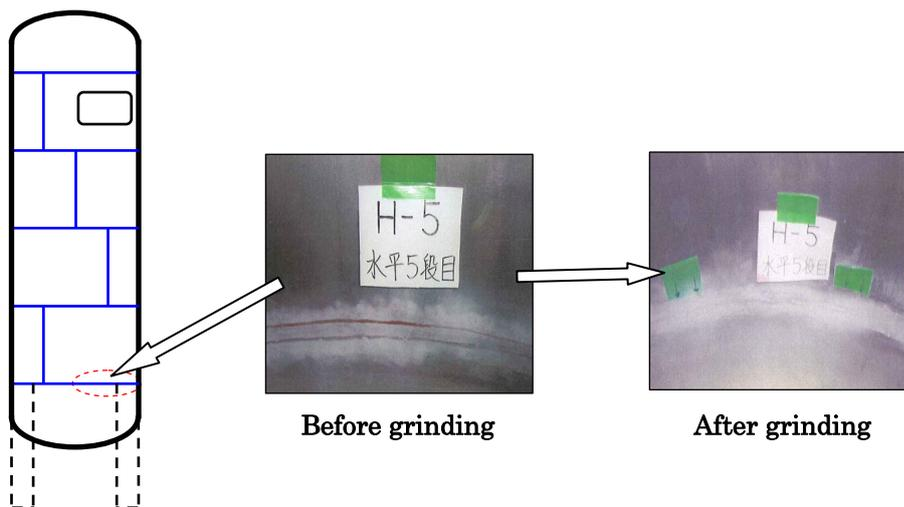
Figure 7 Sample of investigation results for the degas tank
