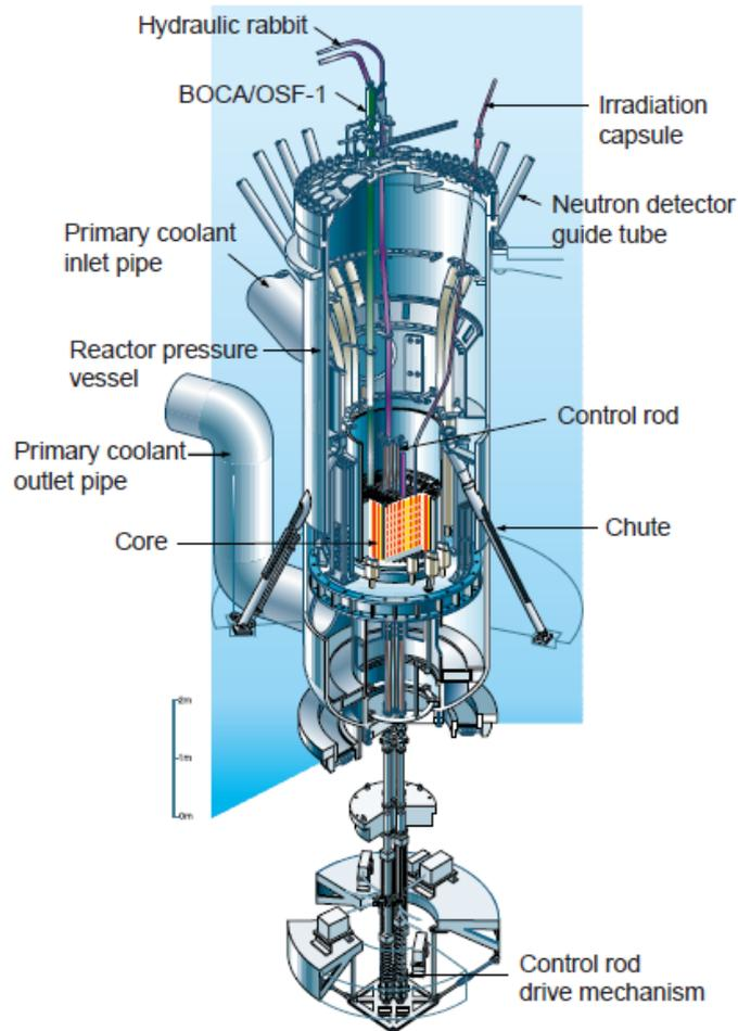
Figure 1 Cutaway view of Reactor core with pressure vessel
