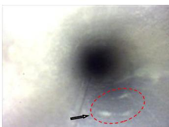
No.3 Inlet side strait pipe pitting corrosion
