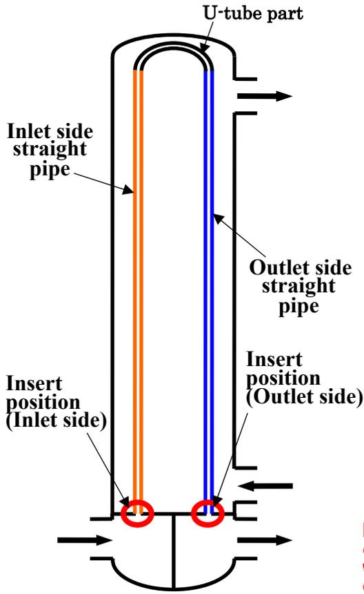
Figure 3 Inspected parts in Eddy current testing
