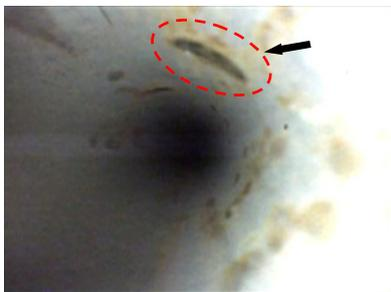
(a) No.1 Corrosion color change in outlet side straight pipe
