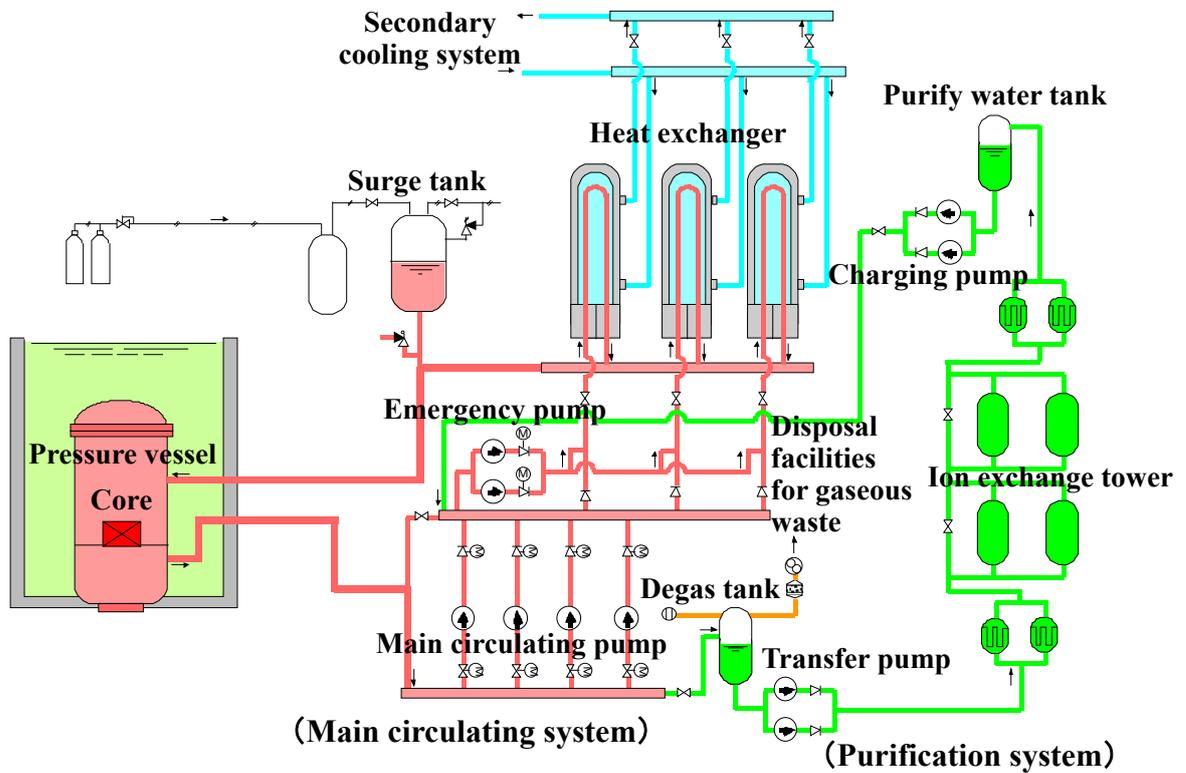
Figure 2 Diagram of the primary cooling system
