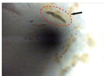
No.1 Outlet side strait pipe corrosion, color change
