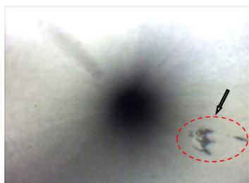
No.2 Outlet side strait pipe separation of oxide film
