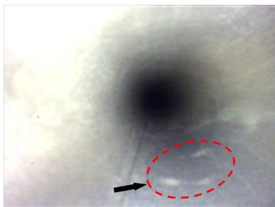
(b) No.3 Pitting corrosion in inlet side straight pipe
