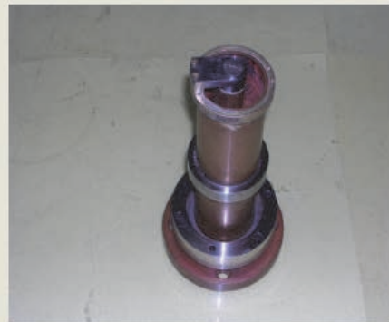
First RF window prototype after vacuum brazing
