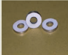
Alumina tubes metallized in BARC
