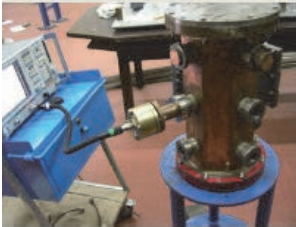
Coaxial coupler connected to RFQ cavity
