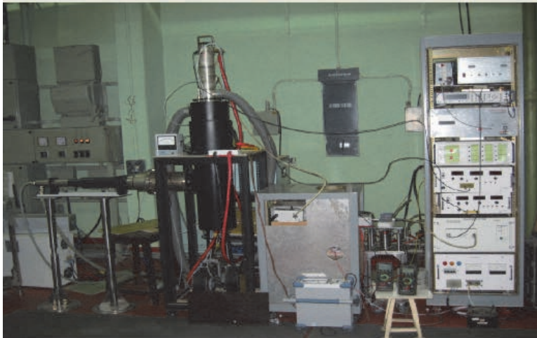
RF System for 400 keV prototype RFQ (35 kW tetrode-tube based RF power supply using 1 kW intermediate driver).
