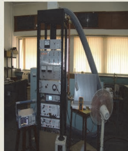
New Driver stage : 350 MHz, 2.5 kW
