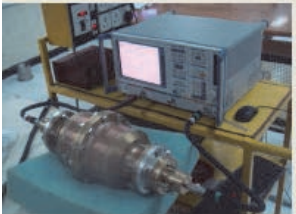
Coaxial adapters under RF Characterization
