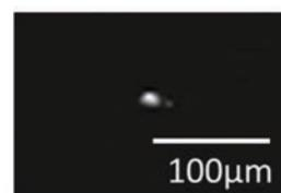
Fig. 2 NFP of the MZ waveguide ( $\lambda=1.55\ \mu\text{m}$ ).
