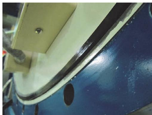
Fig. 2 Rectangular type gasket for the tandem.
