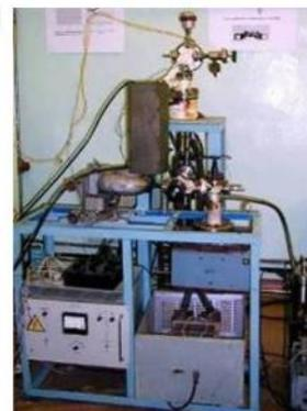
NL : Pump HBP-5 DM, NS : Pump NORD-100, NS2 : Magnet-discharge pump NORD-250, BL : Nitrogen trap, PT : Thermocouple vacuum meter, PA : Ionization vacuum meter, CV : Work chamber, V : Vacuum valve, S<sub>1</sub> : Omegatron-type sensor of the PMO-13 mass spectrometer EPDO-2, S<sub>2</sub> : Quadruple mass spectrometer RGA-100
