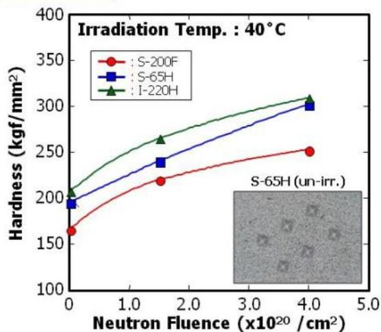
Hardness of irradiated Be was increased with increasing the neutron fluence.
