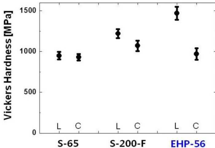
Hot extrusion : anisotropy in microhardness
