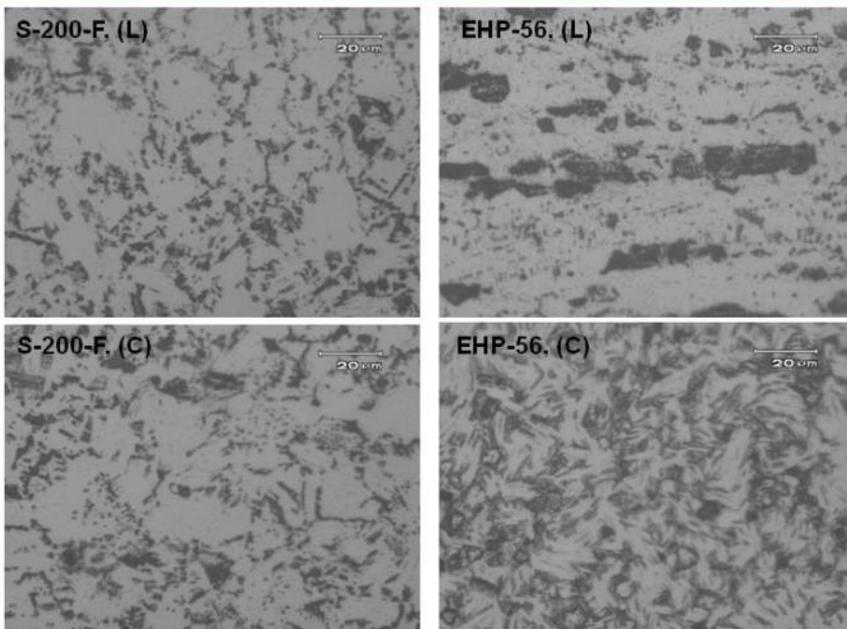
**Small grains but lower hardness in EHP-56, (c) ←  $\langle 10\bar{1}0 \rangle$  texture**
