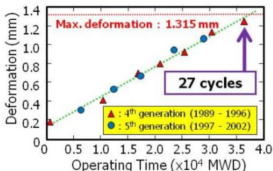
Deformation increased with increasing operation time for accumulation of helium.
