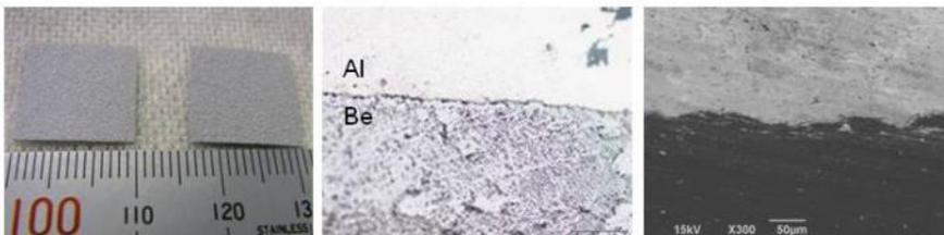
Aspect after spraying      Cross section (Left: Microscope, Right: SEM, BEI)
