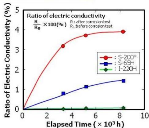
The electric conductivity change of S-200F was larger than that of I-220H.
