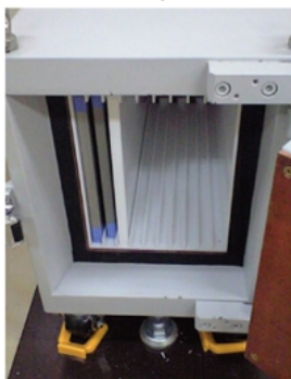
Shielding box made by thick lead
