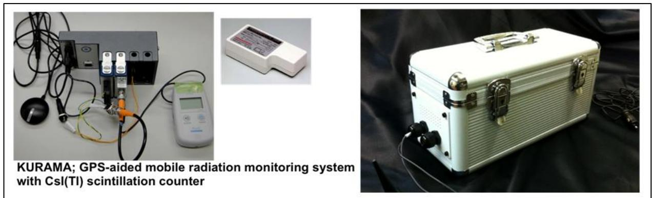
Figure 2-6 Example of mobile gamma radiation monitoring system
