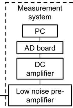
So, it is important to suppress the electrical noise to signal path between signal source and the pre-amplifier.
