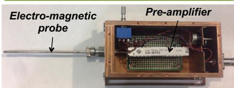
Electrical wirings can be shorter and the pre-amplifier can be covered by a metal shielding case resulting in better S/N ratio.
