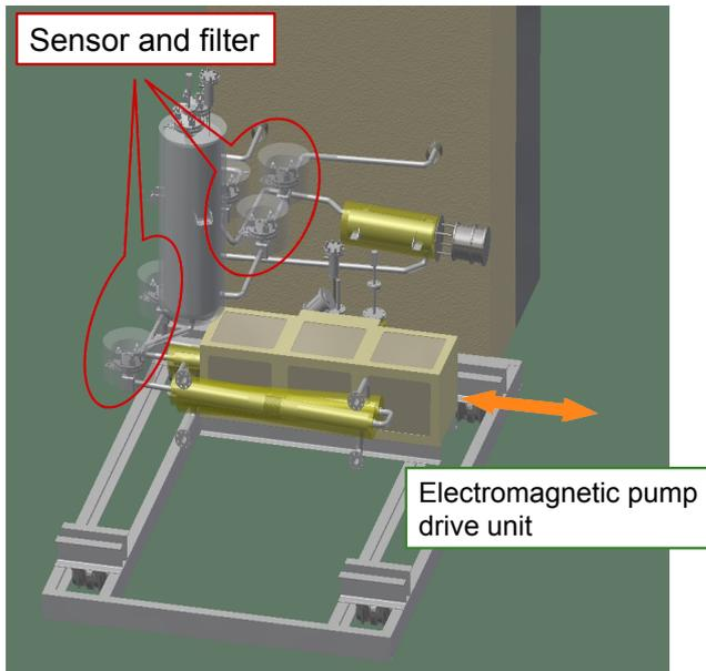
It pulled out an electromagnetic pump drive unit.
