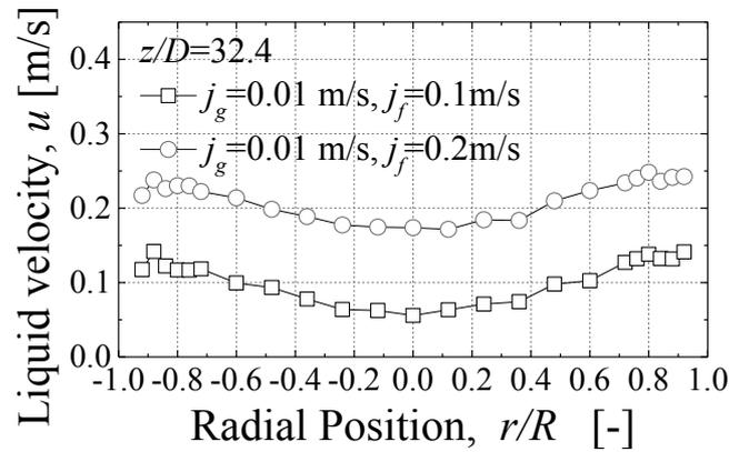
Fig.1 Local liquid velocity profiles.
