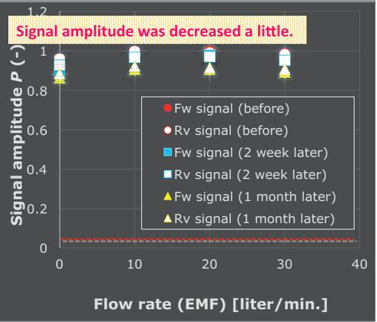
Plug-in type of Ultrasonic flowmeter can apply to re-wetted condition.
