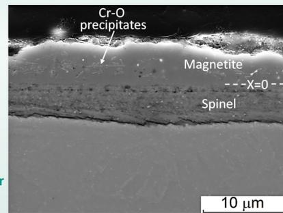
T91-B after exposure for 2015 h with intermittent increase in  $c_o$  after ~1200 h
