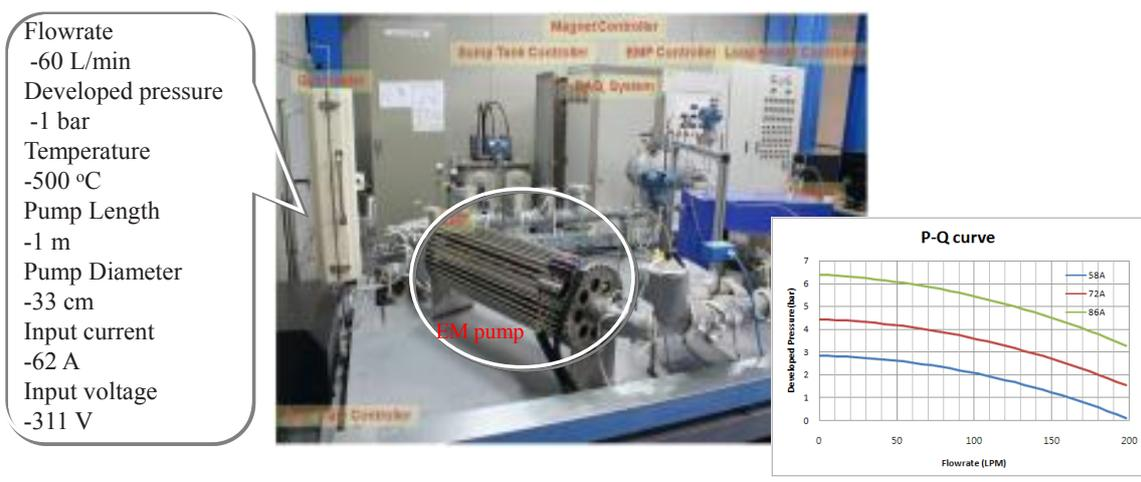
◆ The EM pump for the experiment of the liquid **PbBi** flow
