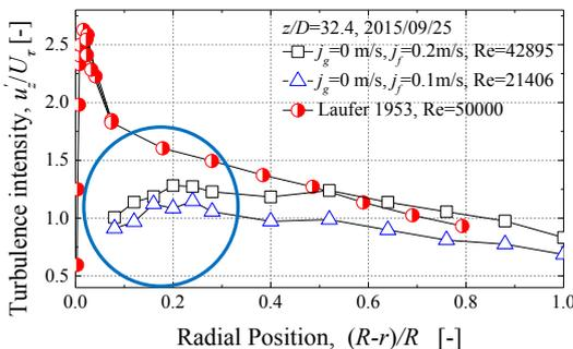
Due to this comparison, it is found that **the measured turbulence intensity decreases at further area from the wall surface.**
