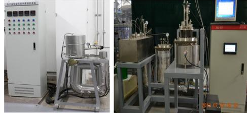
Thermal convention corrosion loop
