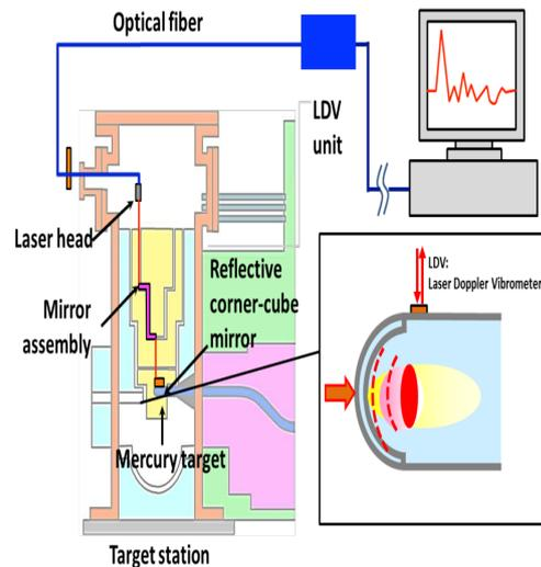
LDV system installed @ JSNS Hg target
