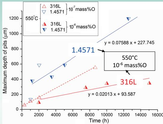
Maximum depth of pit-type corrosion attack on austenitic steels tested in flowing LBE (~ 2 m/s) depending on temperature and oxygen concentration in the melt.
