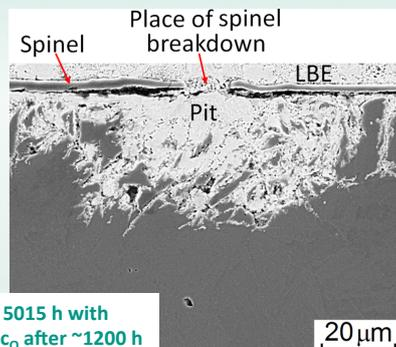
T91-A after exposure for 5015 h with intermittent increase in  $c_o$  after ~1200 h
