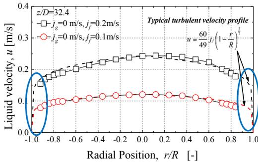
Measured velocity profiles seem to show good agreement with typical turbulent velocity profile.
