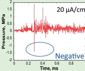
**Time response of pressure in LBE @ the center of beam window**
