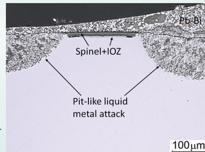
T91-A after exposure for 1007 h with temporary increase in  $c_o$  after ~450 h
