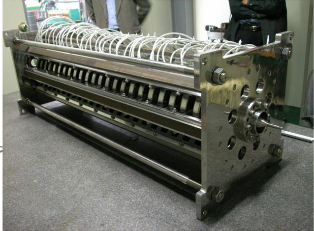
◆ The EM pump for the corrosion test of the material in the **sodium** environment
