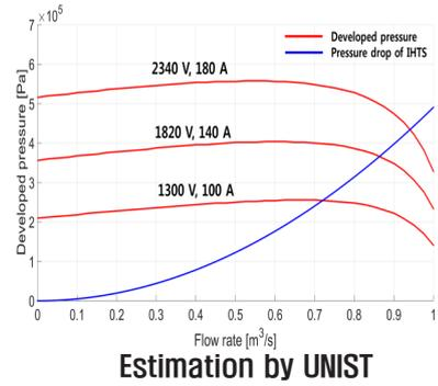
◆ The DC pump for test of the reaction between sodium and CO<sub>2</sub>
