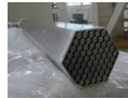
Full-scale simulated FA for flow experiments (61 pins/ wire wrapped)
