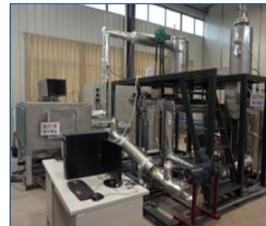
Pre-research loop for measurement and control of liquid metal
