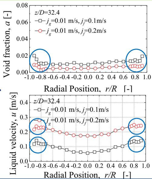
In case of poor wettability condition, many bubbles tend to be trapped in the wall region. **Then, void fraction becomes high near the wall and the liquid phase is accelerated by the gas phase flowing along the wall.**
