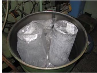
Fig. 5 Vacuum-cast Be ingots
