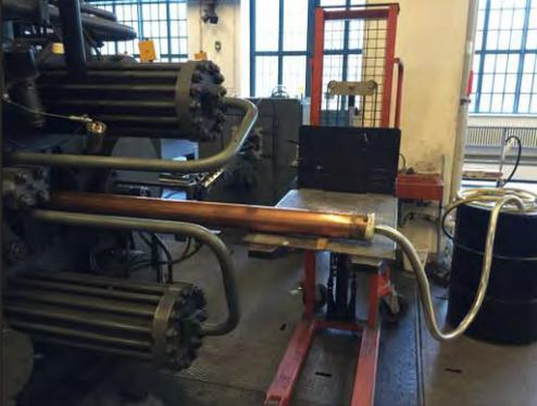
During the hot extrusion process the sample can brake. Therefore a special equipment was build. We have called it Catcher. It is a tube that is connected to the mouth of the press.
