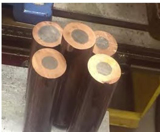
Fig. 1 Encapsulated Be-Ti rods after their cutting by disc saw
