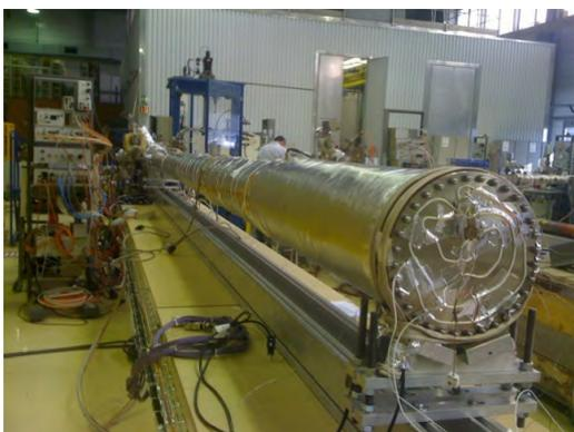
Figure 2: Vacuum Test for LHCb Beryllium Chamber
