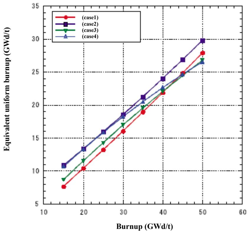
**Fig. 3.9** Equivalent uniform burnup in a transportation package system for PWR SF
