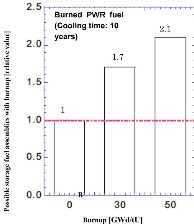
**Fig. 2.2** Variation in the possible storage amount of fuel assemblies with burnup (PWR  $17 \times 17$ , initial enrichment 4.7 wt%, infinite array ( $k_{inf} = 0.95$ ), ORIGEN2.1 burnup calculation, MVP criticality calculation)
