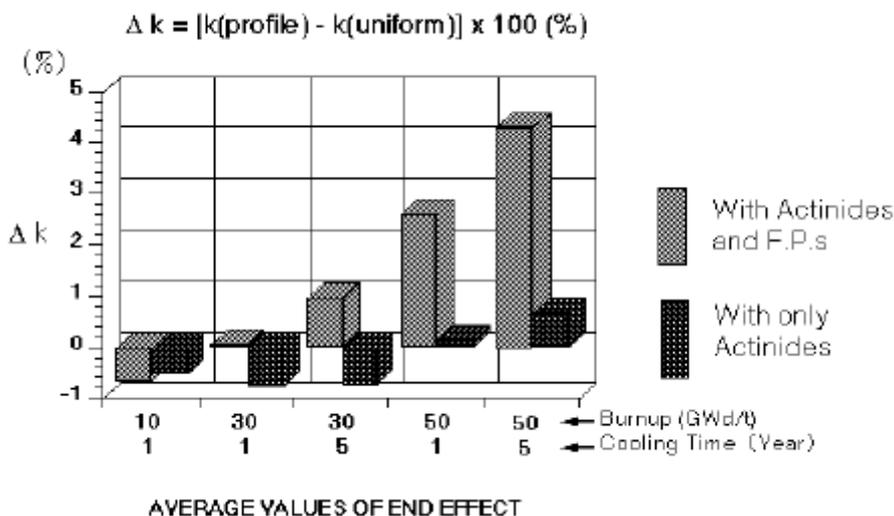
**Fig. 4.2** Effect of axial burnup distribution (End effect of infinite array system with a single pin cell) [66]
