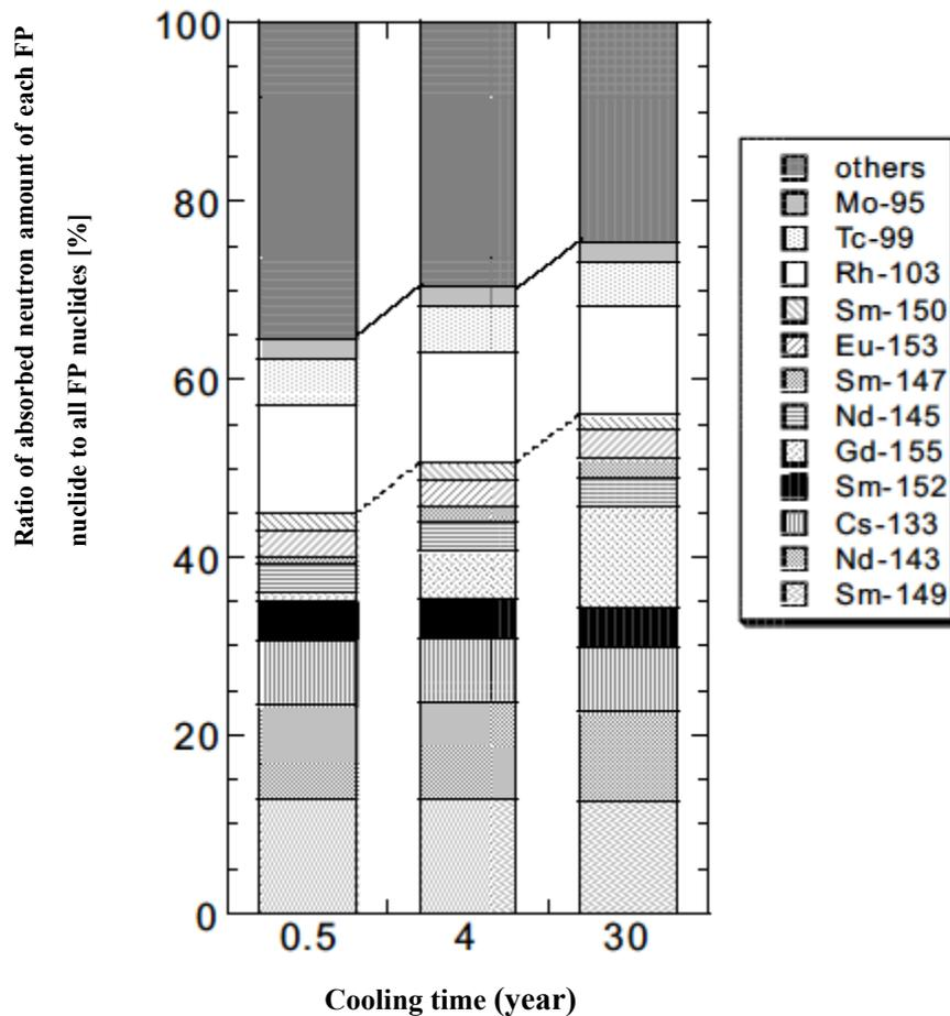
**Fig. 4.1** Ratio of a number of absorbed neutrons for each FP nuclide to that of all FP nuclides (contributions of the 12 nuclides are on the continuous line, and those of the 9 nuclides excluding <sup>103</sup>Rh, <sup>99</sup>Tc, and <sup>95</sup>Mo are on the dotted line)
