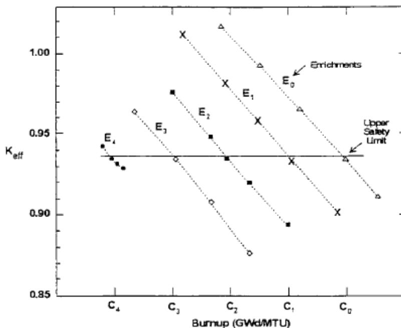
Fig. 5.2 Setup method for the initial enrichment reference burnup [84]
