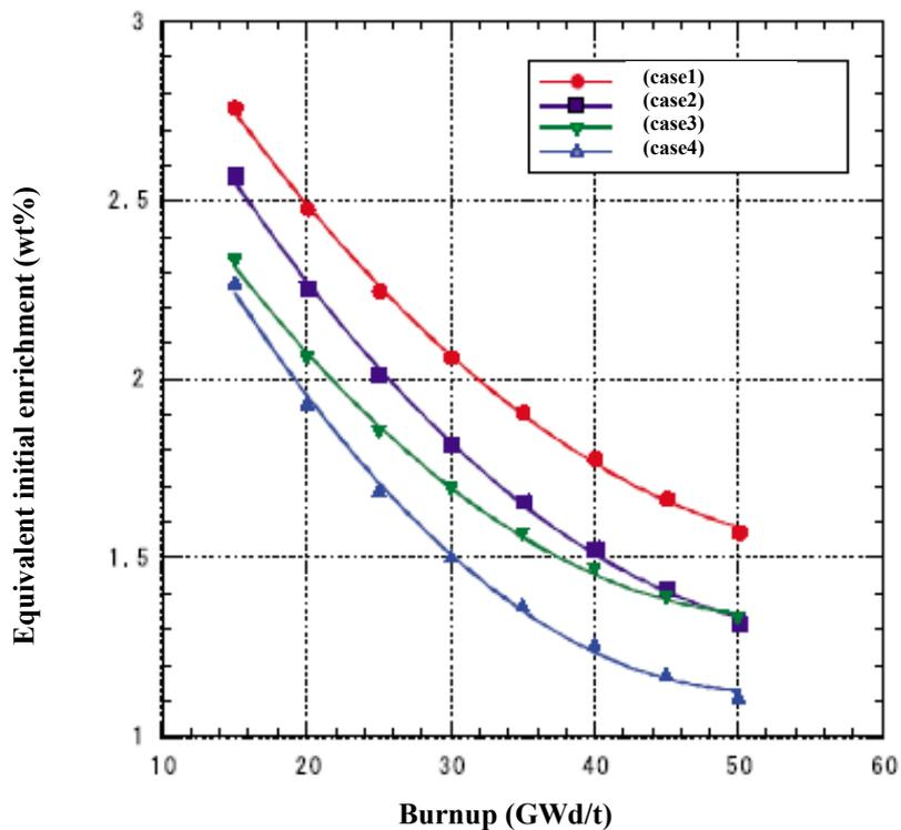
Fig. 3.10 Equivalent initial enrichment in an infinite arrangement geometry of a single-fuel pin cell
