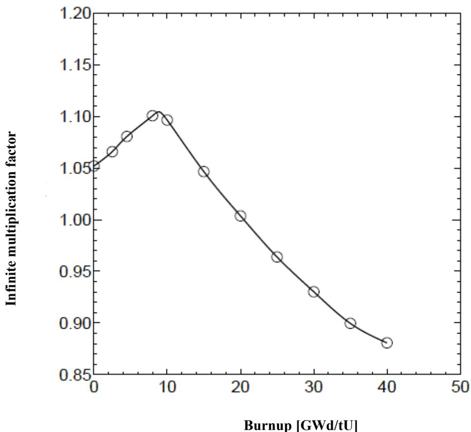
**Fig. 3.12** Variation in the infinite neutron multiplication factor for the burnup of a BWR fuel assembly containing a burnable poison (moderator void fraction: 40%)
