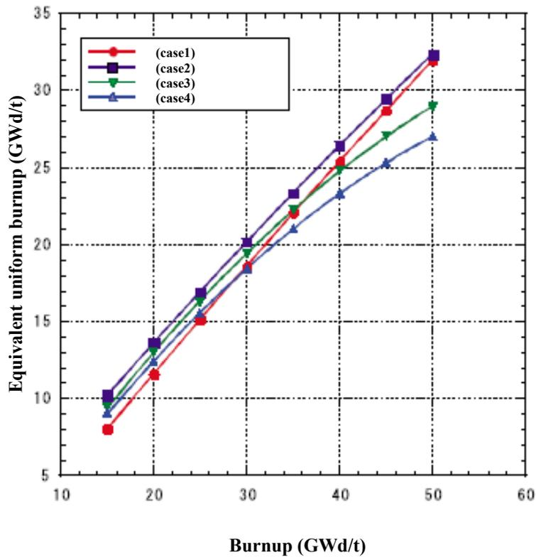
**Fig. 3.8** Equivalent uniform burnup in an infinite arrangement geometry system of a single-fuel pin cell
