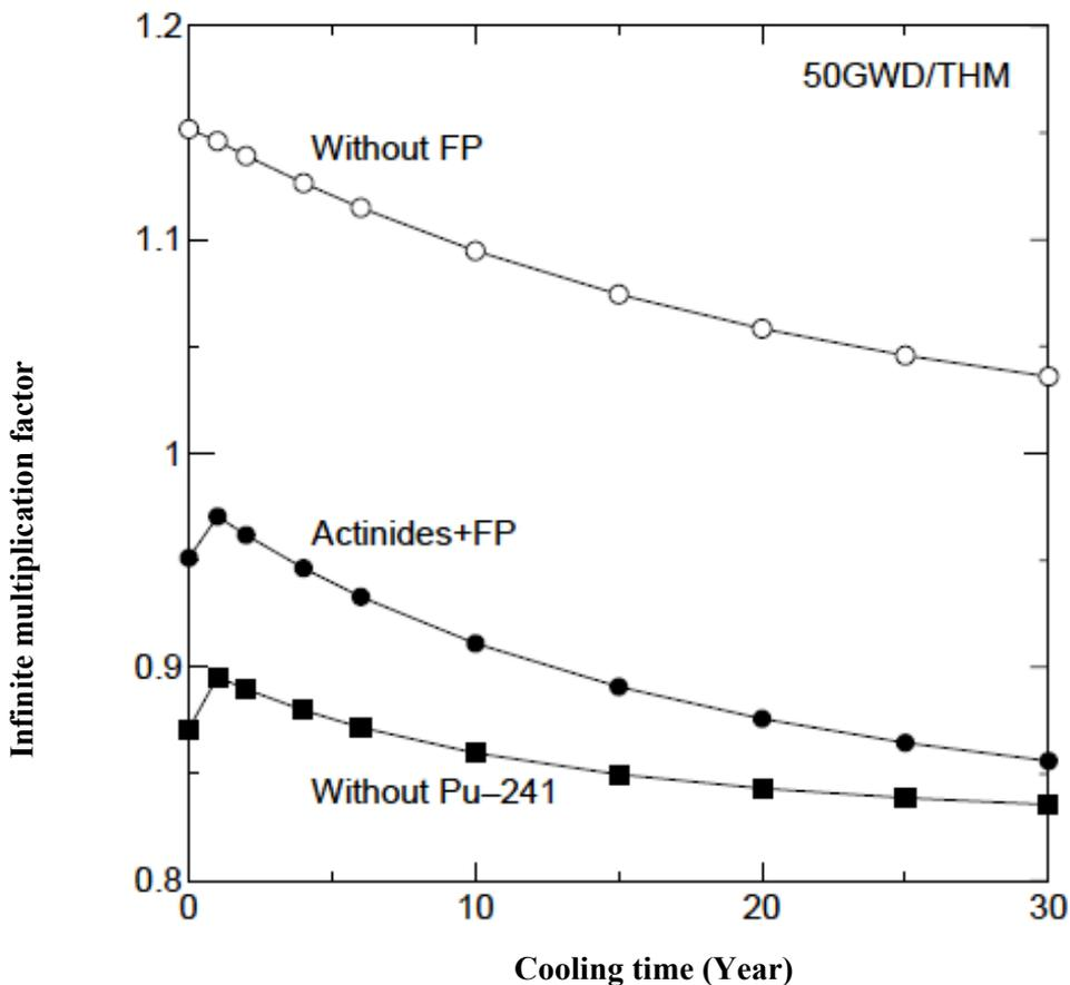
**Fig. 3.13** Variation in infinite multiplication factor with cooling time [36]
