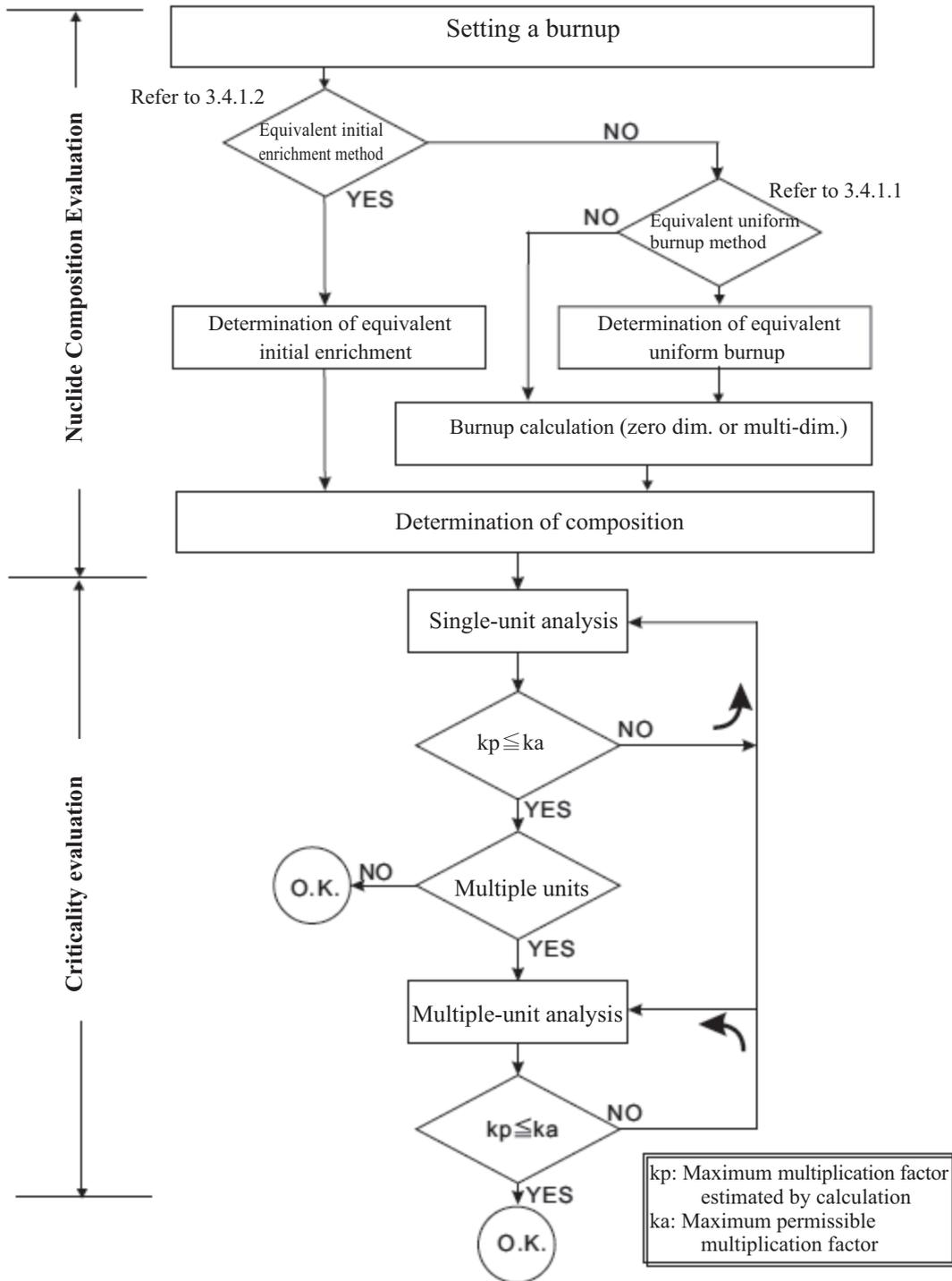
Fig. 2.3 Procedure for a criticality safety assessment applying for burnup credit
