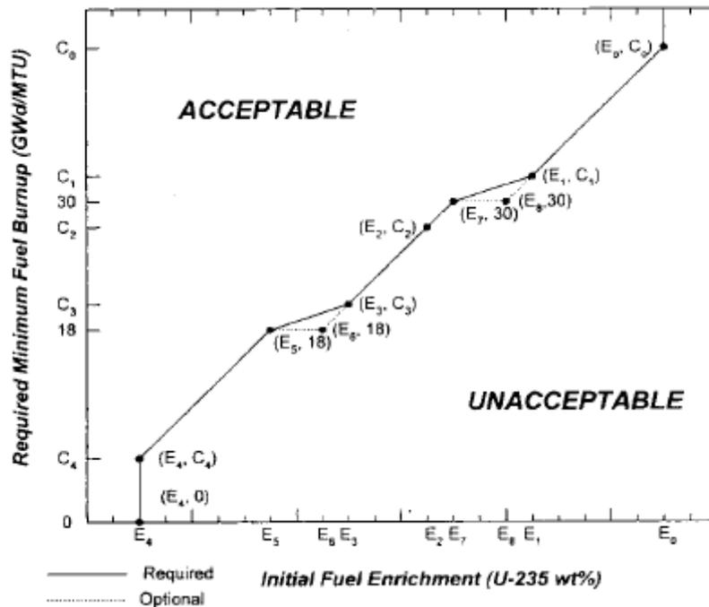
**Fig. 5.1** Spent fuel loading curve [84]
