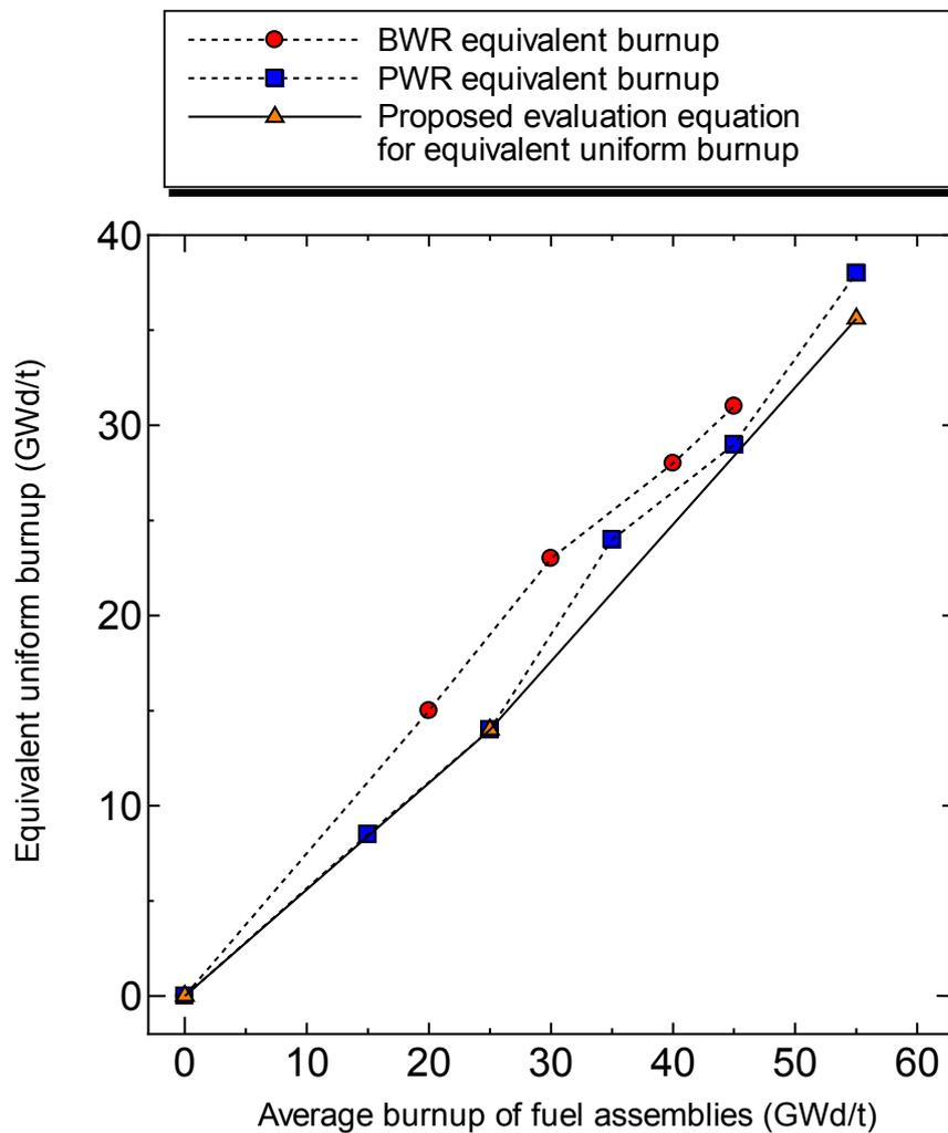
**Fig. 3.7** Equivalent uniform burnup in a dry storage cask considering the axial burnup distribution, irradiation histories, and nuclide composition calculation accuracy of ORIGEN2 (U + Pu only) [31]
