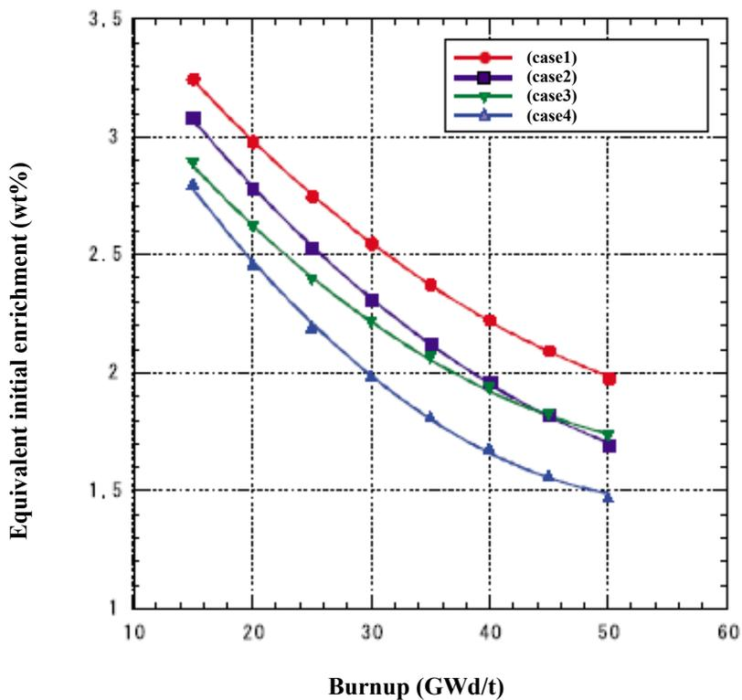
Fig. 3.11 Equivalent initial enrichment in a system of spent fuel transportation packages
