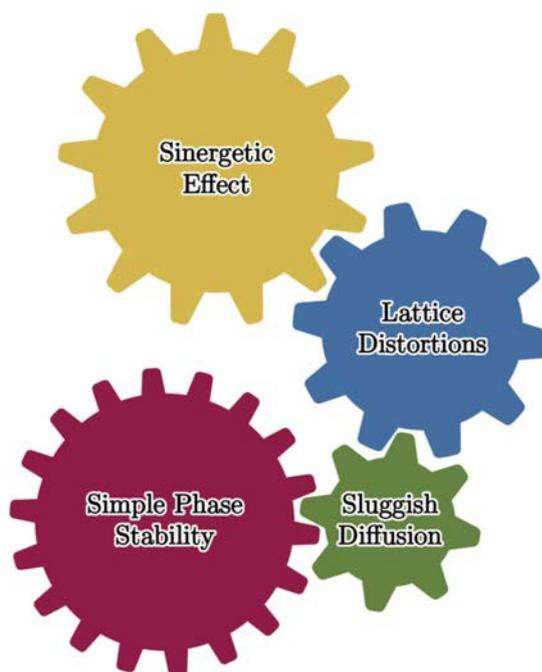
Fig. 1 Essential characteristics of high-entropy alloys [1]
