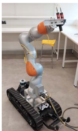
Figure 3: KUKA IIWA system integrated onto a Superdroid HD2 with a fiber-coupled Raman system.
