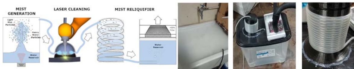
Figure 1: The mist generation and capture system utilizing centrifugal forces and bubble filtration.
