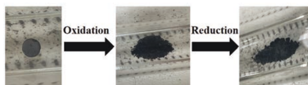
Fig.1 Photos of simulated debris U:Zr:Ca=4.5:4.5:1 1700°C (Left:before Redox Middle:after oxidation Right:after Redox)
