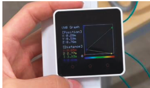
Fig.2 3D position detection using UWB.
