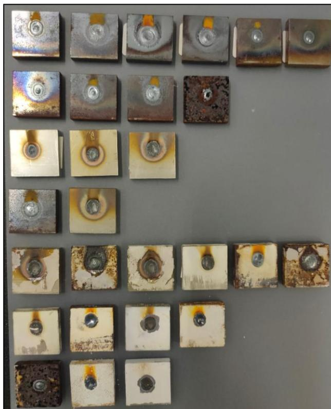
Fig. 3-4 Various laser-irradiated test specimens
