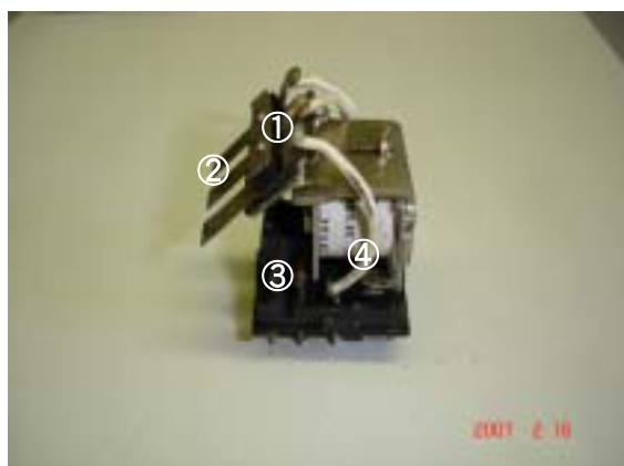
Fig. 4.1.5 Structure of the EMR (ID No. 3) without the plastic cover after the test step 8. 1. Hinge; 2. Contacts of moving side, three Ag alloy contacts of 4mm in diameter are attached on three thin Cu plates; 3. Contacts of fixed side; 4. Magnet coil.
