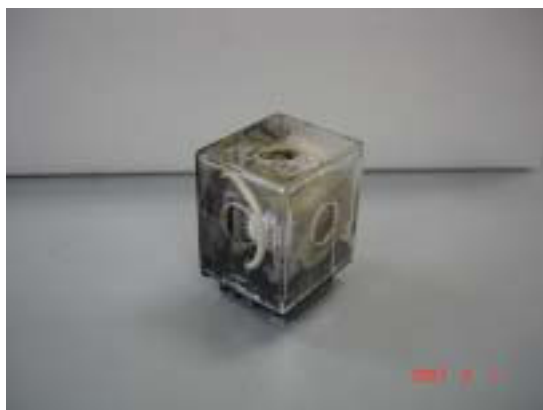
Fig. 4.1.2 Appearance of the EMR (ID No. 3) set up a plastic cover with five holes of 10mm in diameter. This EMR was used from the test step 4 to the test step 8.
