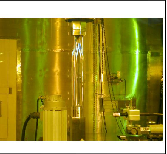
A photograph showing a nozzle-attached hexagonal tube being inserted into a larger component. The tube has a nozzle protruding from one end.                    |
