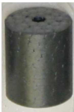
Fig. 5 Appearance of a fuel compact
