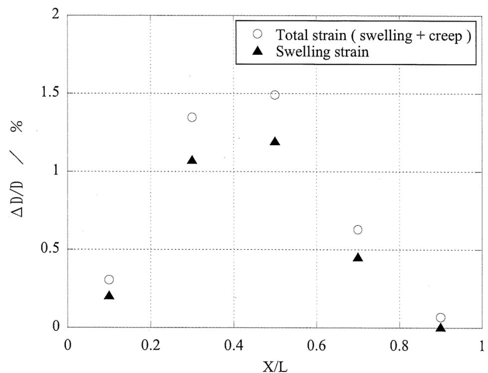
Fig.23 Cladding deformation after the irradiation
