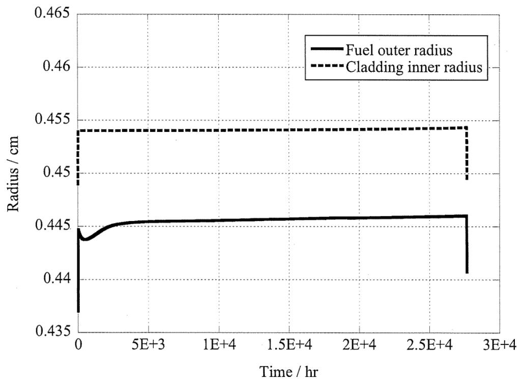
Fig.12 Deformation profiles of fuel and cladding at  $X/L=0.9$
