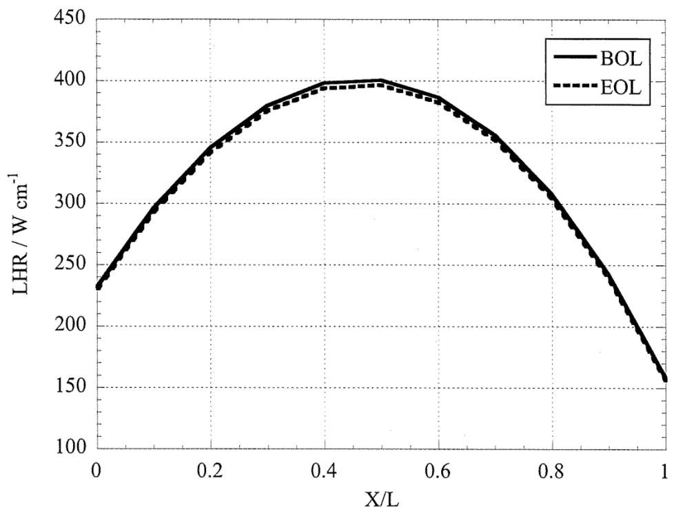
Fig.3 Axial distribution condition of LHR
