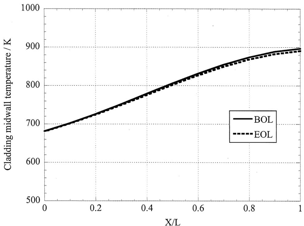
Fig.4 Axial distribution condition of cladding midwall temperature
