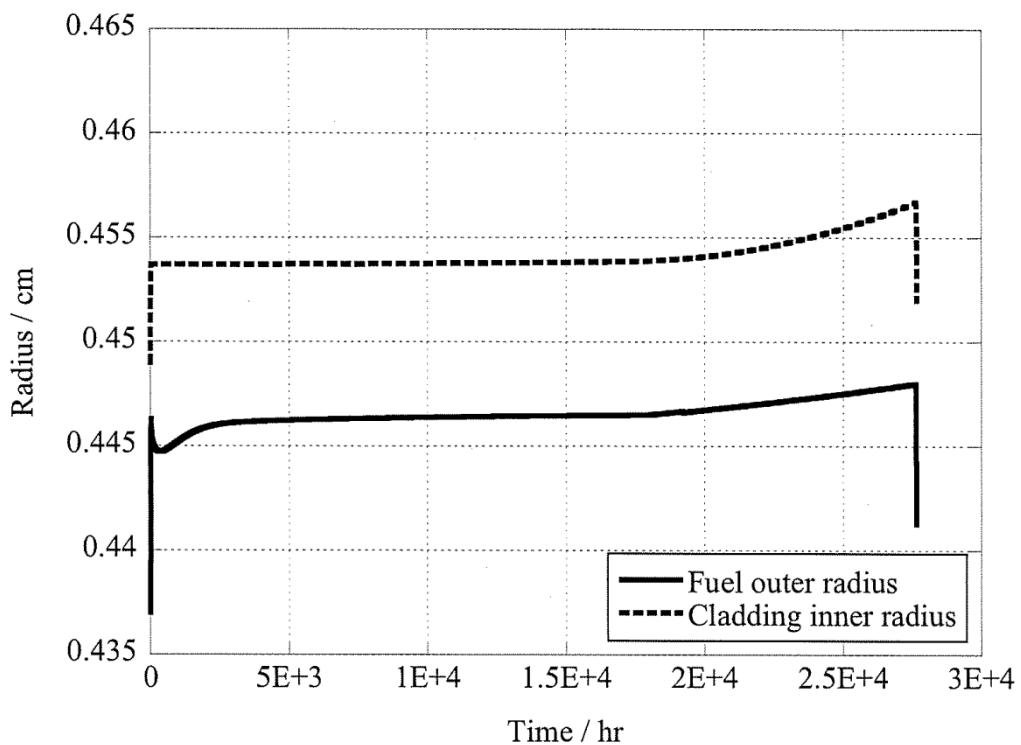
Fig.13 Deformation profiles of fuel and cladding at  $X/L=0.7$
