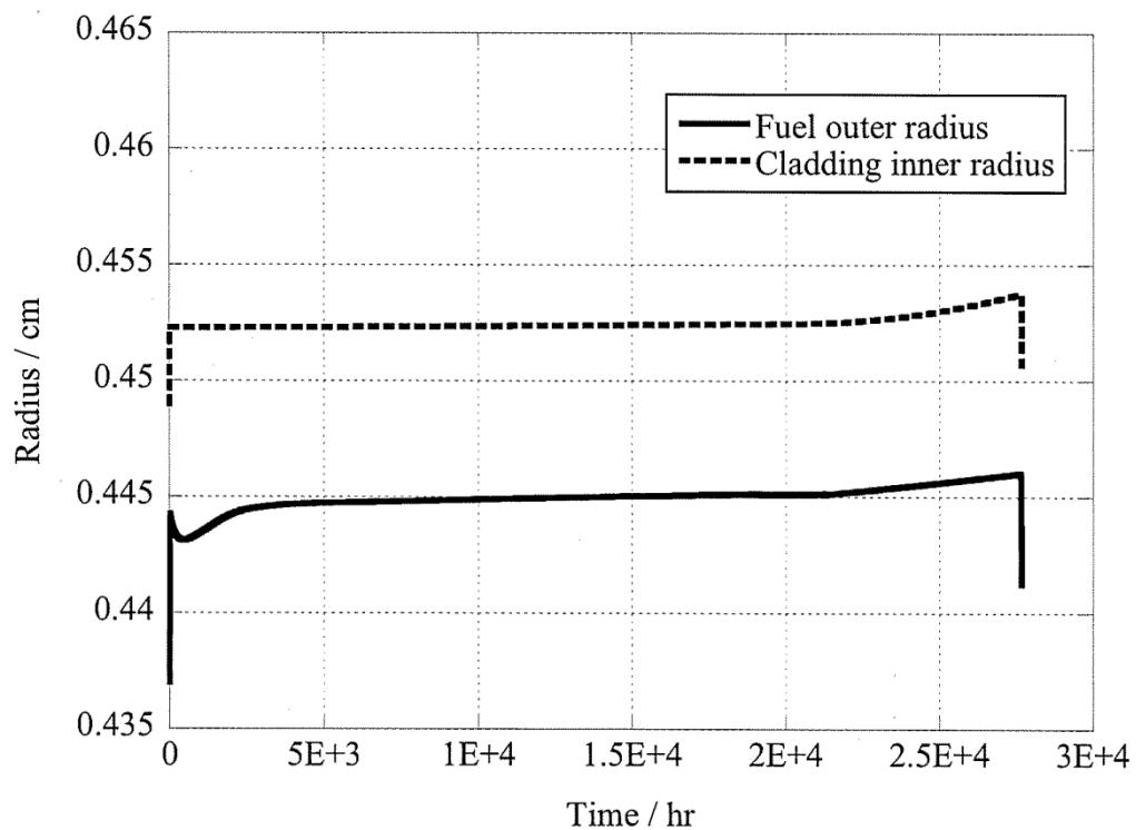
Fig.16 Deformation profiles of fuel and cladding at  $X/L=0.1$
