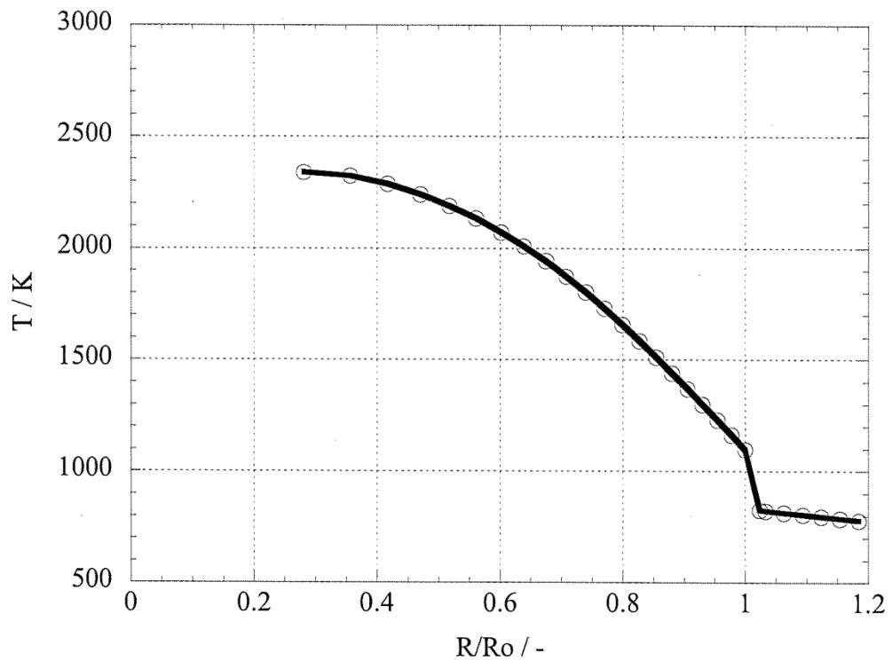
Fig.19 Radial distribution of fuel temperature at  $X/L=0.5$
