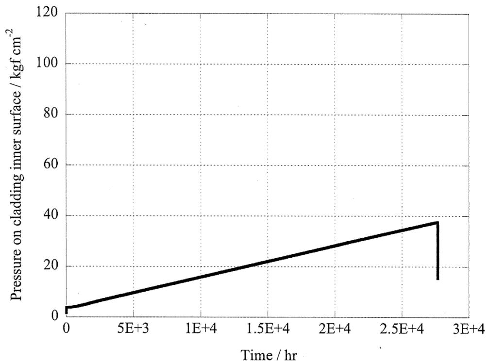
Fig.22 Profile of pressure on the cladding inner surface at  $X/L=0.5$
