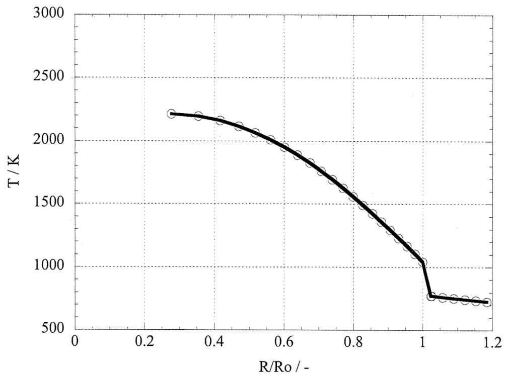
Fig.20 Radial distribution of fuel temperature at  $X/L=0.3$
