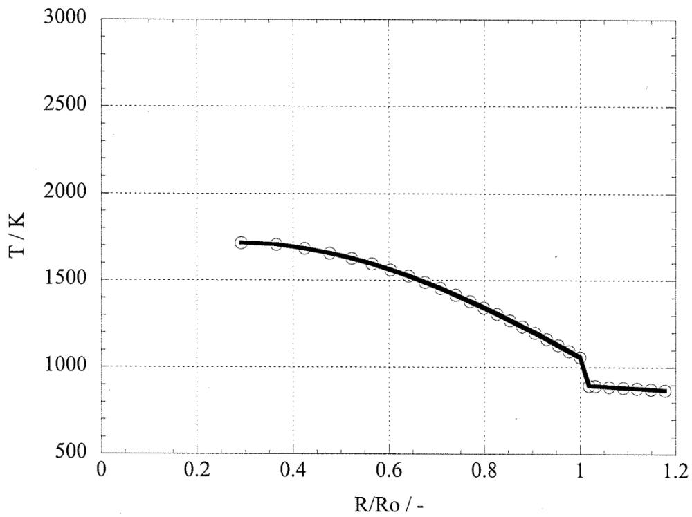
Fig.17 Radial distribution of fuel temperature at  $X/L=0.9$
