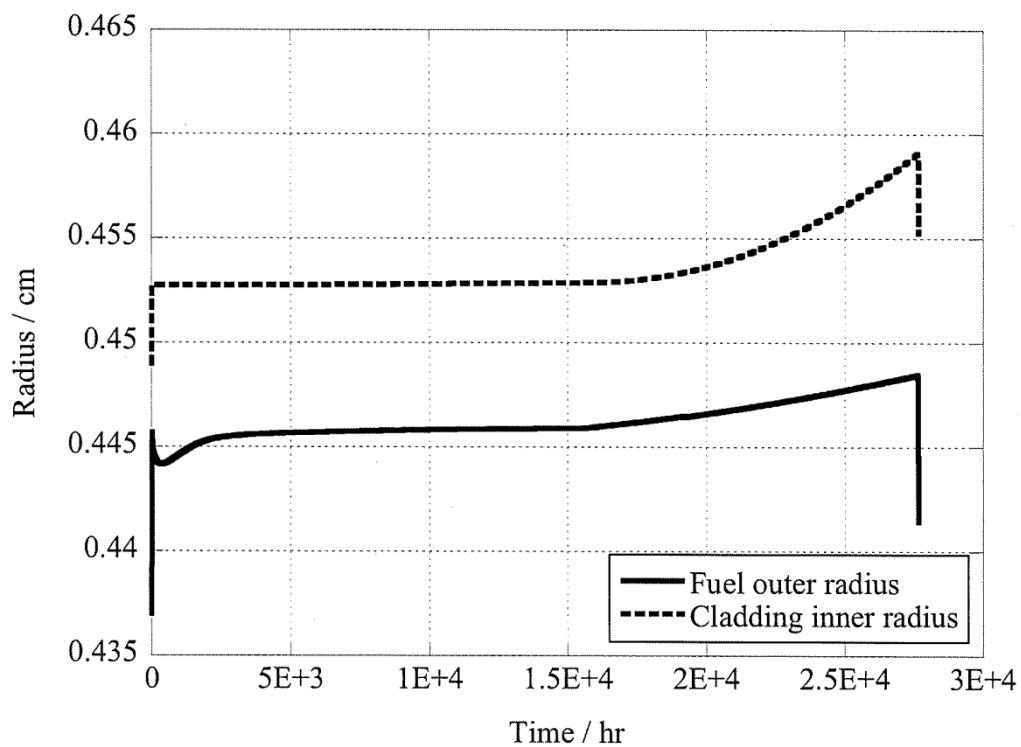
Fig.15 Deformation profiles of fuel and cladding at  $X/L=0.3$
