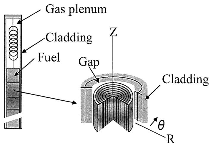
Fig.1 Geometrical model of CEDAR
