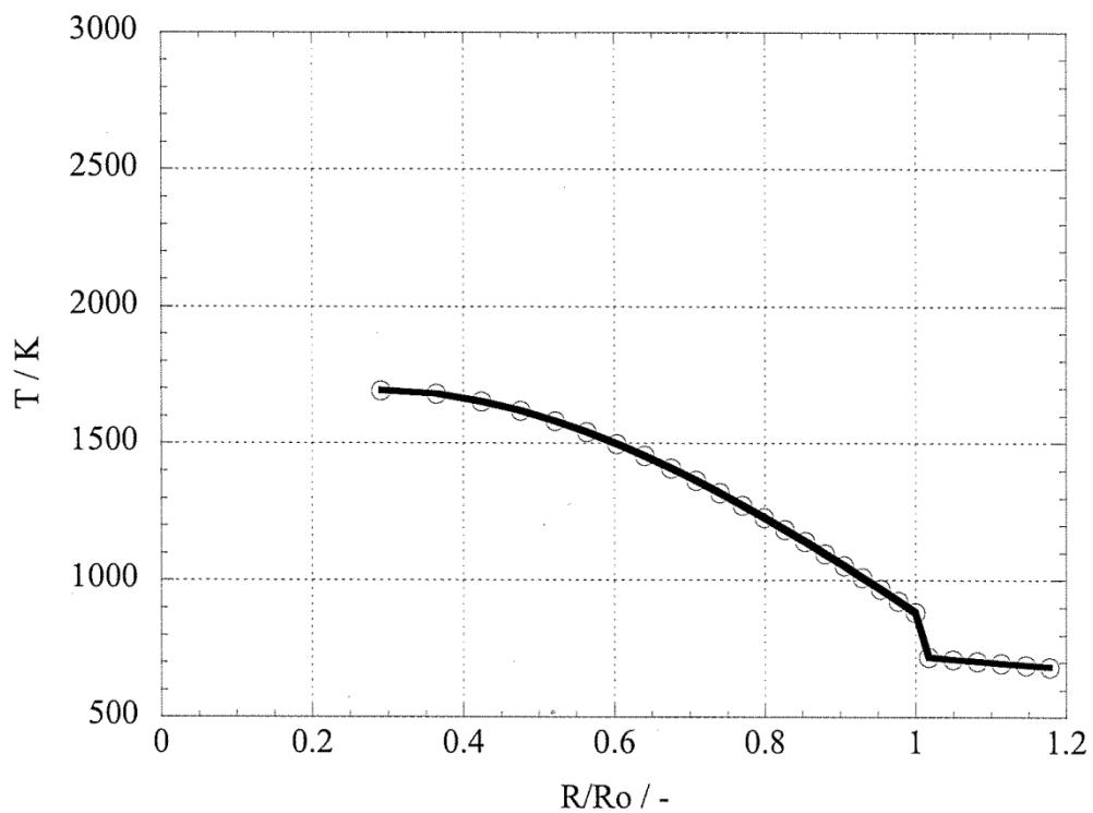
Fig.21 Radial distribution of fuel temperature at  $X/L=0.1$
