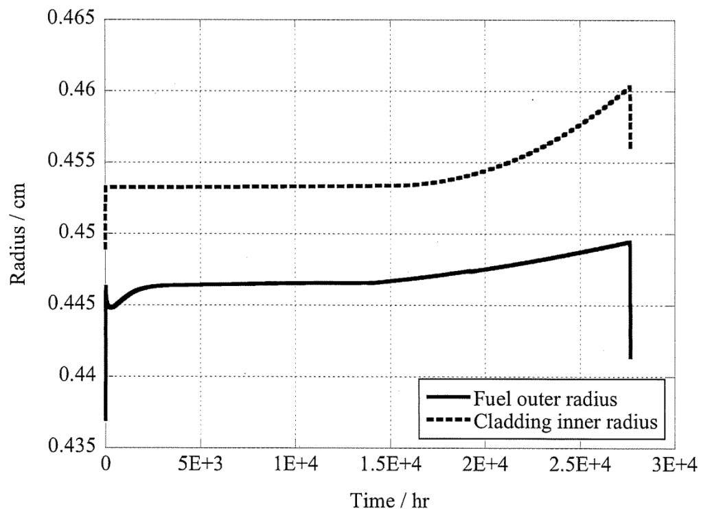
Fig.14 Deformation profiles of fuel and cladding at  $X/L=0.5$
