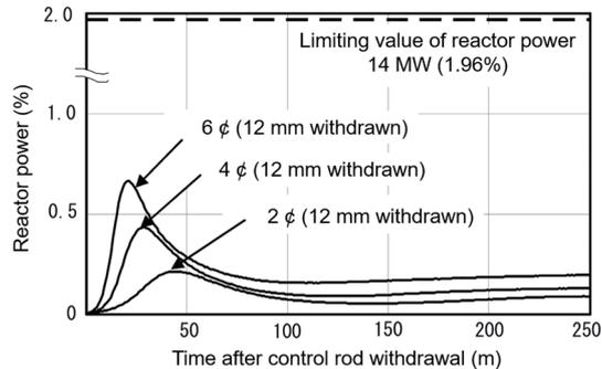
Fig.3-10 Change in reactor power after positive reactivity insertion
