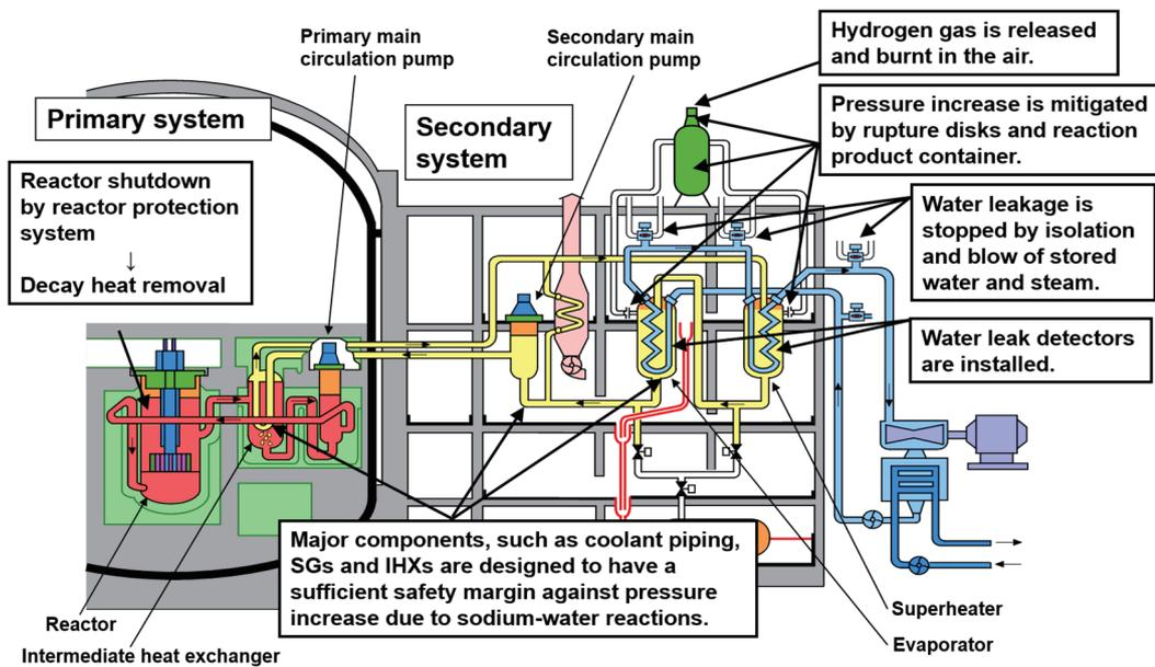
Fig.4-4 Safety assurance on sodium-water reaction
