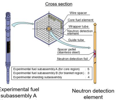
Experimental fuel subassembly A (for core region)      Neutron detection element
