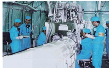
《Equipment to handle neutron detection foil》
