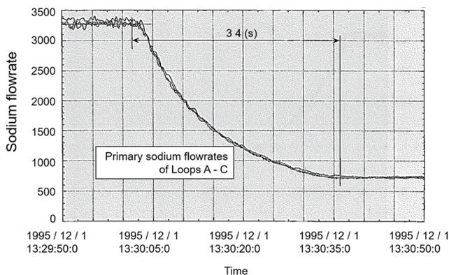
Fig.3-7 Flow coastdown characteristics of primary circulation pump
