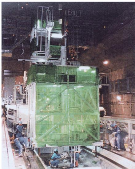
《Equipment to handle neutron detection element》
