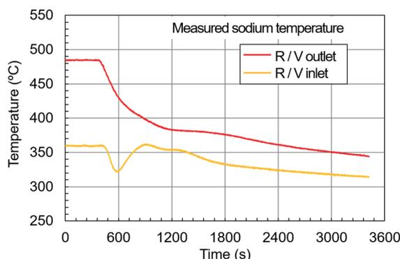
Fig.3-6 Plant trip test at 40% power operation
