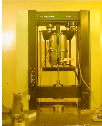
Photo 6-3 tension testing machine
