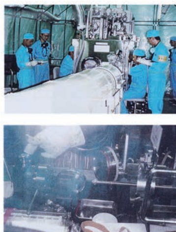
《Equipment to handle neutron detection foil》 (b) Take-out of neutron detection foil (using globe box)
