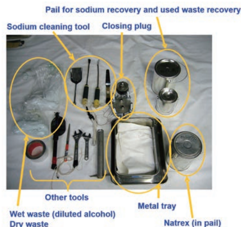
Fig.8-1 Sodium cleaning tools (physical method)
