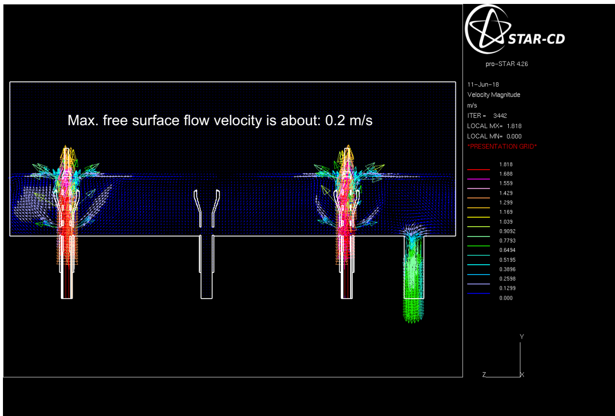
Fig. 2.4.5(a) LBE flow vector in the expansion tank (lengthwise cross section).
