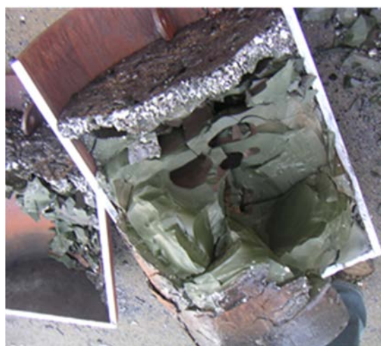
Figure A4 Top and cross-sectional views of the solidified product (G25) in disassemble processes.
